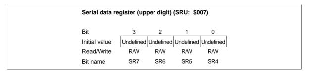
Figure 77 Serial Data Register (SRU)
