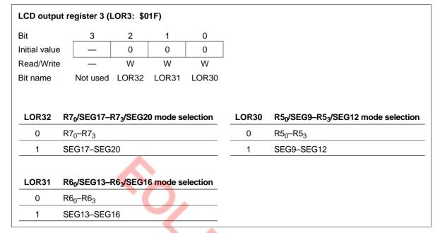
Figure 93 LCD Output Register 3 (LOR3)
