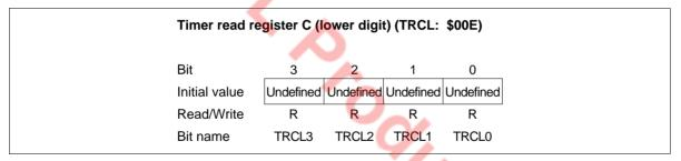
Figure 59 Timer Read Register C Lower Digit (TRCL)
