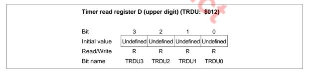
Figure 68 Timer Read Register D Upper Digit (TRDU)
