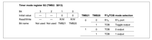
Figure 48 Timer Mode Register B2 (TMB2)
