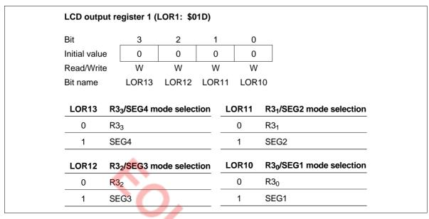
Figure 91 LCD Output Register 1 (LOR1)
