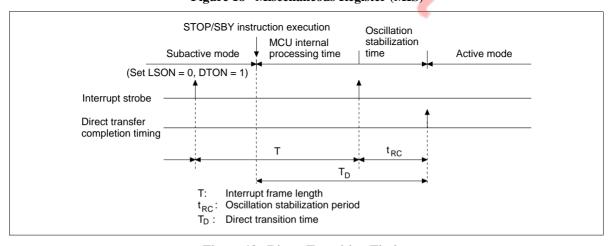
Figure 19 Direct Transition Timing
