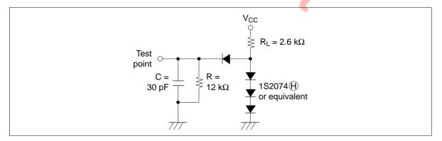
Figure 109 Timing Load Circuit
