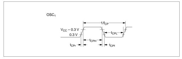
Figure 104 External Clock Timing
