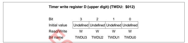
Figure 66 Timer Write Register D Upper Digit (TWDU)
