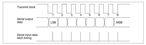
Figure 78 Serial Interface Output Timing
