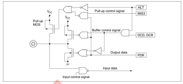
Figure 29 I/O Buffer Configuration
