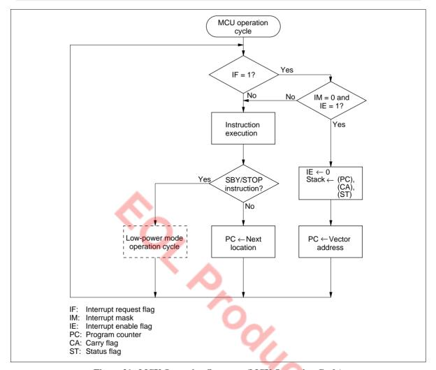
Figure 21 MCU Operating Sequence (MCU Operation Cycle)
