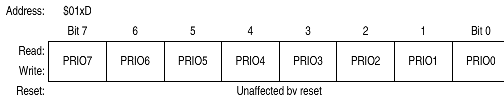
Figure 16-15. Transmit Buffer Priority Register (TBPR)
