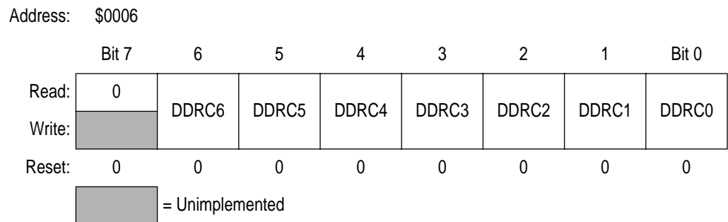
Figure 17-11. Data Direction Register C (DDRC)
