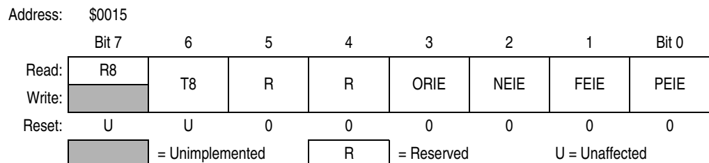
Figure 12-12. SCI Control Register 3 (SCC3)
