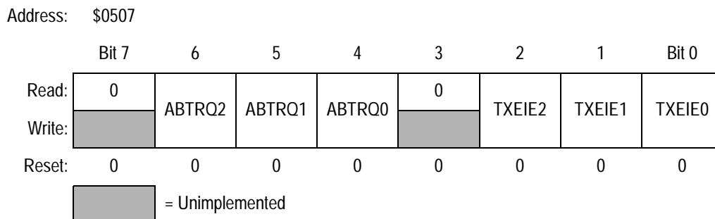
Figure 24-22. Transmitter Control Register (CTCR)
