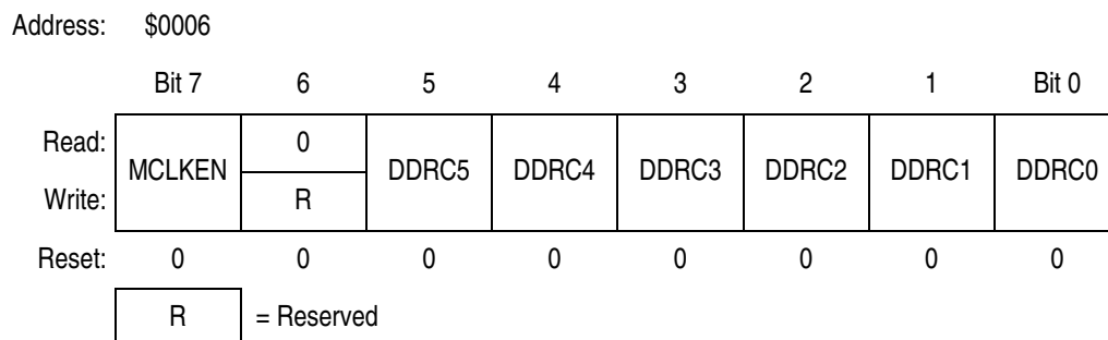
Figure 22-9. Data Direction Register C (DDRC)
