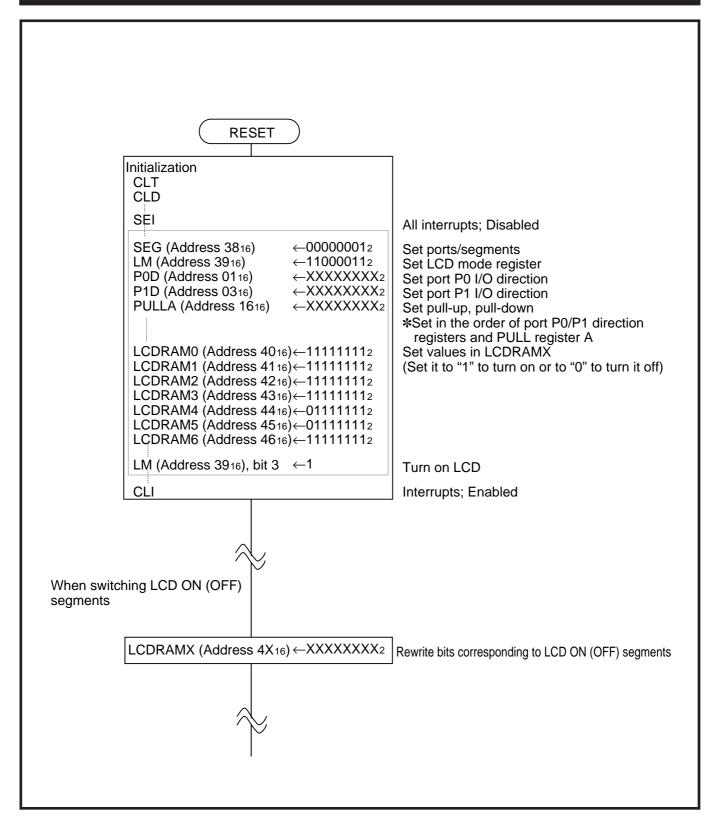
Fig. 2.7.14 Control procedure
