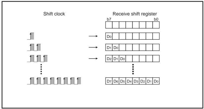
Fig. 2.5.5 Receive operation in clock synchronous mode
