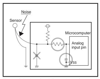
Fig. 3.2.5 Analog signal line and a resistor and a capacitor
