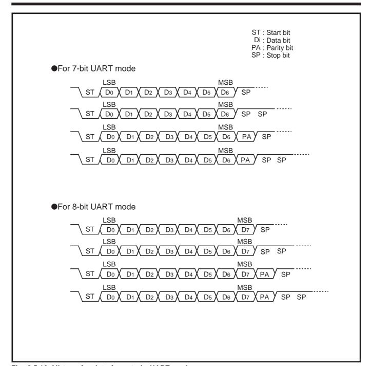
Fig. 2.5.10 All transfer data formats in UART mode
