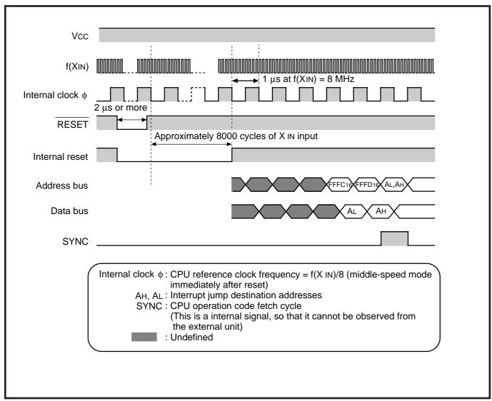
Fig. 2.9.2 Internal processing sequence immediately after reset release
