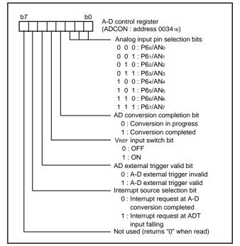
Fig. 26 Structure of A-D control register
