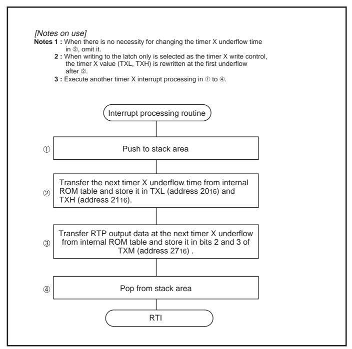
Fig. 2.3.40 Timer X interrupt processing procedure example when real time port is used
