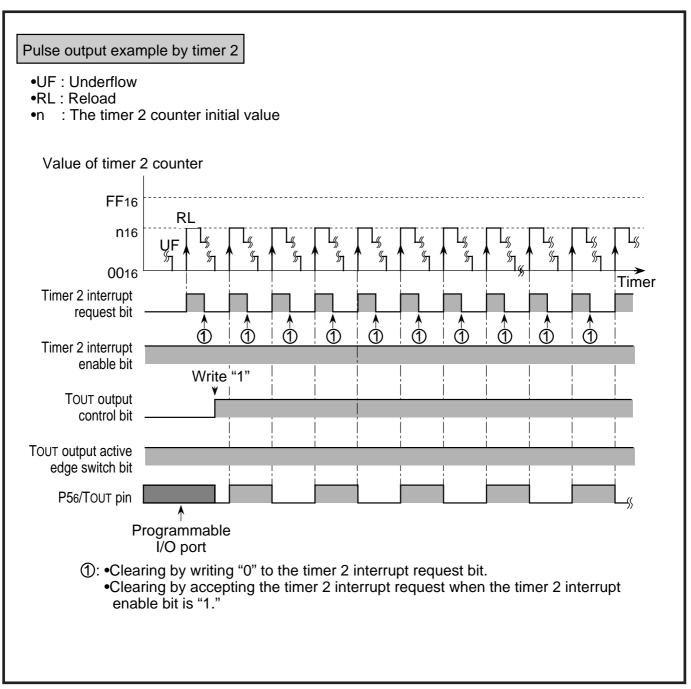
Fig. 2.4.4 Pulse output example
