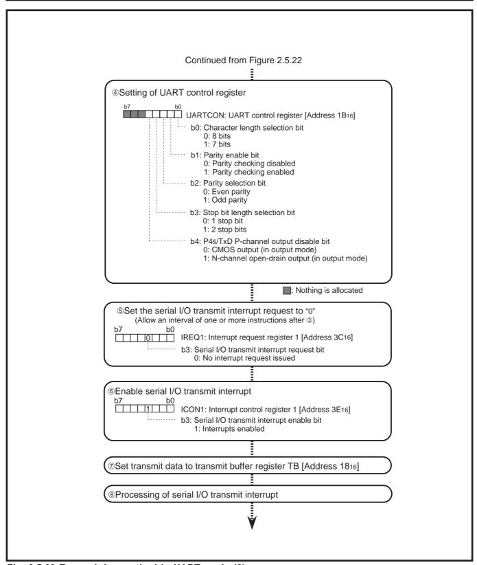
Fig. 2.5.23 Transmitting method in UART mode (2)
