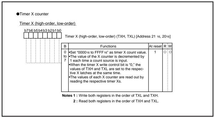
Fig. 2.3.13 Structure of timer X counter
