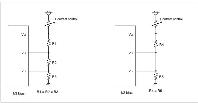
Fig. 30 Example of circuit at each bias
