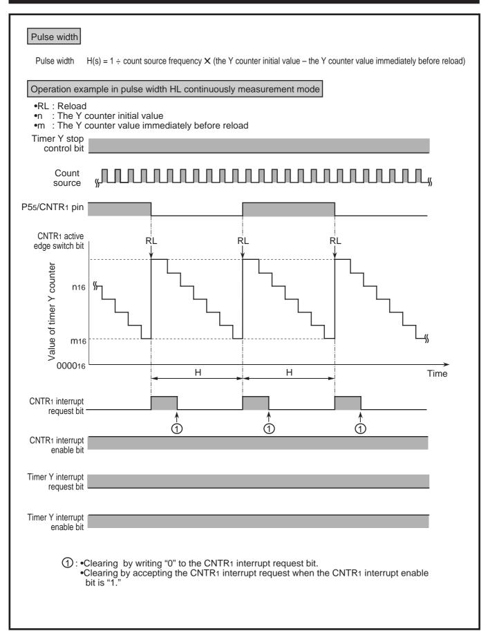
Fig. 2.3.9 Pulse width HL continuously measurement mode operation example
