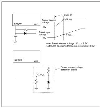
Fig. 35 Example of reset circuit
