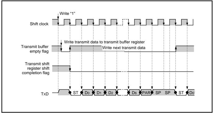
Fig. 2.5.11 Transmit timing example in UART mode
