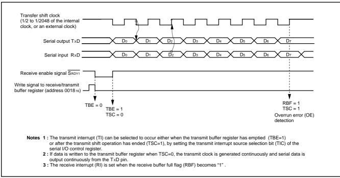
Fig. 22 Operation of clock synchronous serial I/O function
