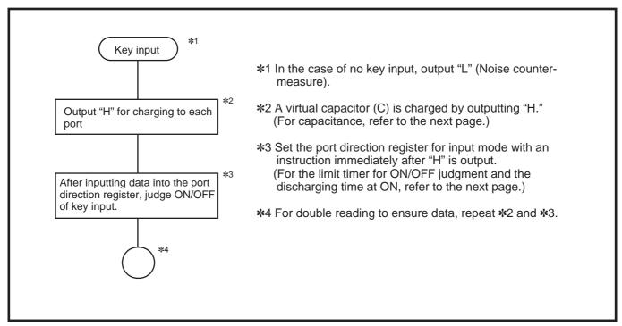
Fig. 2.1.8 Key input control procedure 1
