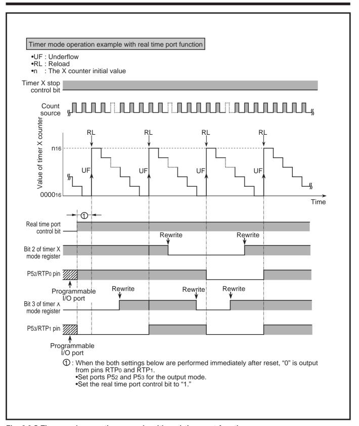
Fig. 2.3.5 Timer mode operation example with real time port function
