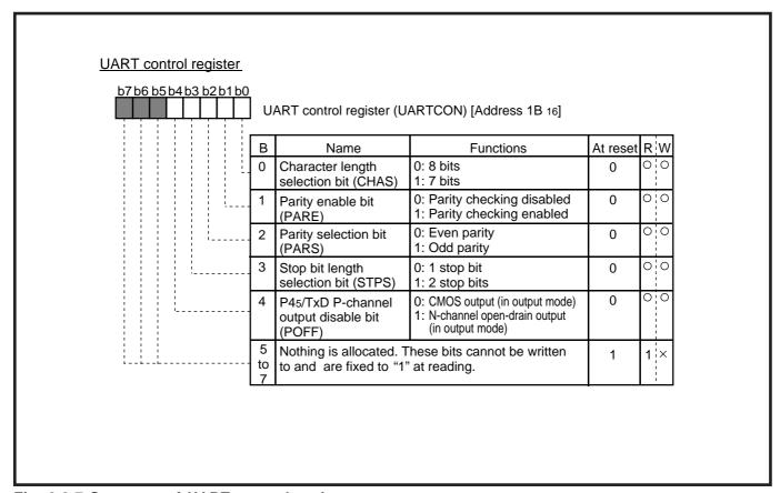
Fig. 3.3.7 Structure of UART control register
