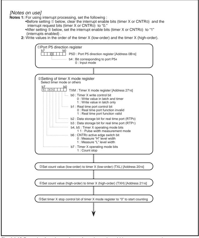
Fig. 2.3.25 Example of setting registers for using pulse width measurement mode
