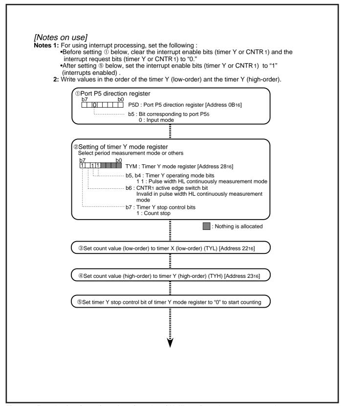
Fig. 2.3.30 Example of setting registers for using pulse width HL continuously measurement mode
