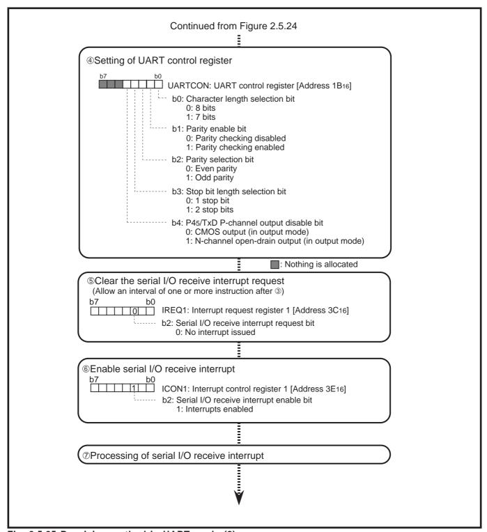
Fig. 2.5.25 Receiving method in UART mode (2)
