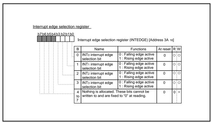
Fig. 3.3.15 Structure of interrupt edge selection register
