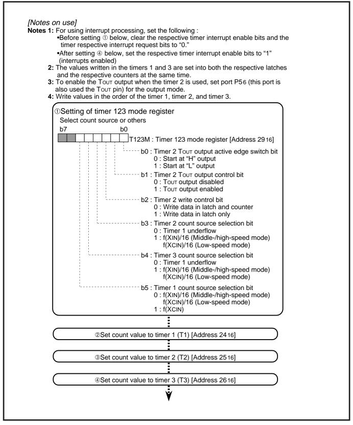
Fig. 2.4.13 Example of setting registers for timers 1, 2, and 3
