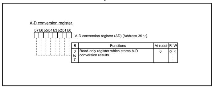
Fig. 2.6.5 Structure of A-D conversion register
