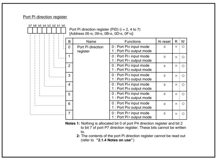
Fig. 3.3.2 Structure of port Pi (i = 2, 4 to 7) direction registers
