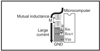
Fig. 3.2.6 Wiring for a large current signal line
