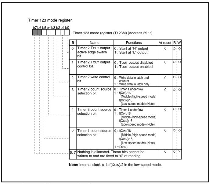
Fig. 2.4.8 Structure of timer 123 mode register
