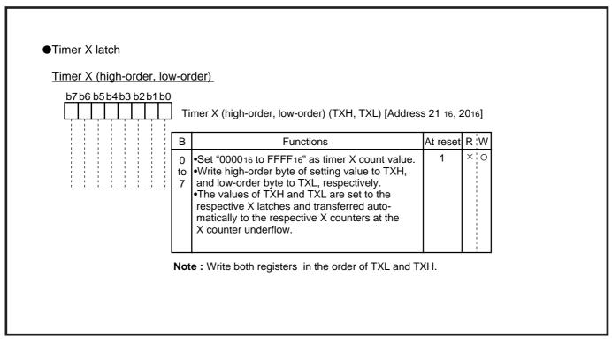
Fig. 2.3.12 Structure of timer X latch
