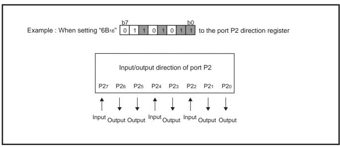
Fig. 2.1.4 Port direction register setting example
