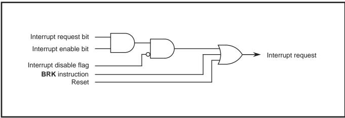
Fig. 2.2.5 Interrupt control diagram
