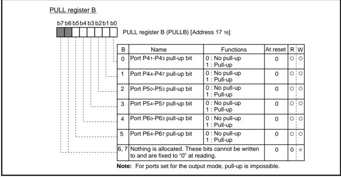
Fig. 2.1.6 Structure of PULL register B
