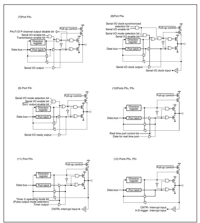
Fig. 12 Port block diagram (2)
