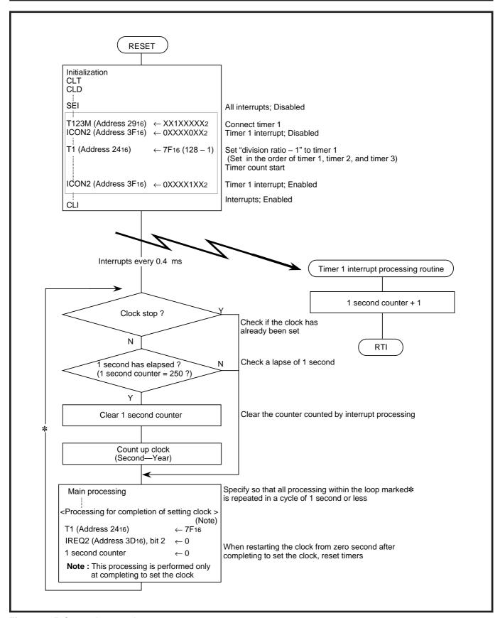
Fig. 2.4.15 Control procedure
