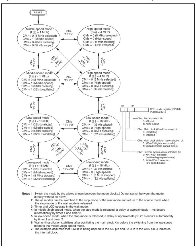
Fig. 2.8.4 State transitions of internal clock  $\phi$
