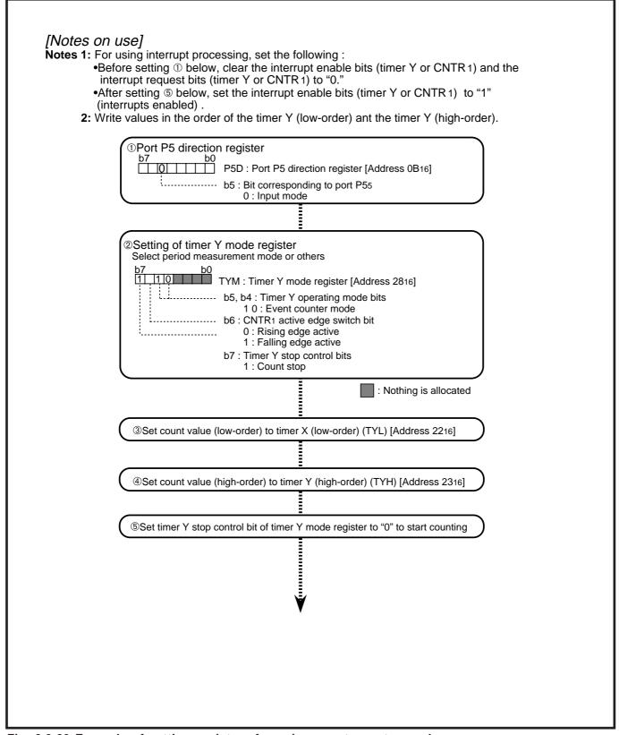
Fig. 2.3.29 Example of setting registers for using event counter mode
