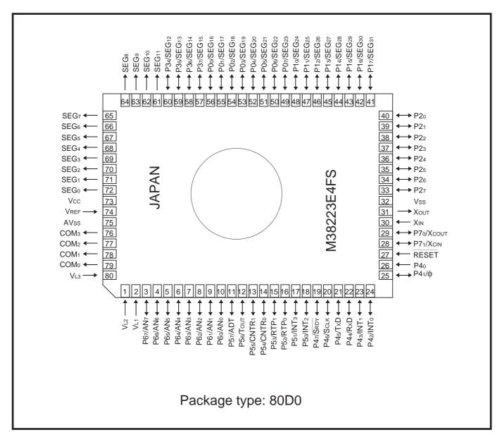
Fig. 3.1.1 Pin configuration of EPROM version (top view)
