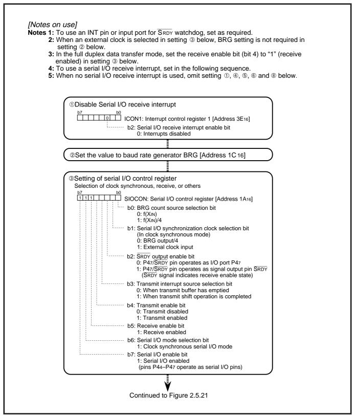
Fig. 2.5.20 Receiving method in clock synchronous mode (1)
