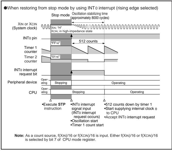
Fig. 2.8.2 Execution sequence example at restoration by occurrence of INTo Interrupt request
