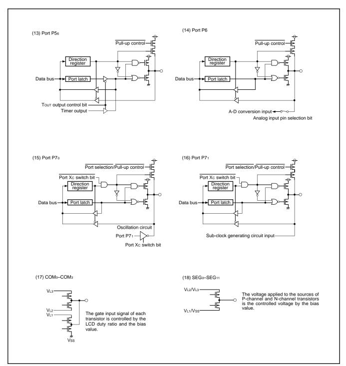
Fig. 13 Port block diagram (3)
