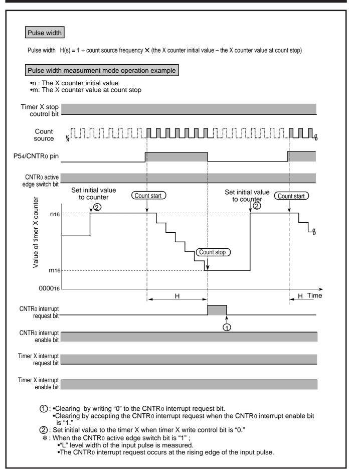
Fig. 2.3.4 Pulse width measurement mode operation example
