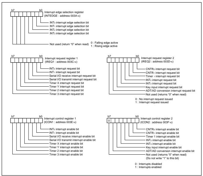
Fig. 15 Structure of interrupt-related registers
