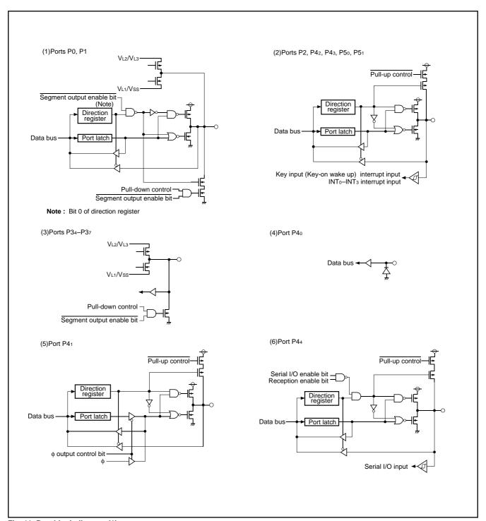
Fig. 11 Port block diagram (1)
