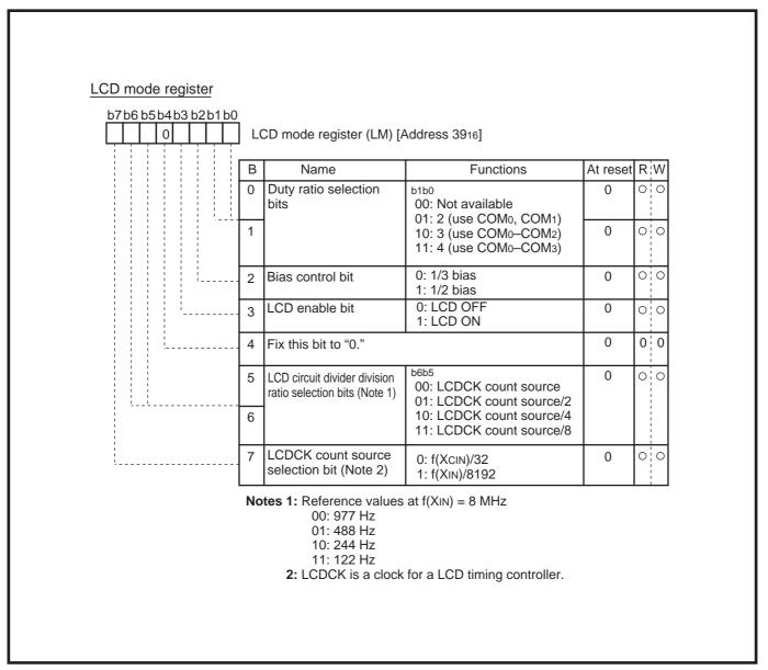
Fig. 2.7.3 Structure of LCD mode register
