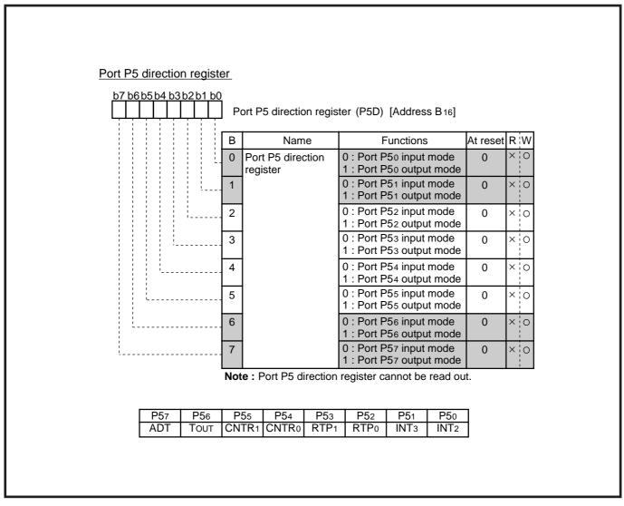
Fig. 2.3.11 Structure of port P5 direction register
