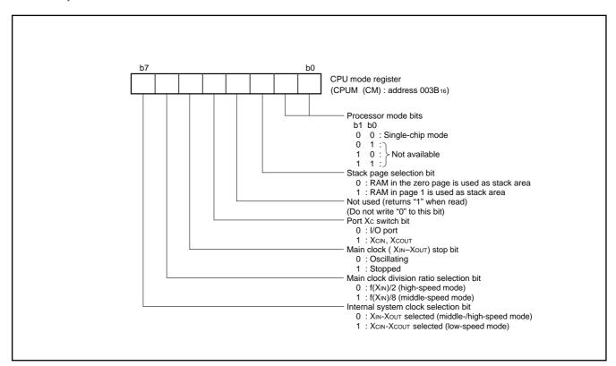
Fig. 7 Structure of CPU mode register
