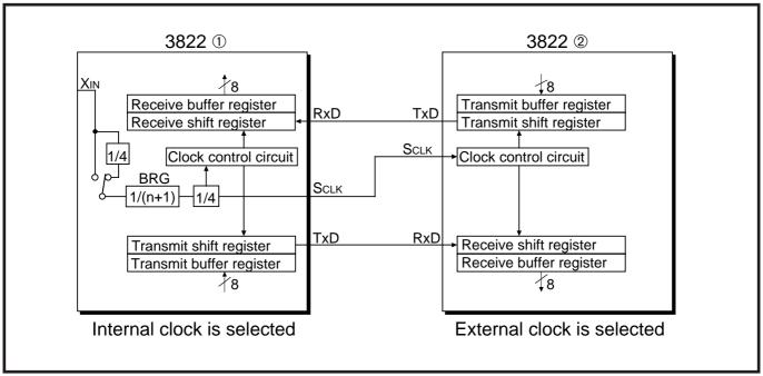
Fig. 2.5.1 External connection example in clock synchronous mode
