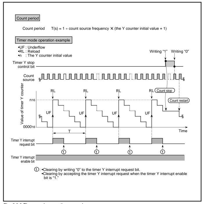
Fig. 2.3.6 Timer mode operation example
