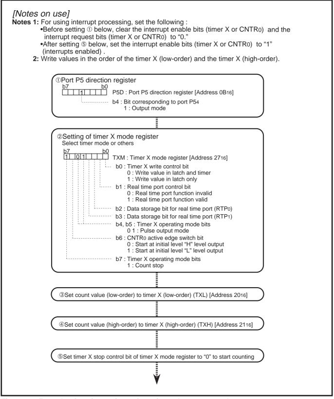
Fig. 2.3.23 Example of setting registers for using pulse output mode
