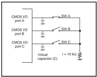
Fig. 2.1.7 Connection example 1 for key input
