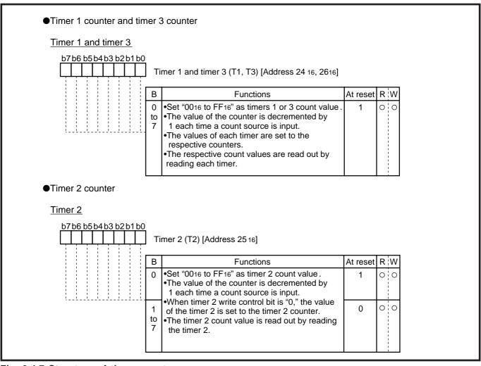
Fig. 2.4.7 Structure of timer counters
