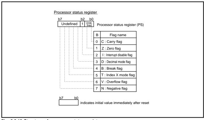
Fig. 2.2.13 Structure of processor status register
