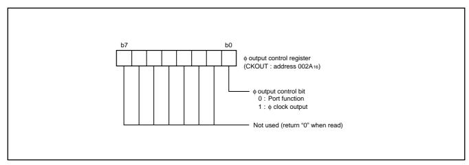
Fig. 34 Structure of  $\varphi$  output control register
