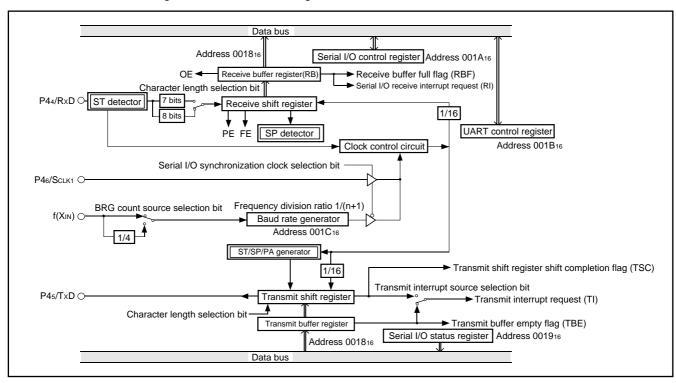
Fig. 23 Block diagram of UART serial I/O
