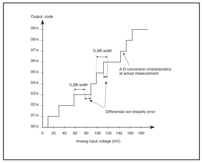
Fig. 2.6.12 Differential non-linearity error of A-D converter
