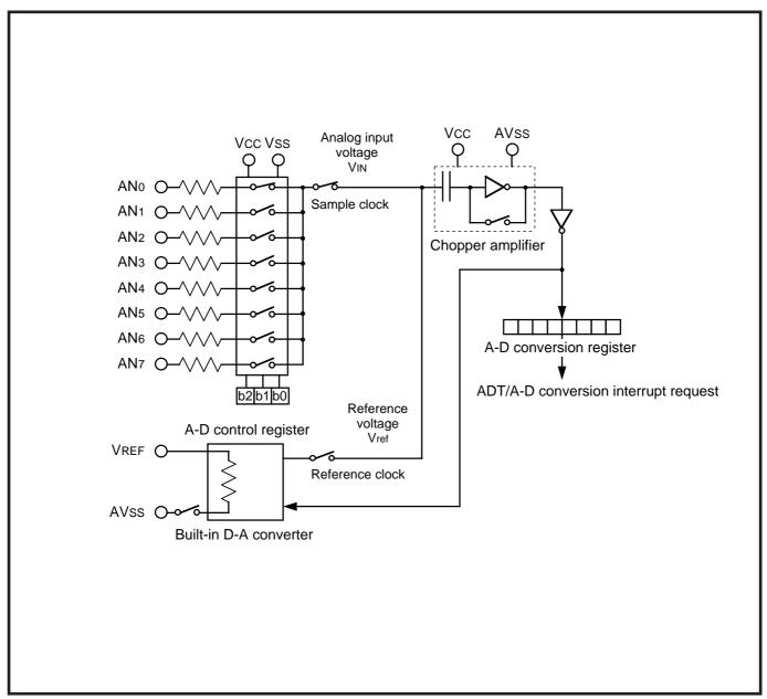
Fig. 2.6.2 A-D converter equivalent connection diagram
