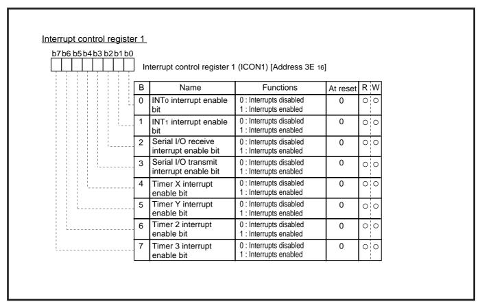
Fig. 3.3.19 Structure of interrupt control register 1
