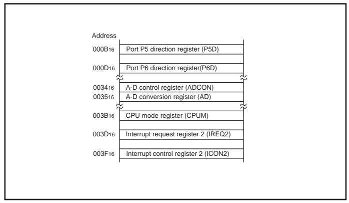
Fig. 2.6.3 Memory allocation of A-D converter-related registers
