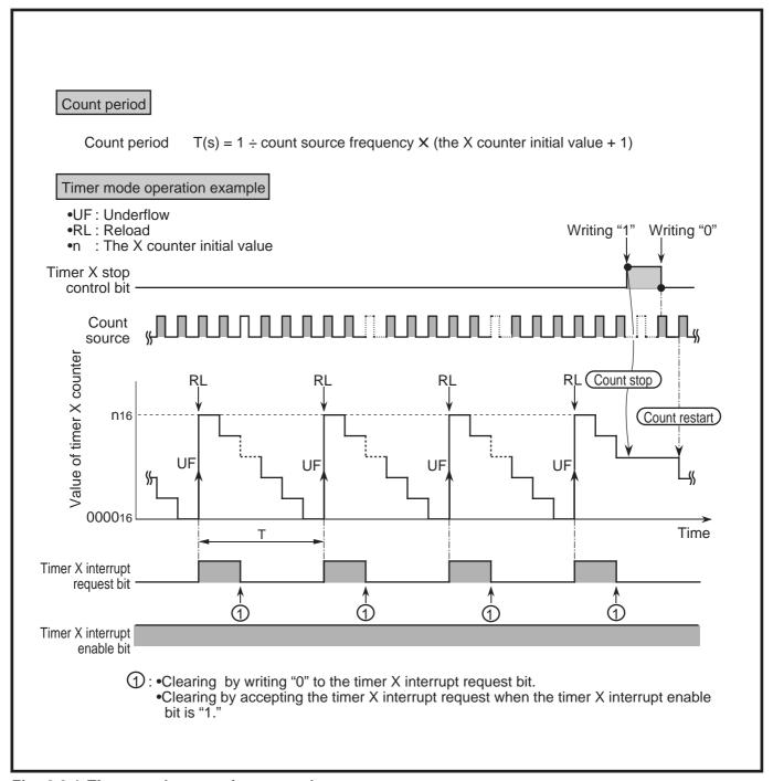
Fig. 2.3.1 Timer mode operation example
