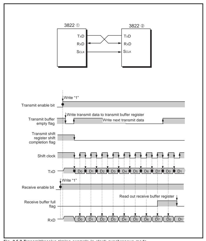
Fig. 2.5.7 Transmit/receive timing example in clock synchronous mode
