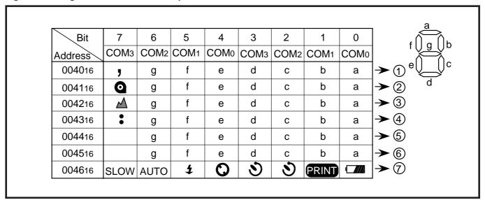
Fig. 2.7.12 LCD display RAM setting example
