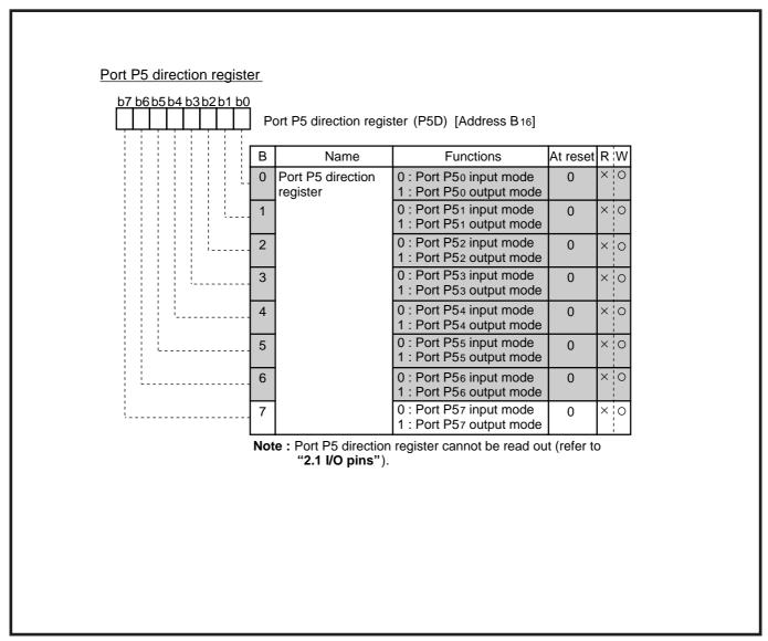
Fig. 2.6.7 Structure of port P5 direction register
