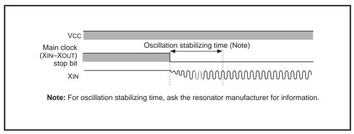
Fig. 2.10.7 Oscillation stabilizing time at reoscillation of XIN
