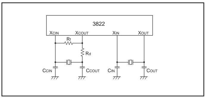
Fig. 2.10.1 Oscillation circuit example using ceramic resonators
