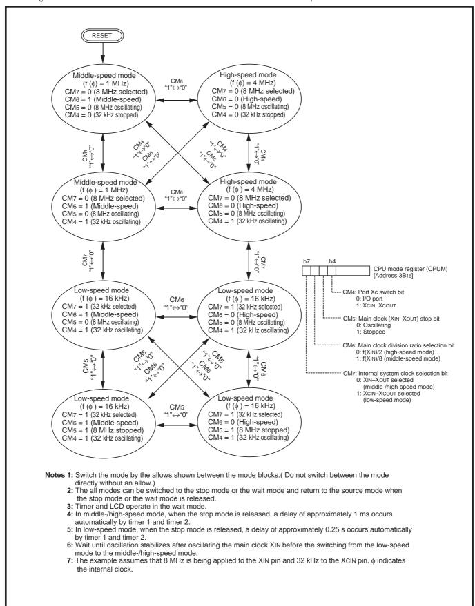
Fig. 2.10.5 State transitions of internal clock  $\phi$
