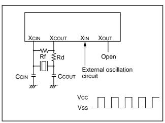
Fig. 39 External clock input circuit
