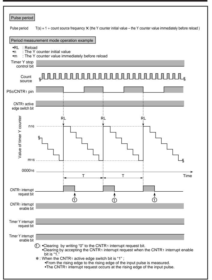
Fig. 2.3.7 Period measurement mode operation example
