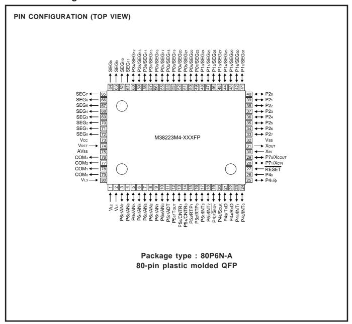
Pin configuration of M38223M4-XXXFP
