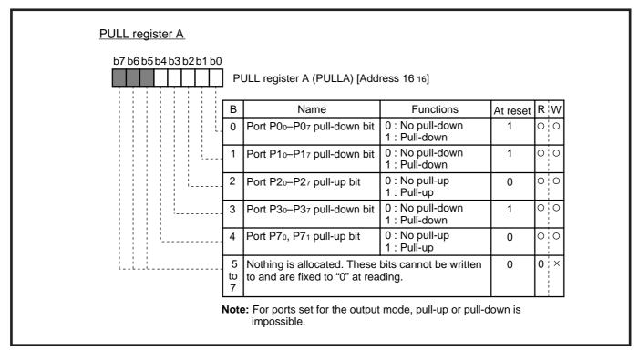
Fig. 2.1.5 Structure of PULL register A
