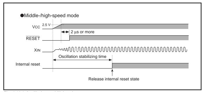
Fig. 2.10.6 Oscillation stabilizing time at poweron
