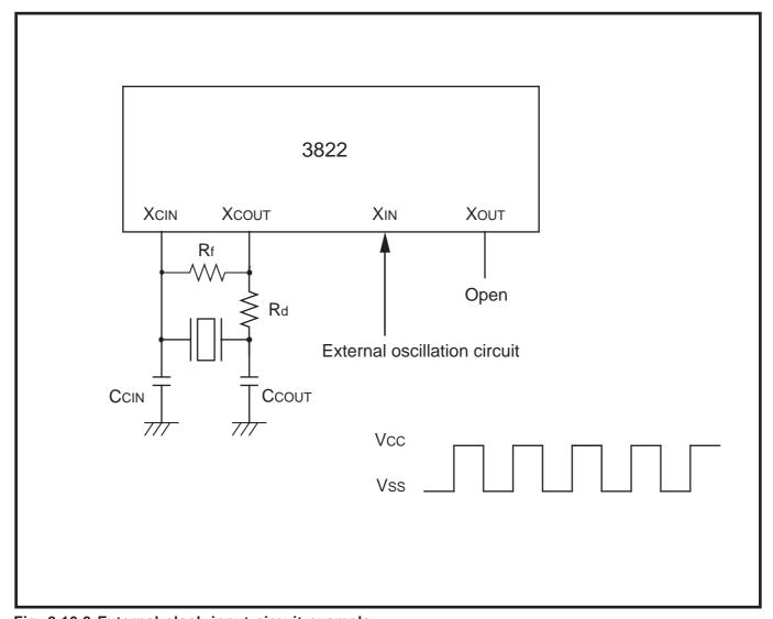
Fig. 2.10.2 External clock input circuit example
