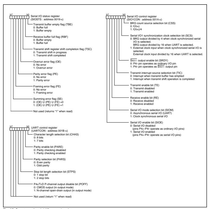
Fig. 25 Structure of serial I/O control registers
