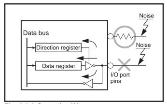
Fig. 3.2.9 Setup for I/O ports
