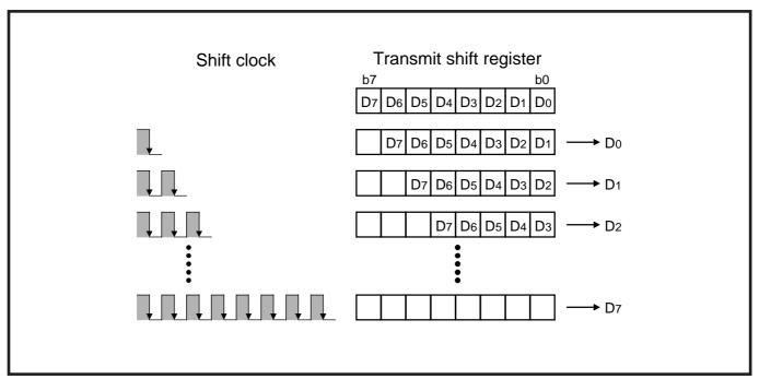
Fig. 2.5.3 Transmit operation in clock synchronous mode
