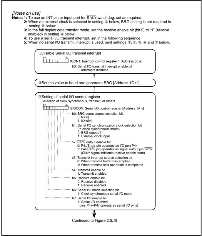
Fig. 2.5.18 Transmitting method in clock synchronous mode (1)
