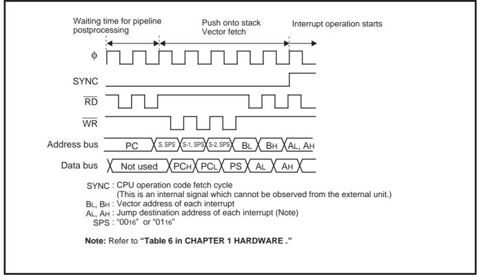
Fig. 2.2.4 Timing after acceptance of interrupt request
