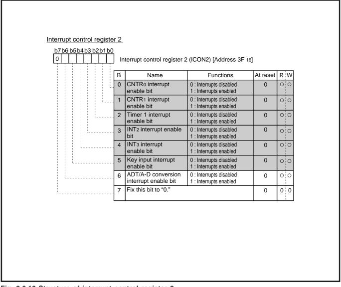
Fig. 2.6.10 Structure of interrupt control register 2
