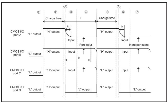
Fig. 2.1.12 Timing diagram 2 where switch A is pressed
