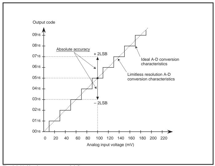
Fig. 2.6.11 Absolute accuracy of A-D converter
