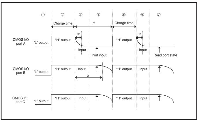
Fig. 2.1.9 Timing diagram 1 where switch A is pressed
