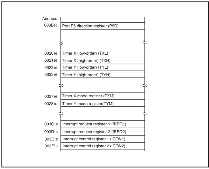
Fig. 2.3.10 Memory allocation of timer X- and timer Y-related registers
