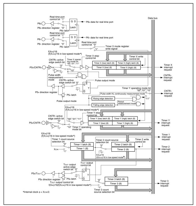
Fig. 17 Timer block diagram
