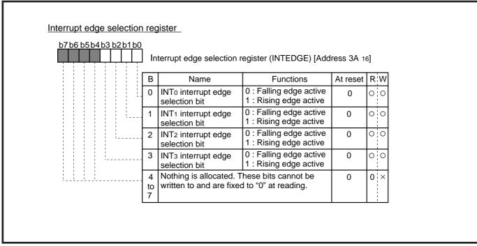
Fig. 2.2.8 Structure of interrupt edge selection register
