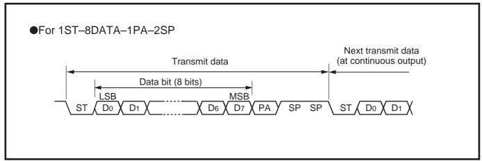
Fig. 2.5.9 Transfer data format in UART mode
