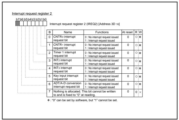
Fig. 2.2.10 Structure of interrupt request register 2
