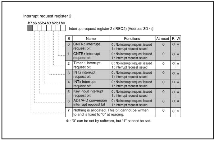
Fig. 2.4.10 Structure of interrupt request register 2
