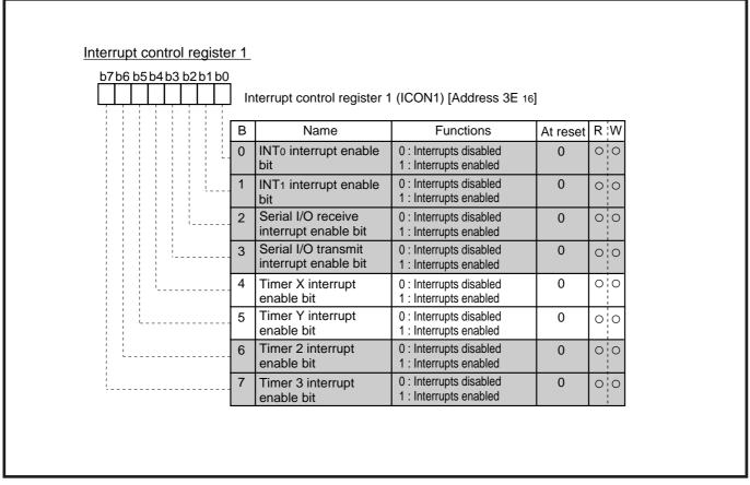
Fig. 2.3.20 Structure of interrupt control register 1
