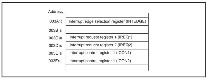
Fig. 2.2.7 Memory allocation of interrupt-related registers
