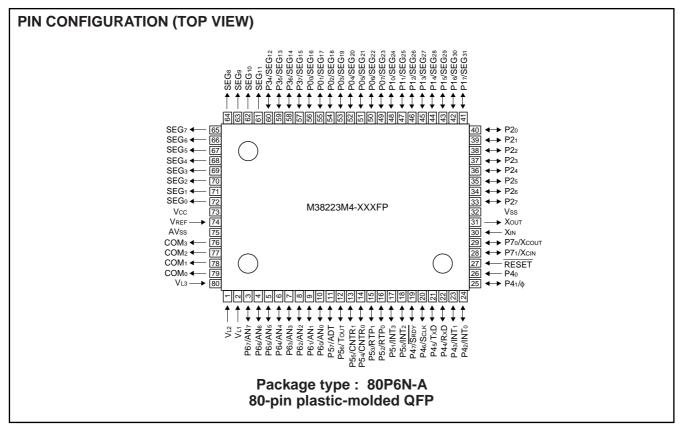
Fig. 1 Pin configuration of M38223M4-XXXFP
