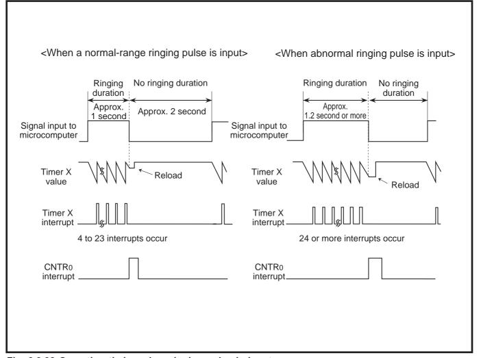
Fig. 2.3.38 Operation timing when ringing pulse is input
