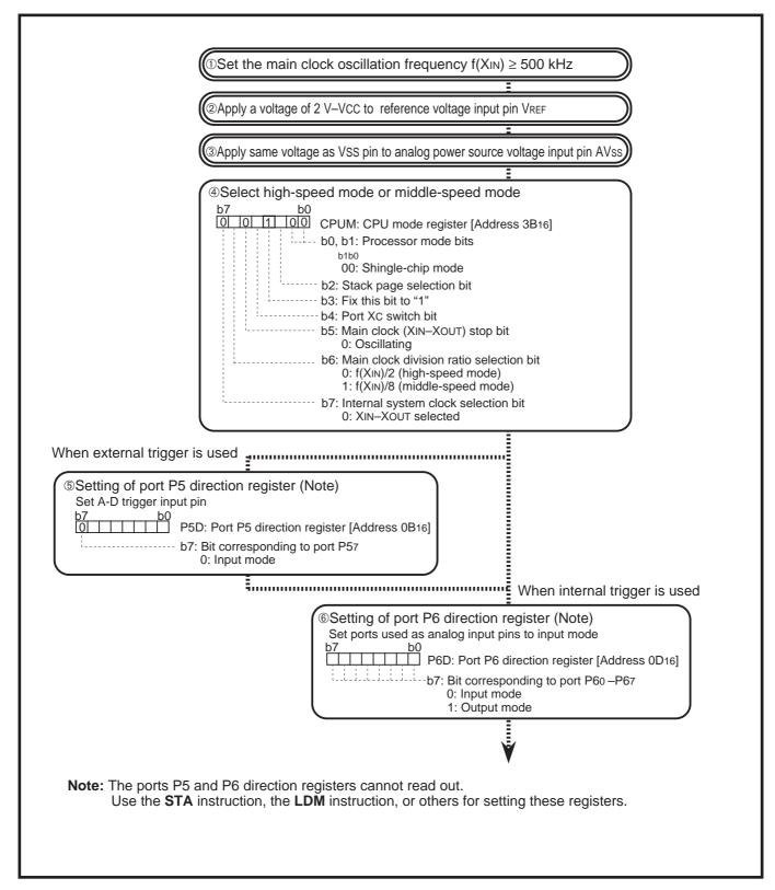
Fig. 2.6.13 Operating conditions for using A-D converter
