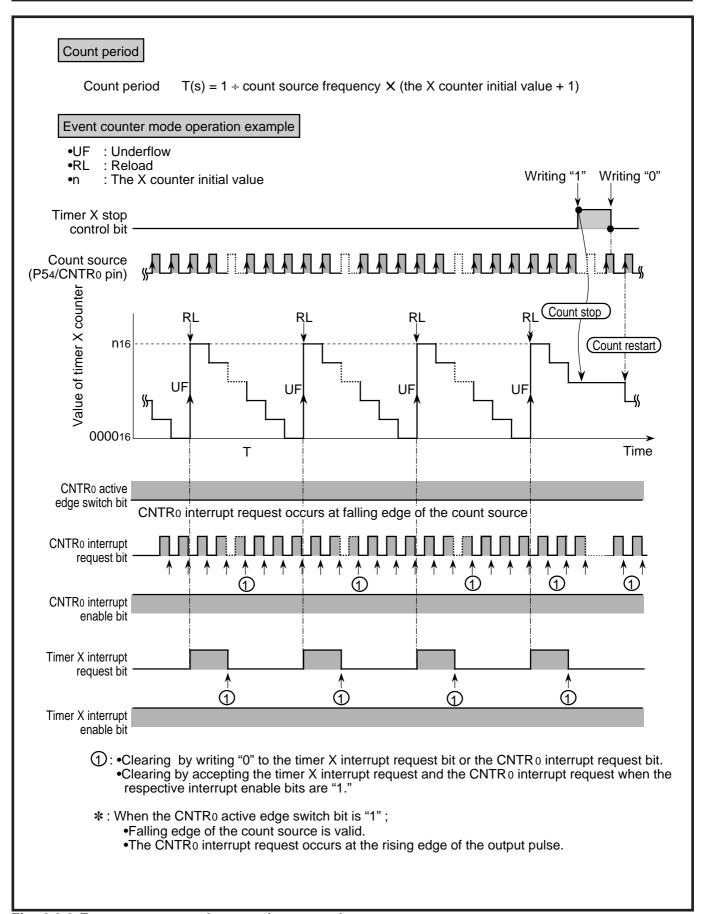
Fig. 2.3.3 Event counter mode operation example
