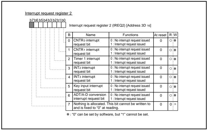
Fig. 3.3.18 Structure of interrupt request register 2
