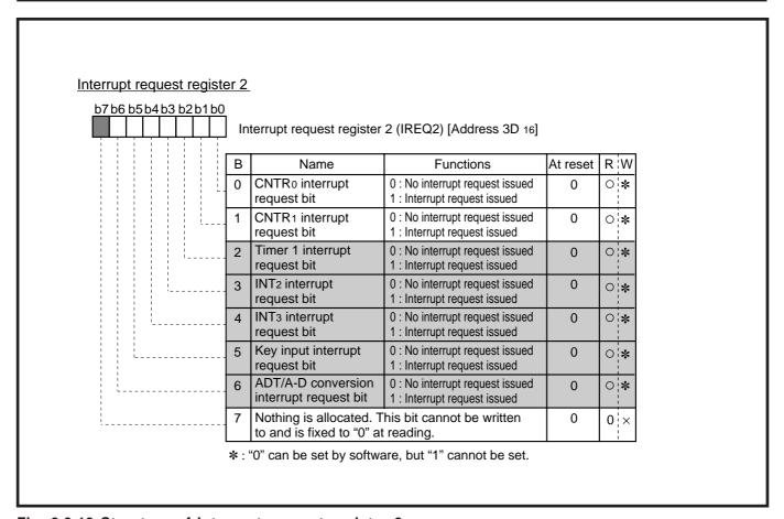
Fig. 2.3.19 Structure of interrupt request register 2
