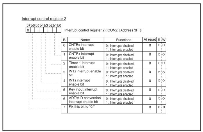
Fig. 2.2.12 Structure of interrupt control register 2
