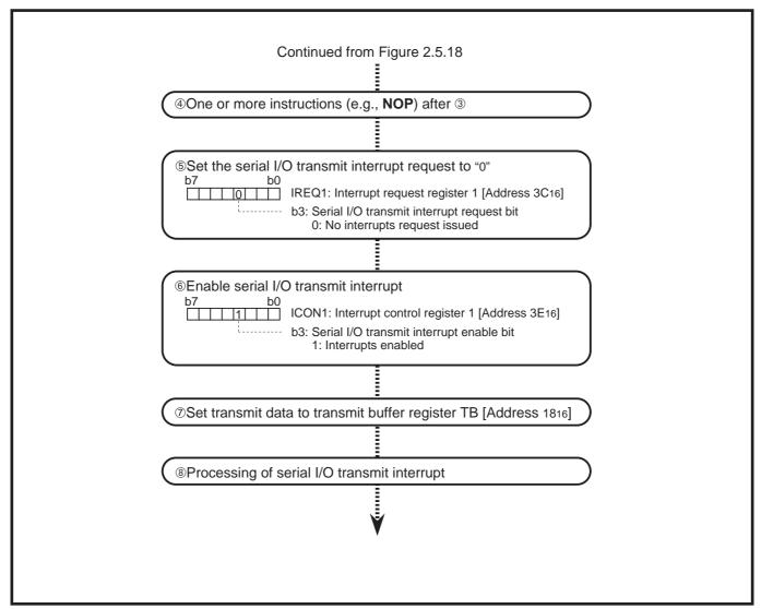
Fig. 2.5.19 Transmitting method in clock synchronous mode (2)
