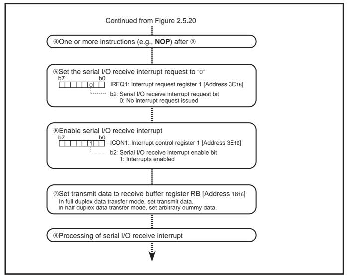
Fig. 2.5.21 Receiving method in clock synchronous mode (2)
