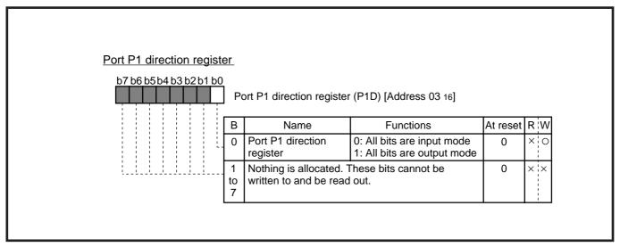
Fig. 2.7.5 Structure of port P1 direction register
