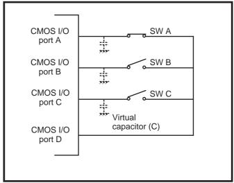
Fig. 2.1.10 Connection example 2 for key input
