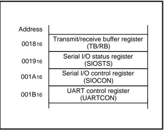
Fig. 2.5.13 Memory allocation of serial I/O-related registers
