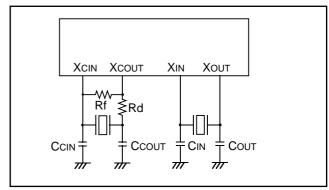
Fig. 38 Ceramic resonator circuit
