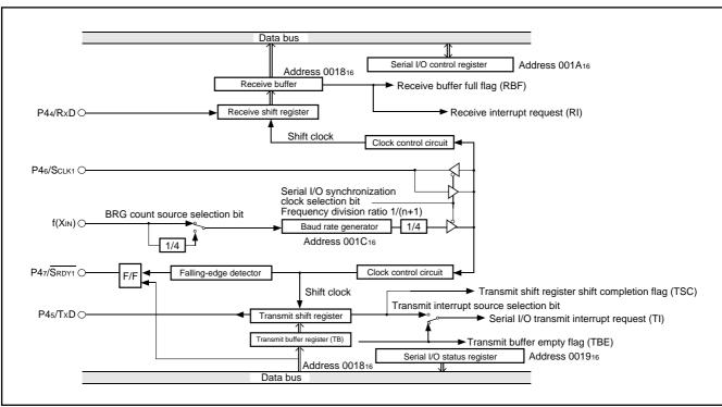
Fig. 21 Block diagram of clock synchronous serial I/O
