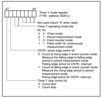
Fig. 19 Structure of timer Y mode register
