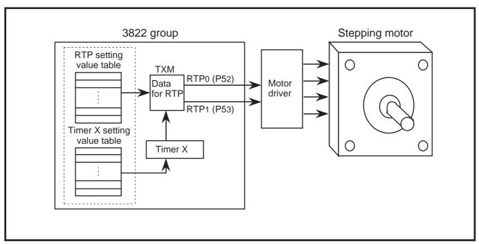
Fig. 2.3.41 Application connection example when RTP is used
