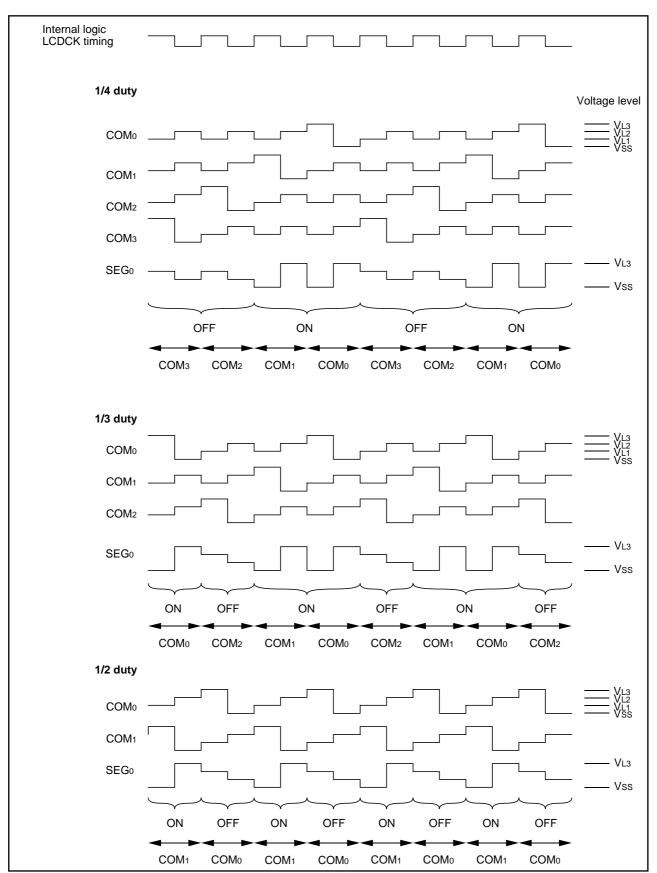
Fig. 33 LCD drive waveform (1/3 bias)
