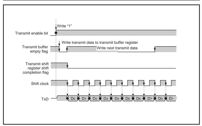
Fig. 2.5.4 Transmit timing example in clock synchronous mode
