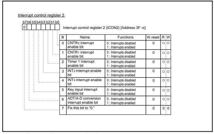
Fig. 3.3.20 Structure of interrupt control register 2
