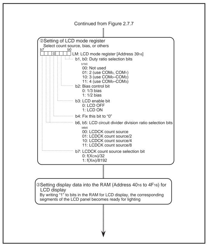
Fig. 2.7.8 Example of setting registers for LCD display (2)
