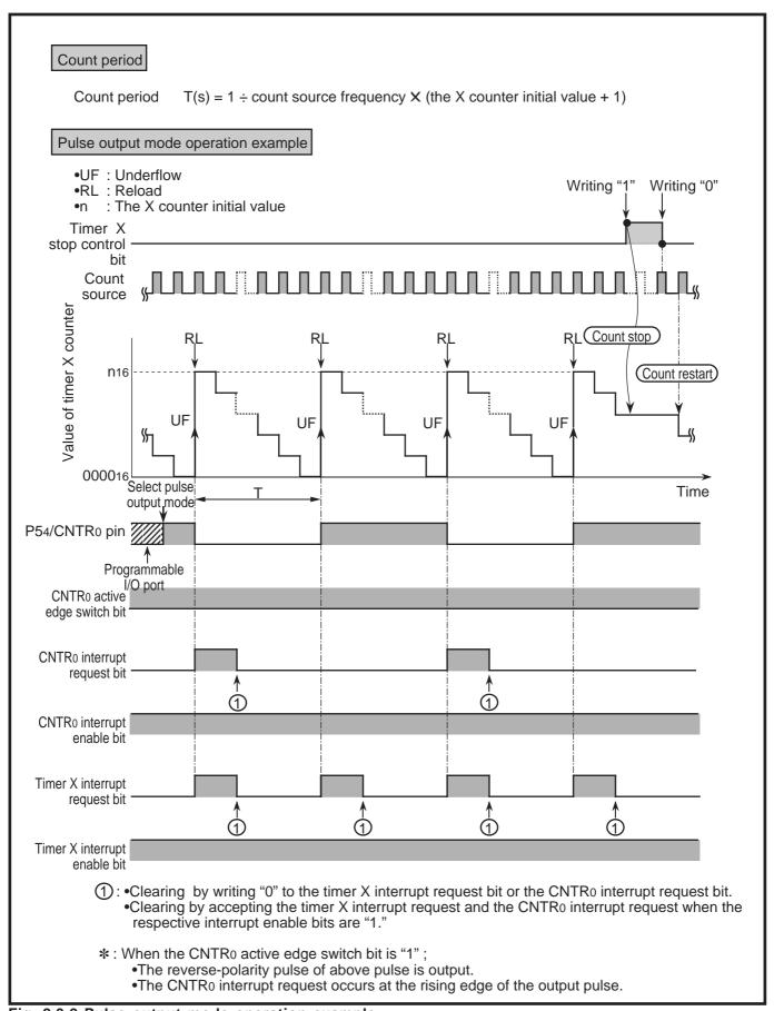
Fig. 2.3.2 Pulse output mode operation example
