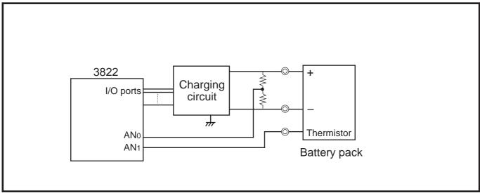
Fig. 2.6.18 Example of peripheral circuit
