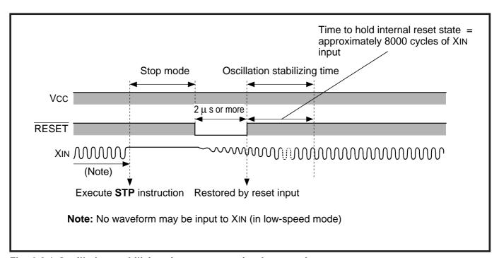
Fig. 2.8.1 Oscillation stabilizing time at restoration by reset input
