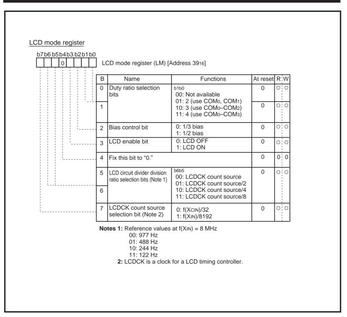
Fig. 3.3.14 Structure of LCD mode register
