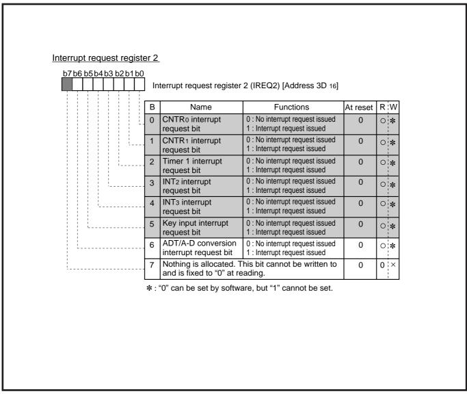
Fig. 2.6.9 Structure of interrupt request register 2
