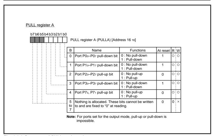
Fig. 3.3.3 Structure of PULL register A
