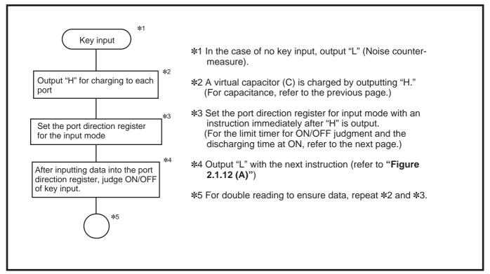
Fig. 2.1.11 Key input control procedure 2
