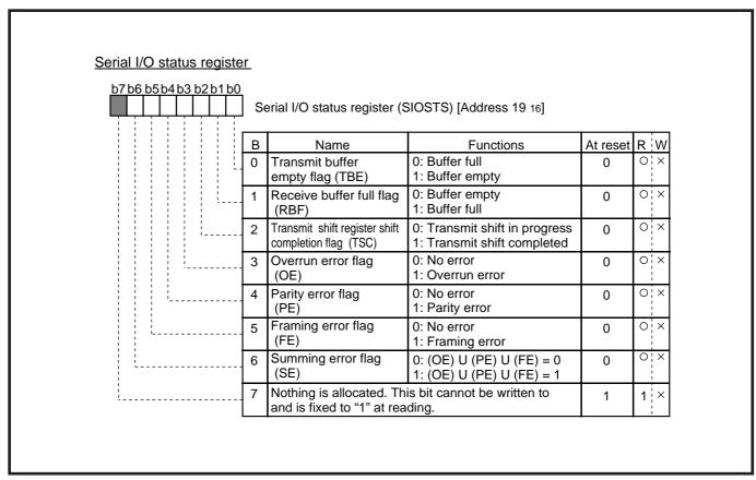
Fig. 3.3.5 Structure of serial I/O status register
