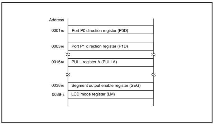
Fig. 2.7.1 Memory allocation of LCD display-related registers
