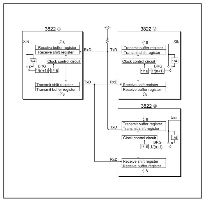
Fig. 2.5.8 External connection example in UART mode
