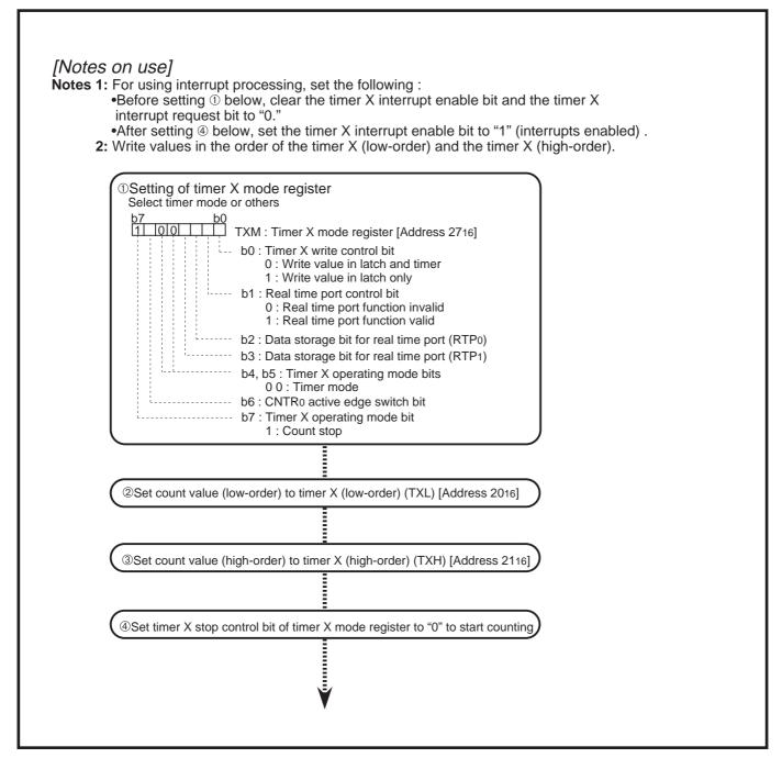
Fig. 2.3.22 Example of setting registers for using timer mode
