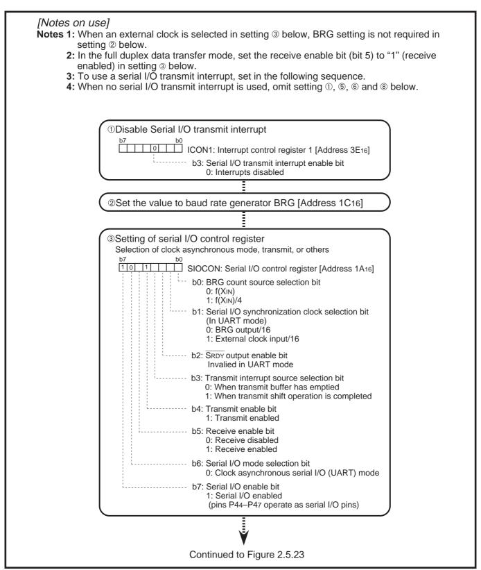
Fig. 2.5.22 Transmitting method in UART mode (1)
