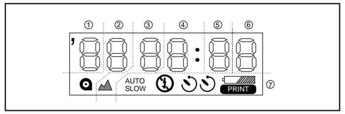
Fig. 2.7.11 Segment allocation example
