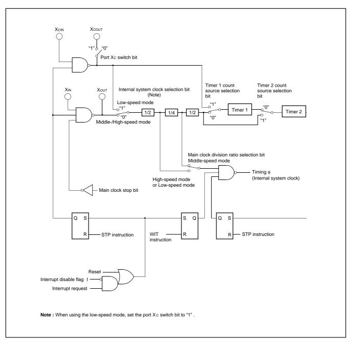
Fig. 40 Clock generating circuit block diagram
