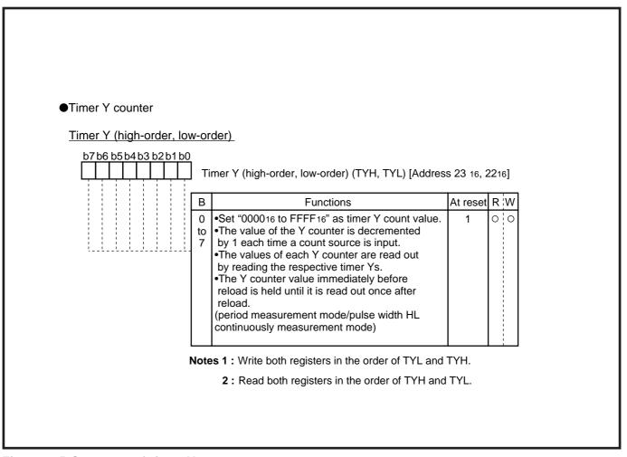
Fig. 2.3.15 Structure of timer Y counter
