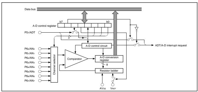
Fig. 27 A-D converter block diagram
