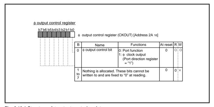
Fig. 2.10.4 Structure of  $\phi$  output control register
