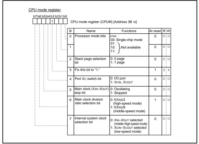
Fig. 3.3.16 Structure of CPU mode register
