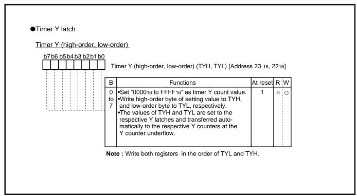
Fig. 2.3.14 Structure of timer Y latch
