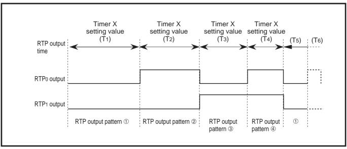
Fig. 2.3.42 RTP output example
