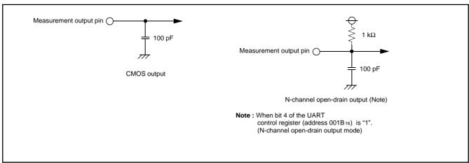
Fig. 43 Circuit for measuring output switching characteristics (1)
