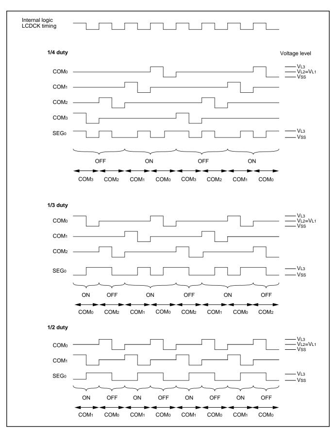
Fig. 32 LCD drive waveform (1/2 bias)
