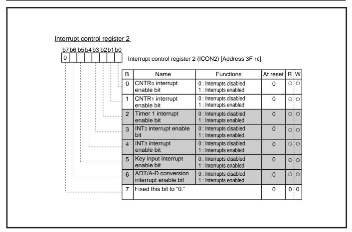
Fig. 2.3.21 Structure of interrupt control register 2
