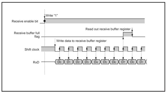
Fig. 2.5.6 Receive timing example in clock synchronous mode
