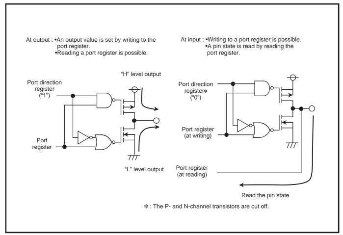
Fig. 2.1.1 I/O port write and read
