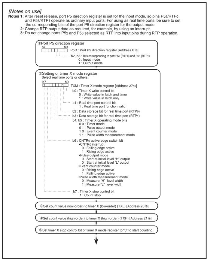
Fig. 2.3.26 Example of setting registers for using real time port
