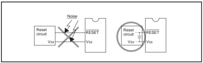
Fig. 3.2.1 Wiring for the RESET input pin
