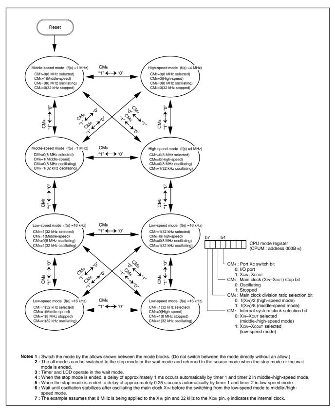
Fig. 41 State transitions of internal clock
