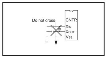
Fig. 3.2.7 Wiring to a signal line where potential levels change frequently
