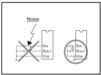
Fig. 3.2.2 Wiring for clock I/O pins
