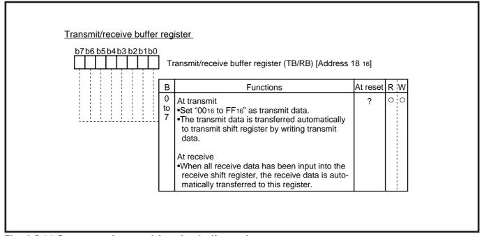
Fig. 2.5.14 Structure of transmit/receive buffer register
