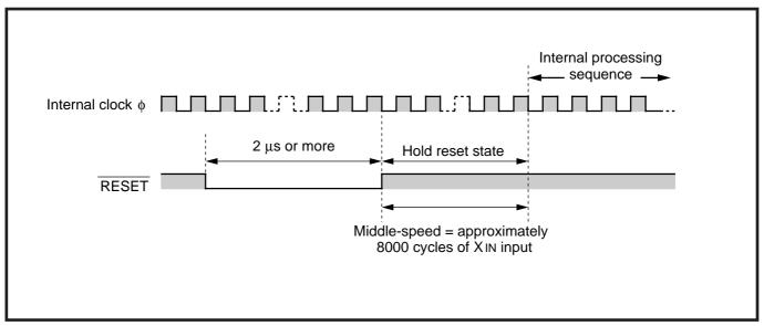
Fig. 2.9.1 Internal reset state hold/release timing
