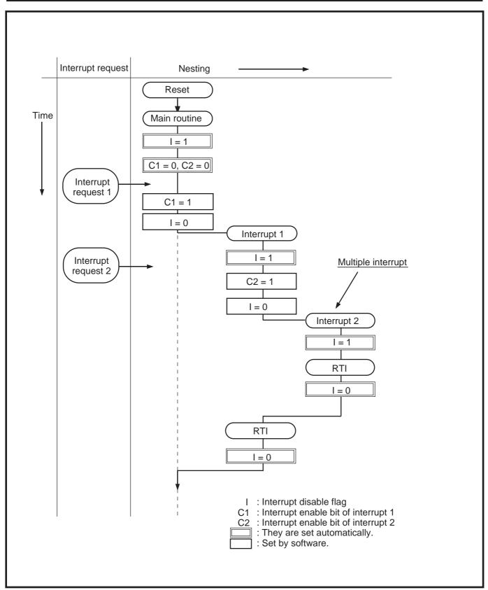
Fig. 2.2.6 Example of multiple interrupts
