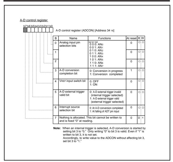
Fig. 3.3.12 Structure of A-D control register
