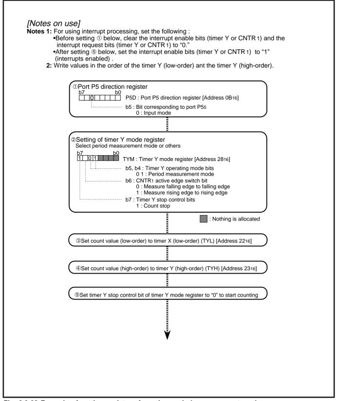
Fig. 2.3.28 Example of setting registers for using period measurement mode
