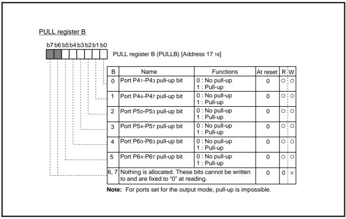
Fig. 3.3.4 Structure of PULL register B
