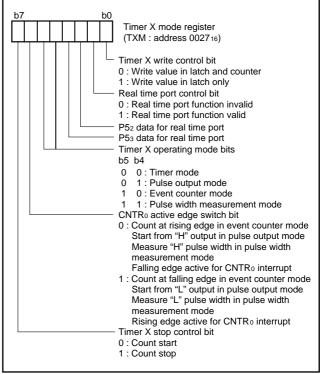
Fig. 18 Structure of timer X mode register
