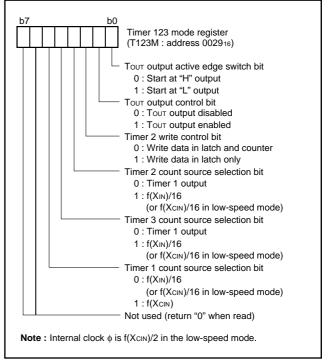
Fig. 20 Structure of timer 123 mode register
