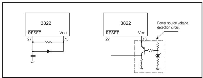
Fig. 2.9.5 Poweron reset circuit examples
