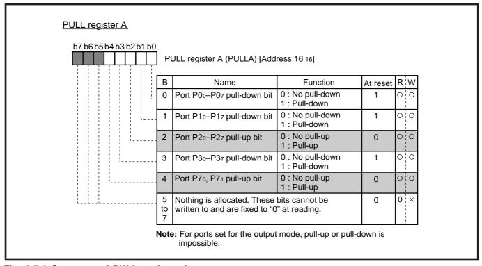
Fig. 2.7.6 Structure of PULL register A
