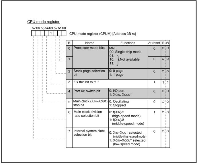
Fig. 2.6.6 Structure of CPU mode register
