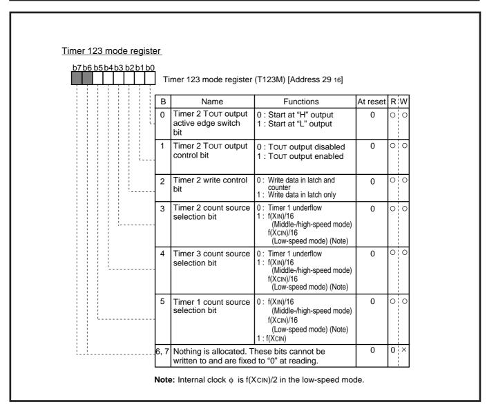
Fig. 3.3.10 Structure of timer 123 mode register
