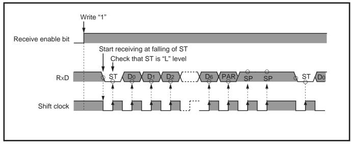
Fig. 2.5.12 Receive timing example in UART mode
