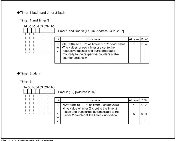
Fig. 2.4.6 Structure of latches
