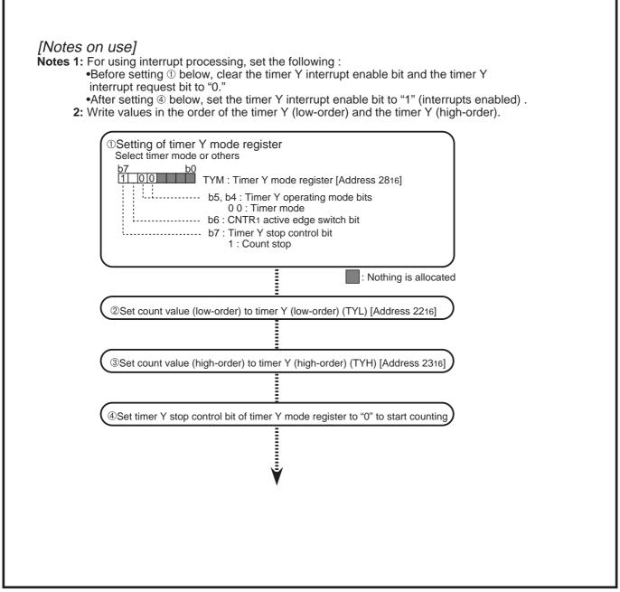
Fig. 2.3.27 Example of setting registers for using timer mode
