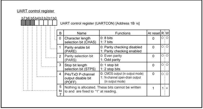
Fig. 2.5.17 Structure of UART control register
