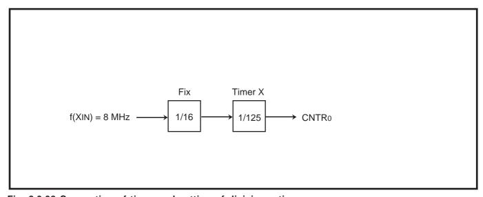
Fig. 2.3.32 Connection of timer and setting of division ratio
