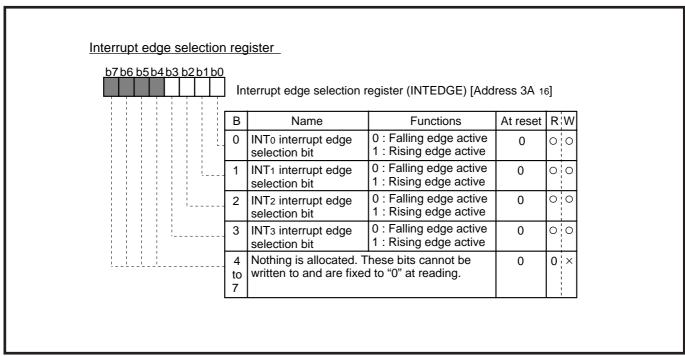
Fig. 2.2.14 Structure of interrupt edge selection register
