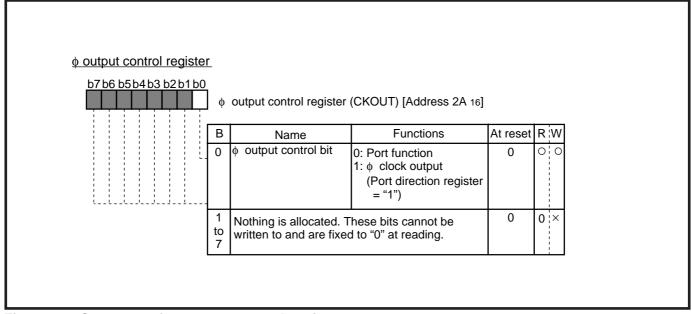
Fig. 3.3.11 Structure of  $\phi$  output control register
