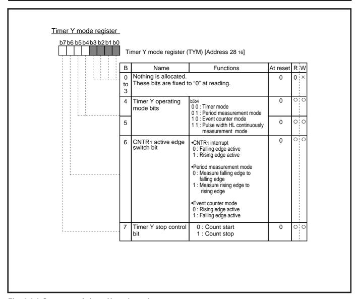
Fig. 3.3.9 Structure of timer Y mode register
