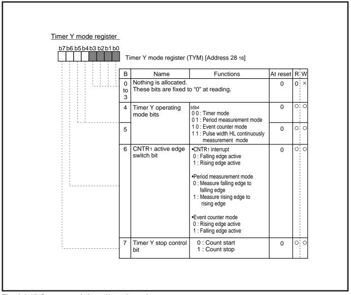
Fig. 2.3.17 Structure of timer Y mode register
