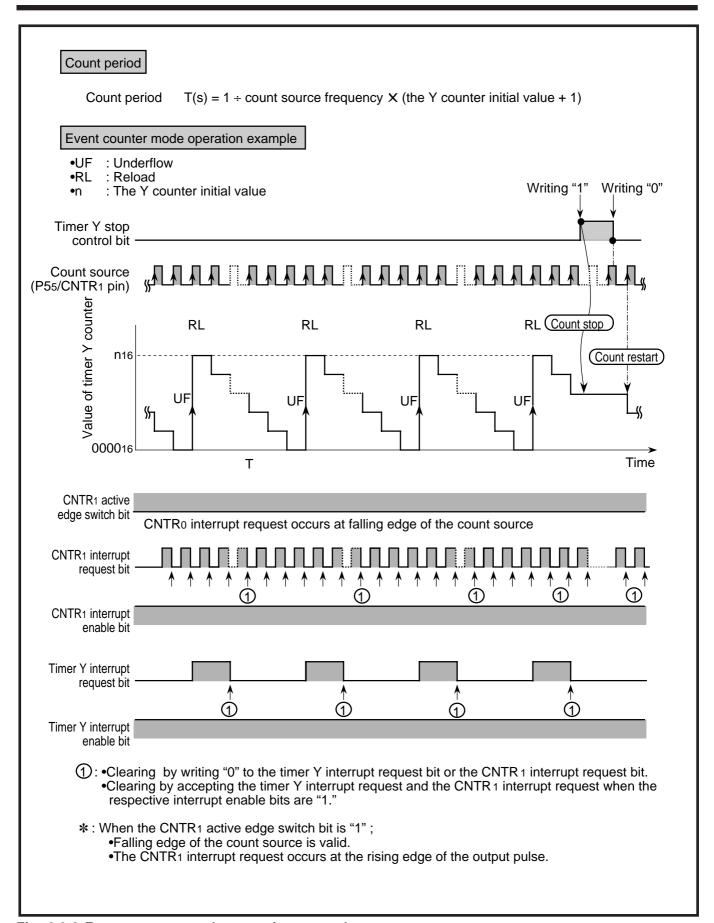
Fig. 2.3.8 Event counter mode operation example
