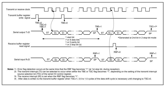
Fig. 24 Operation of UART serial I/O function
