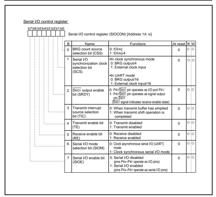
Fig. 3.3.6 Structure of serial I/O control register
