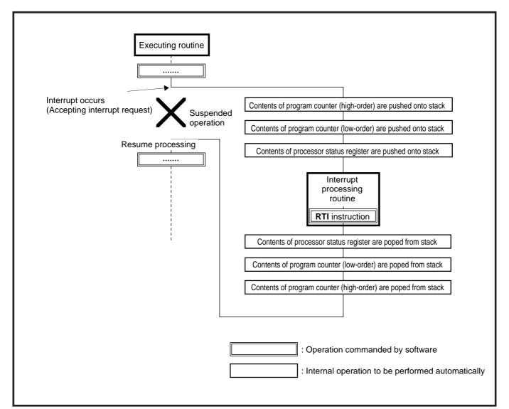
Fig. 2.2.1 Interrupt operation diagram
