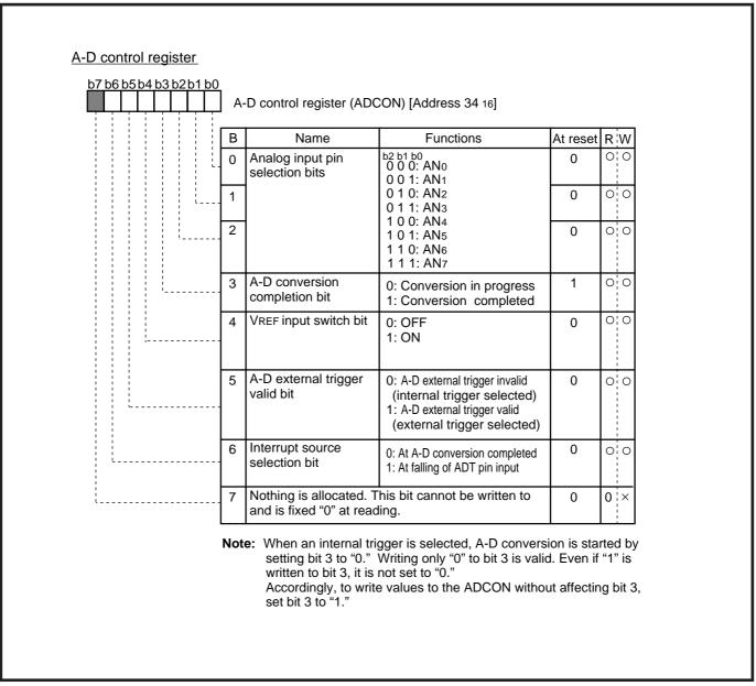
Fig. 2.6.4 Structure of A-D control register
