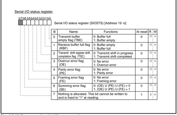
Fig. 2.5.15 Structure of serial I/O status register
