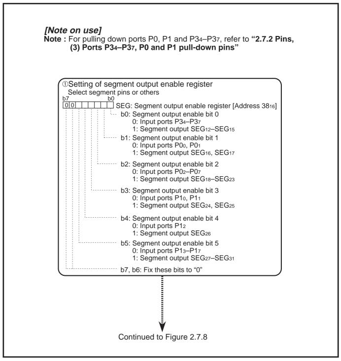
Fig. 2.7.7 Example of setting registers for LCD display (1)
