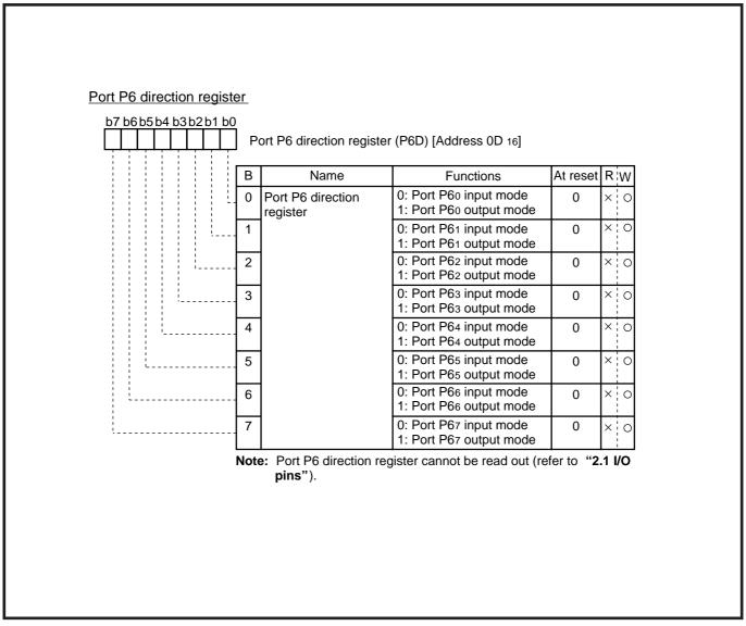
Fig. 2.6.8 Structure of port P6 direction register
