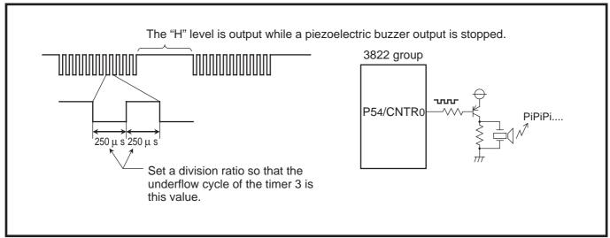
Fig. 2.3.31 Example of peripheral circuit
