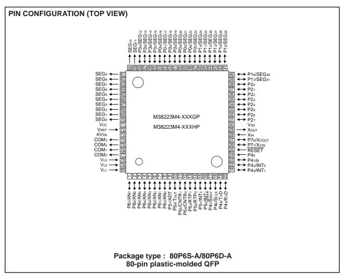
Fig. 2 Pin configuration of M38223M4-XXXGP/HP
