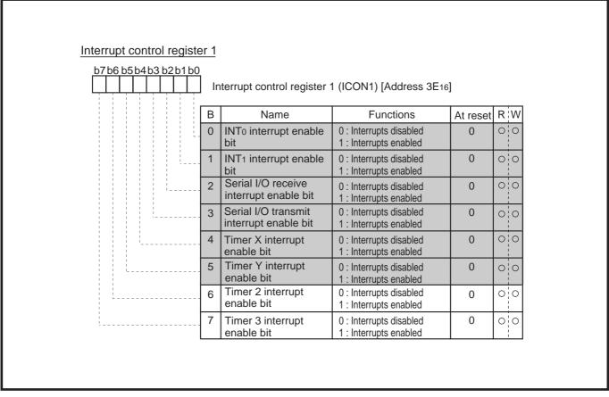
Fig. 2.4.11 Structure of interrupt control register 1
