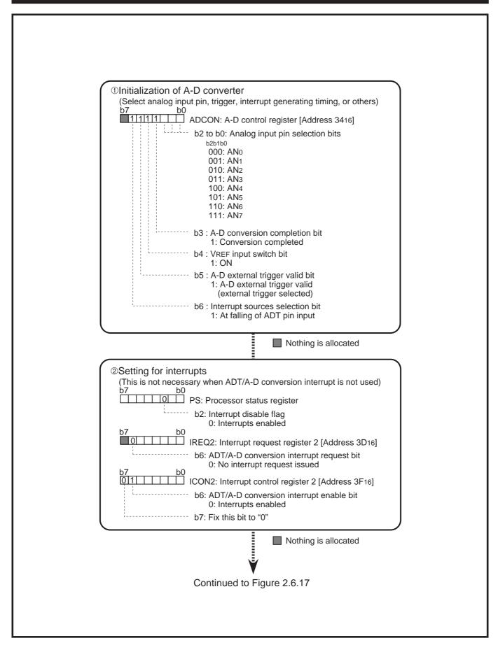
Fig. 2.6.16 Register initialization example when external trigger is selected (1)
