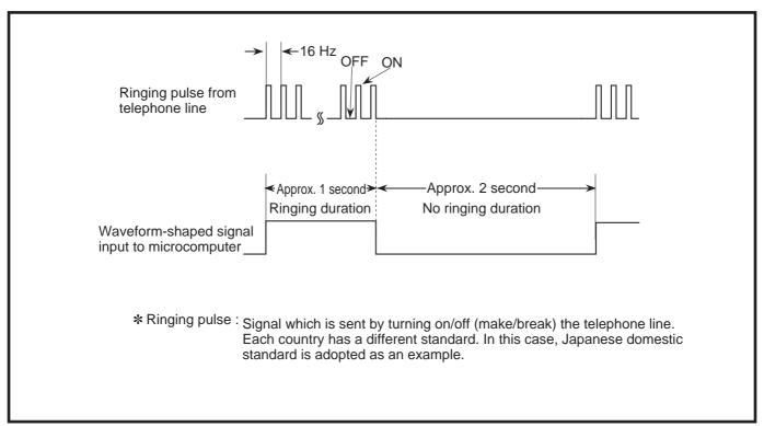
Fig. 2.3.37 Ringer signal waveform
