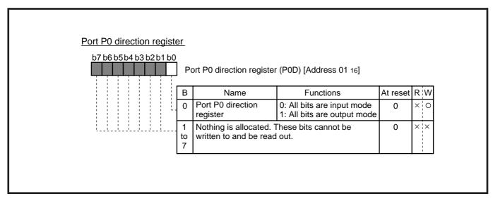
Fig. 2.7.4 Structure of port P0 direction register
