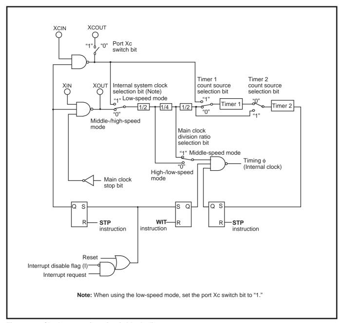
Fig. 2.10.3 Clock generating circuit block diagram
