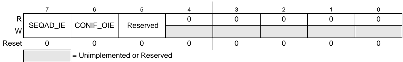
Figure 9-11. ADC Interrupt Enable Register (ADCIE)
