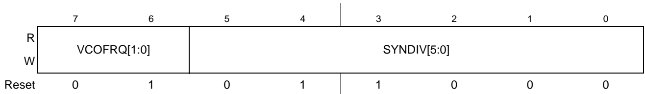
Figure 8-5. S12CPMU_UHV_V6 Synthesizer Register (CPMUSYNR)
