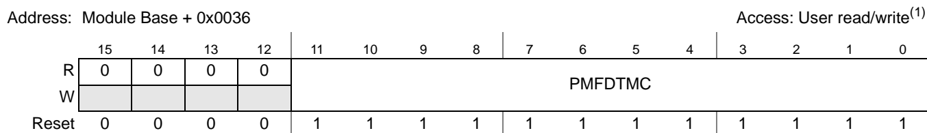
Figure 14-38. PMF Deadtime C Register (PMFDTMC)
