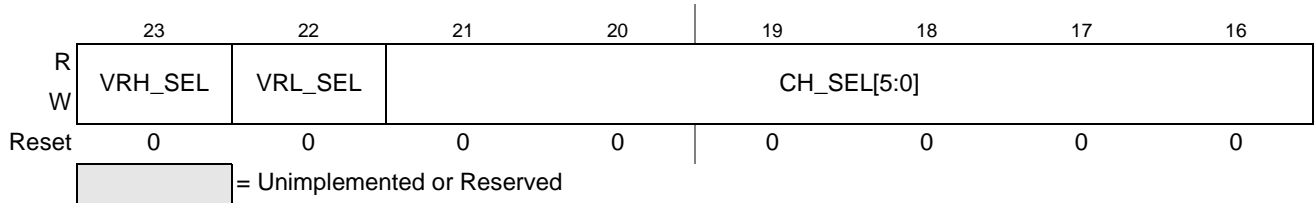
Figure 9-19. ADC Command Register 1 (ADCCMD_1)
