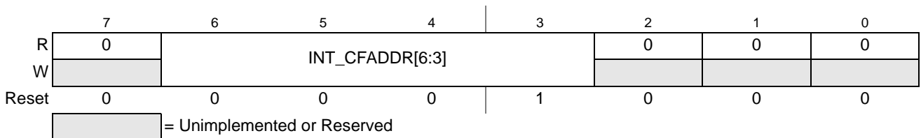
Figure 4-4. Interrupt Configuration Address Register (INT_CFADDR)
