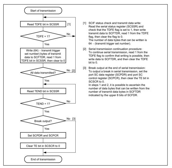
Figure 16.3 Sample Serial Transmission Flowchart
