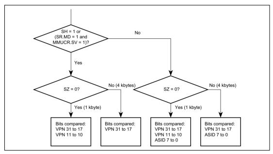
Figure 3.10 Objects of Address Comparison
