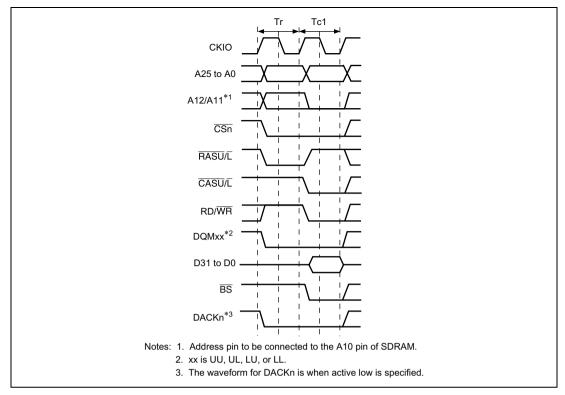
Figure 7.23 Single Write Timing (No Auto Precharge)
