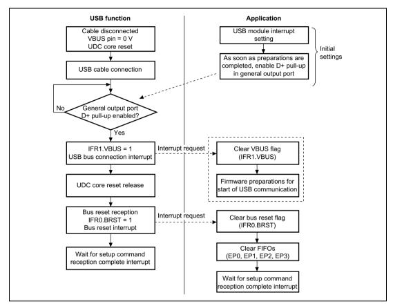
Figure 18.2 Cable Connection Operation
