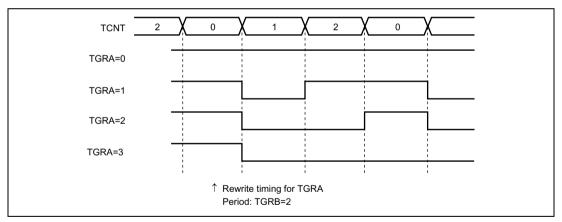
Figure 14.13 Examples of PWM Mode Operation (2)
