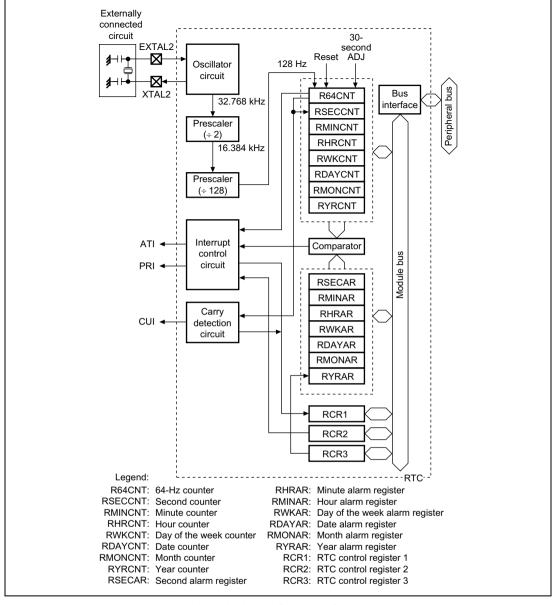
Figure 15.1 RTC Block Diagram
