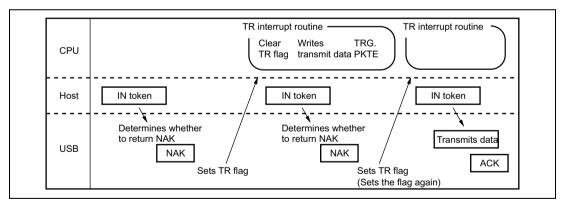
Figure 18.19 TR Interrupt Flag Set Timing
