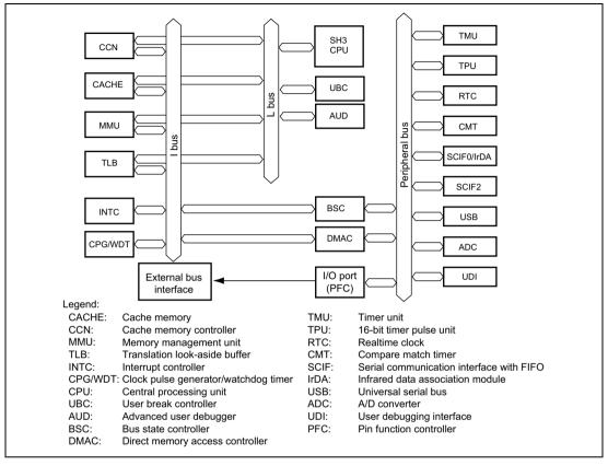
Figure 1.1 Block Diagram of SH7705
