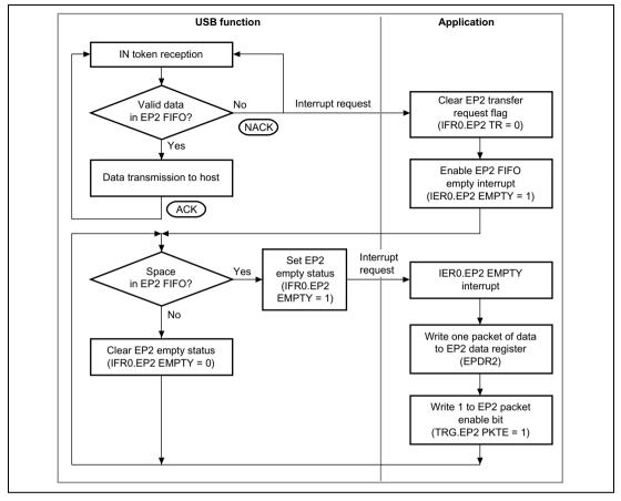
Figure 18.11 EP2 Bulk-In Transfer Operation
