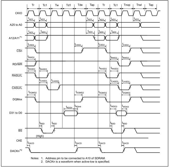
Figure 25.39 Access Timing in Low-Frequency Mode (Auto Precharge)
