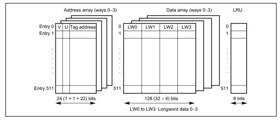
Figure 4.1 Cache Structure (32-kbyte Mode)
