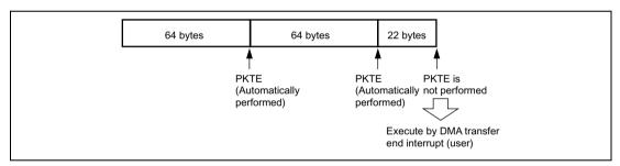
Figure 18.16 PKTE Bit Operation for EP2
