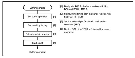
Figure 14.9 Example of Buffer Operation Setting Procedure
