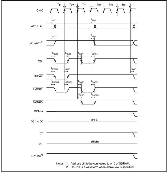
Figure 25.36 Synchronous DRAM Auto-Refresh Timing (TRP = 2 Cycle)
