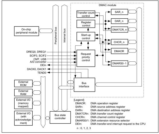
Figure 8.1 Block Diagram of DMAC
