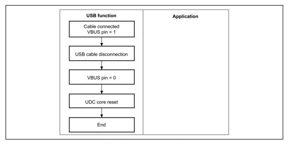
Figure 18.3 Cable Disconnection Operation
