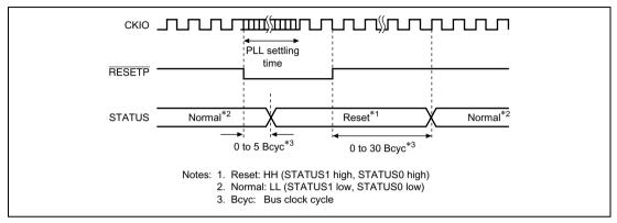
Figure 11.2 Power-On Reset STATUS Output
