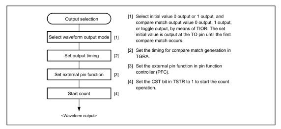
Figure 14.5 Example of Setting Procedure for Waveform Output by Compare Match
