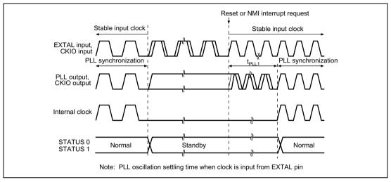
Figure 25.9 PLL Synchronization Settling Time by Reset or NMI
