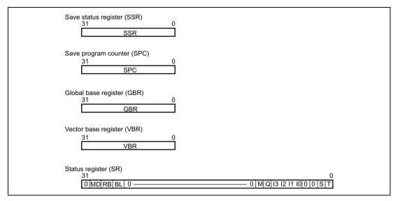
Figure 2.6 Control Register Configuration
