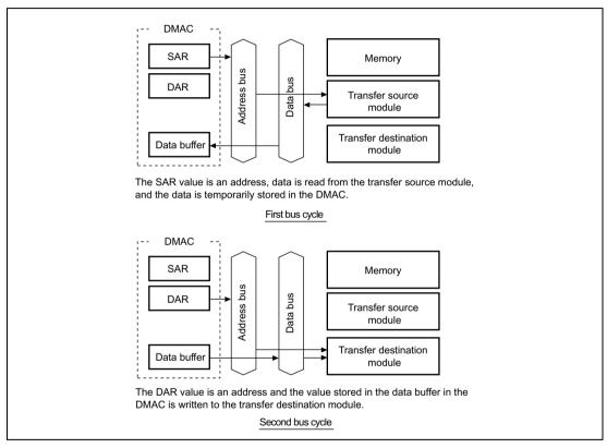
Figure 8.5 Data Flow of Dual Address Mode
