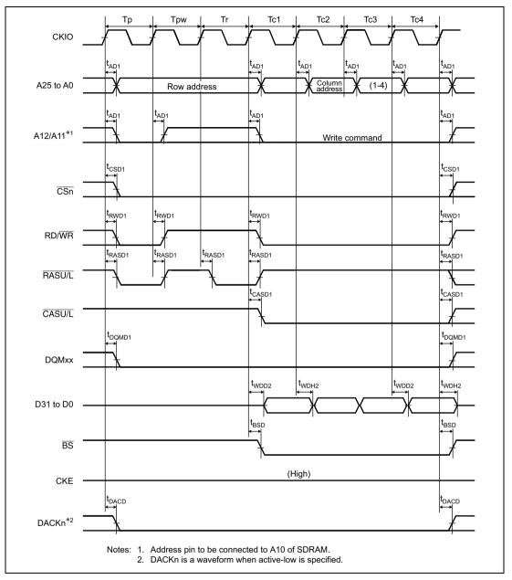
Figure 25.35 Synchronous DRAM Burst Write Bus Cycle (Single Write × 4)
