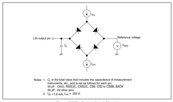
Figure 25.58 Output Load Circuit
