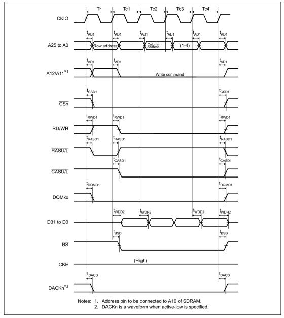
Figure 25.33 Synchronous DRAM Burst Write Bus Cycle (Single Write  $\times$  4) (Bank Active Mode: ACTV + WRITE Commands, TRCD = 1 Cycle, TRWL = 1 Cycle)
