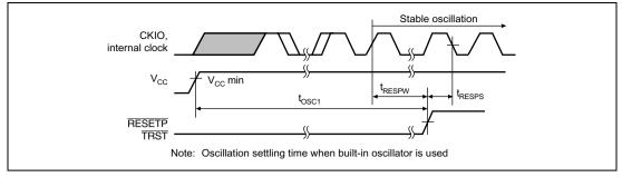
Figure 25.5 Power-On Oscillation Settling Time
