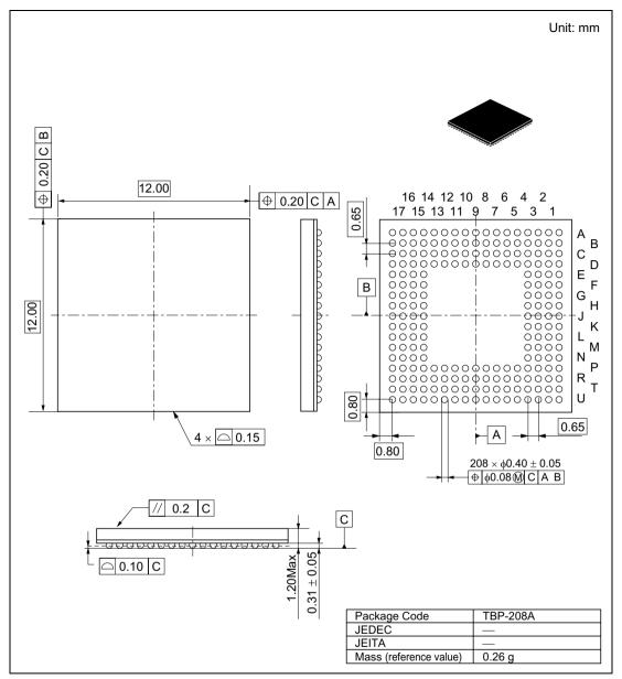
Figure B.2 Package Dimensions (TBP-208A)
