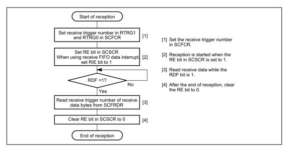
Figure 16.15 Sample Serial Reception Flowchart (1) (First Reception after Initialization)
