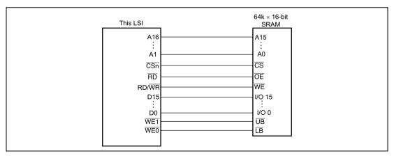
Figure 7.33 Example of Connection with 16-Bit Data-Width Byte-Selection SRAM
