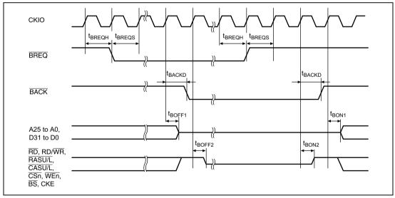
Figure 25.14 Bus Release Timing
