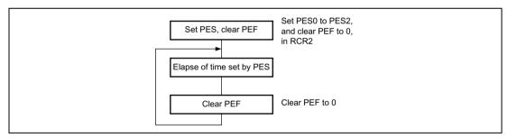
Figure 15.6 Using Periodic Interrupt Function
