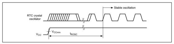
Figure 25.47 Oscillation Settling Time when RTC Crystal Oscillator Is Turned On
