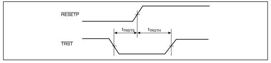
Figure 25.55 TRST Input Timing (Reset Hold)
