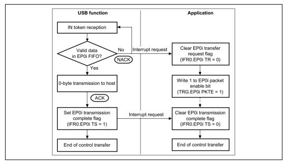
Figure 18.9 Status Stage (Control-Out) Operation
