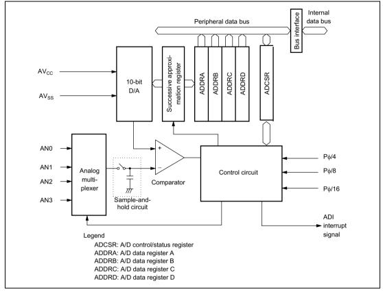
Figure 21.1 Block Diagram of A/D Converter
