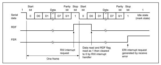
Figure 16.9 Example of SCIF Receive Operation (Example with 8-Bit Data, Parity, One Stop Bit)
