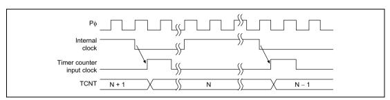
Figure 12.4 Count Timing when Internal Clock Is Operating
