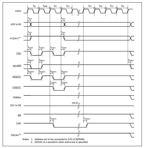
Figure 25.37 Synchronous DRAM Self-Refresh Timing (TRP = 2 Cycle)
