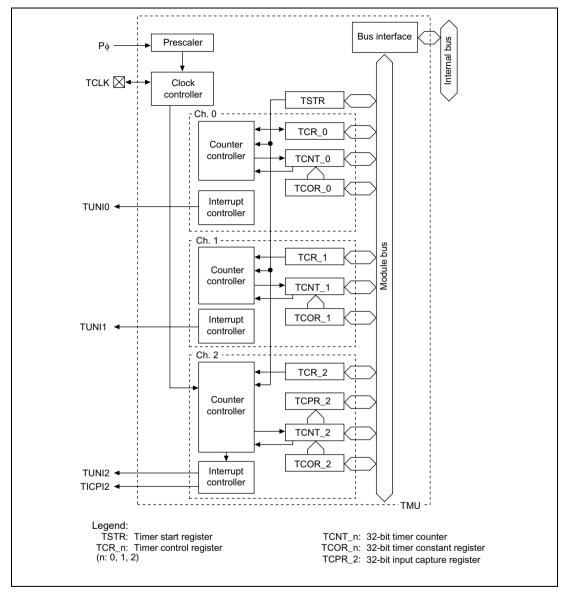
Figure 12.1 TMU Block Diagram
