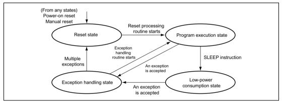
Figure 2.1 Processing State Transitions
