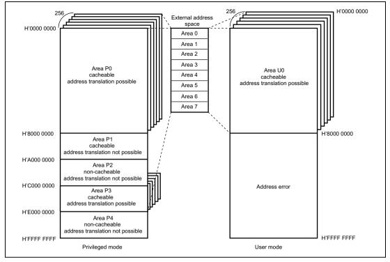
Figure 3.2 Virtual Address Space (MMUCR.AT = 1)
