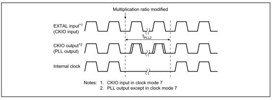
Figure 25.11 PLL Synchronization Settling Time when Frequency Multiplication Ratio Modified
