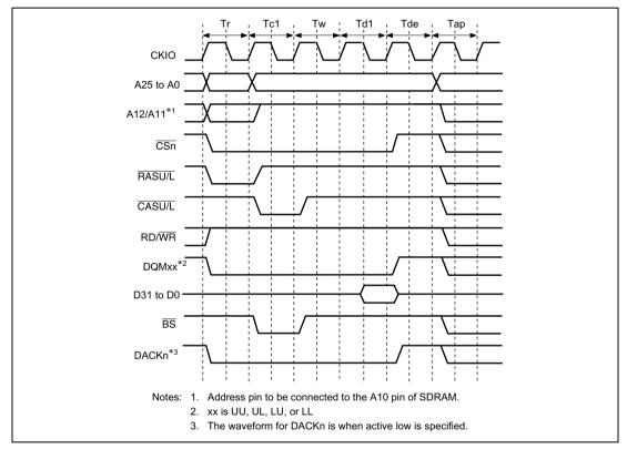
Figure 7.17 Basic Timing for Single Read (Auto Precharge)
