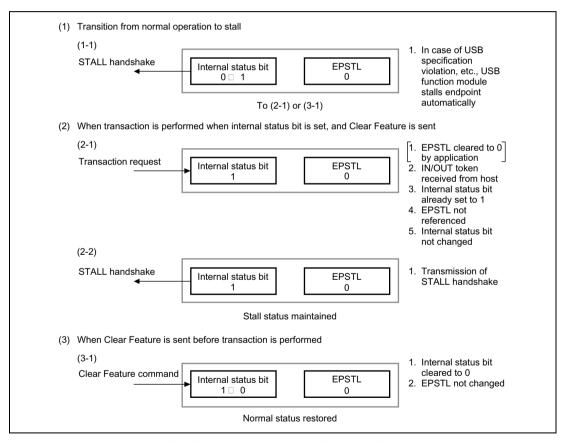
Figure 18.14 Automatic Stall by USB Function Module
