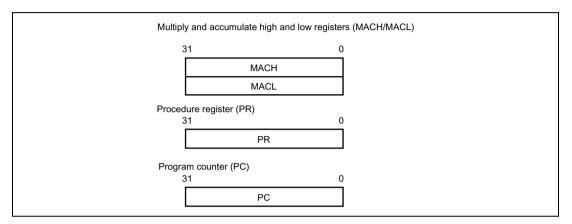
Figure 2.5 System Registers and Program Counter
