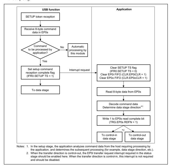
Figure 18.5 Setup Stage Operation
