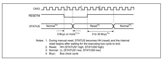
Figure 11.3 Manual Reset STATUS Output
