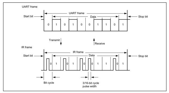
Figure 17.2 Transmit/Receive Operation
