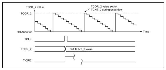
Figure 12.6 Operation Timing when Using Input Capture Function (Using TCLK Rising Edge)
