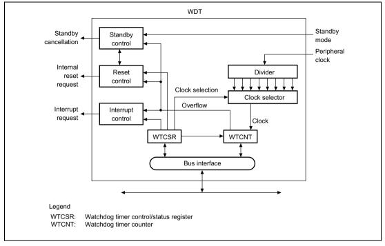
Figure 10.1 Block Diagram of WDT
