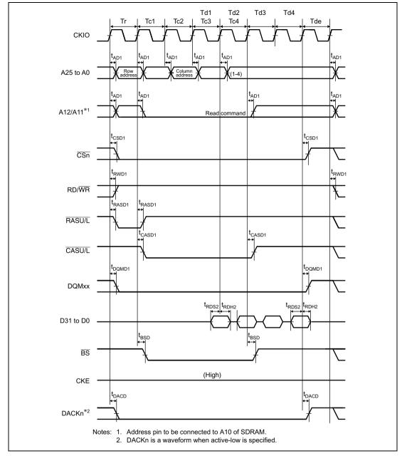
Figure 25.30 Synchronous DRAM Burst Read Bus Cycle (Single Read  $\times$  4) (Bank Active Mode: ACTV + READ Commands, CAS Latency = 2, TRCD = 1 Cycle)
