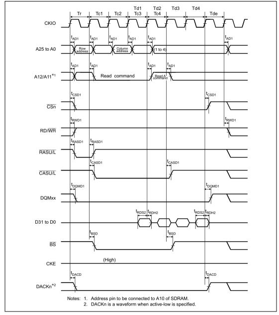
Figure 25.24 Synchronous DRAM Burst Read Bus Cycle (Single Read × 4), (Auto Precharge, CAS Latency = 2, TRCD = 1 Cycle, TRP = 2 Cycle)
