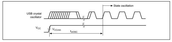
Figure 25.52 Oscillation Settling Time when USB Crystal Oscillator Is Turned On
