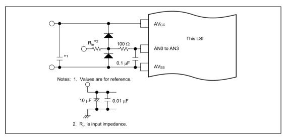
Figure 21.6 Example of Analog Input Protection Circuit
