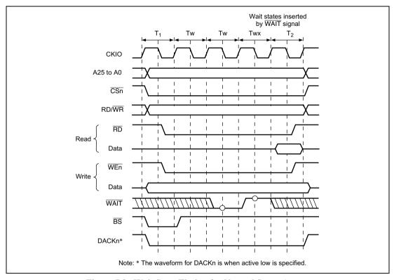
Figure 7.9 Wait State Timing for Normal Space Access (Wait State Insertion by WAIT Signal)
