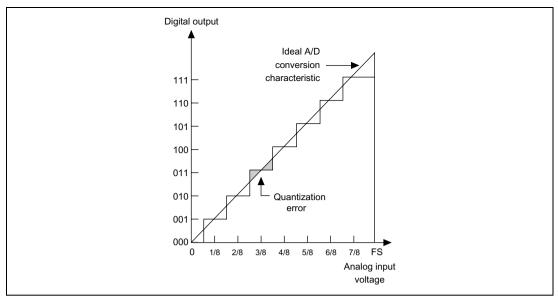
Figure 21.3 Definitions of A/D Conversion Accuracy
