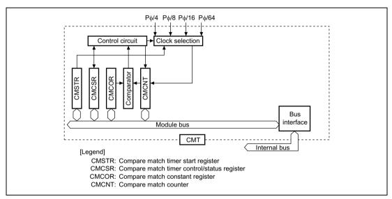
Figure 13.1 CMT Block Diagram
