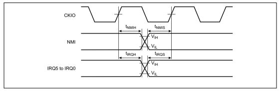
Figure 25.13 Interrupt Signal Input Timing
