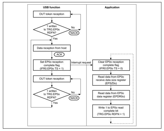
Figure 18.7 Data Stage (Control-Out) Operation
