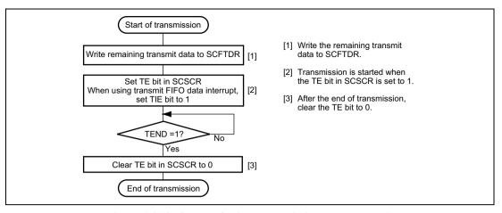
Figure 16.14 Sample Serial Transmission Flowchart (1) (First Transmission after Initialization)
