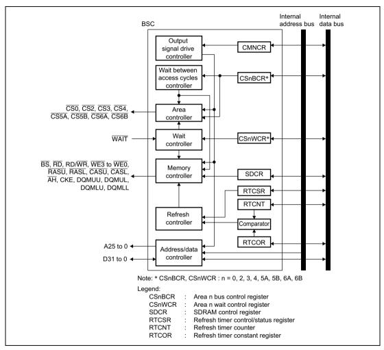
Figure 7.1 BSC Functional Block Diagram
