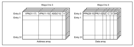
Figure 3.6 Overall Configuration of the TLB
