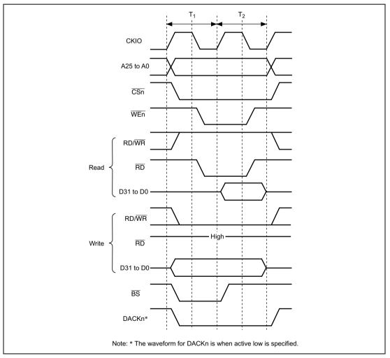
Figure 7.31 Byte-Selection SRAM Basic Access Timing
