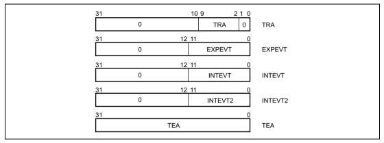
Figure 5.1 Register Bit Configuration
