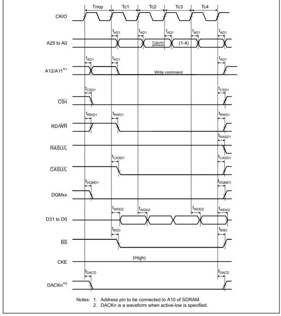
Figure 25.34 Synchronous DRAM Burst Write Bus Cycle (Single Write × 4) (Bank Active Mode: WRITE Command, Same Row Address, TRCD = 1 Cycle, TRWL = 1 Cycle)
