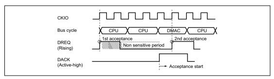
Figure 8.13 Example of DREQ Input Detection in Cycle Steal Mode Edge Detection
