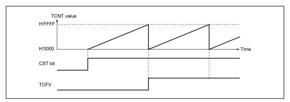
Figure 14.3 Free-Running Counter Operation
