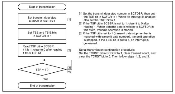
Figure 16.6 Transmit Data Stop Function Flowchart
