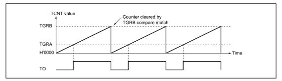
Figure 14.12 Example of PWM Mode Operation (1)
