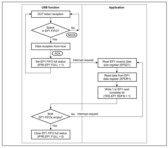
Figure 18.10 EP1 Bulk-Out Transfer Operation
