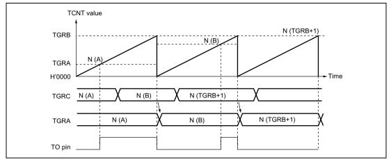
Figure 14.10 Example of Buffer Operation
