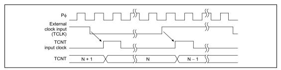
Figure 12.5 Count Timing when External Clock Is Operating (Both Edges Detected)
