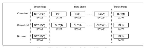
Figure 18.4 Transfer Stages in Control Transfer
