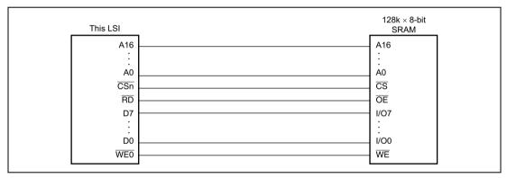
Figure 7.7 Example of 8-Bit Data-Width SRAM Connection
