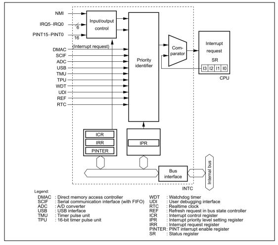
Figure 6.1 Block Diagram of INTC
