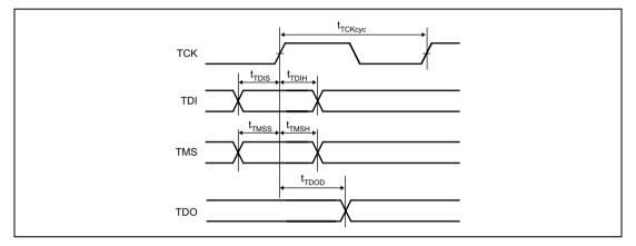
Figure 25.56 UDI Data Transfer Timing
