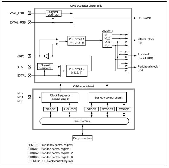
Figure 9.1 Block Diagram of Clock Pulse Generator
