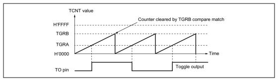
Figure 14.7 Example of Toggle Output Operation
