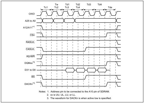
Figure 7.21 Burst Read Timing (Bank Active, Same Row Address)
