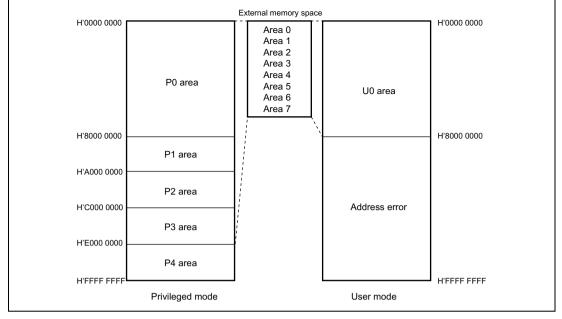
Figure 2.2 Logical Address to External Memory Space Mapping
