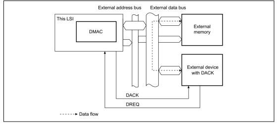
Figure 8.7 Data Flow in Single Address Mode
