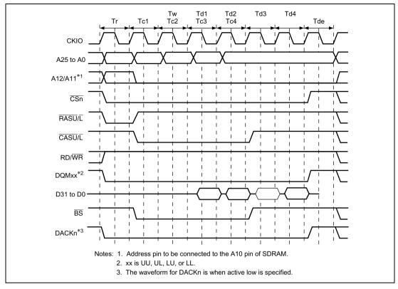
Figure 7.20 Burst Read Timing (No Auto Precharge)
