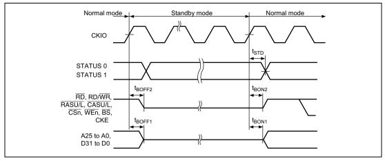
Figure 25.15 Pin Drive Timing at Standby
