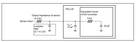
Figure 21.5 Analog Input Circuit Example
