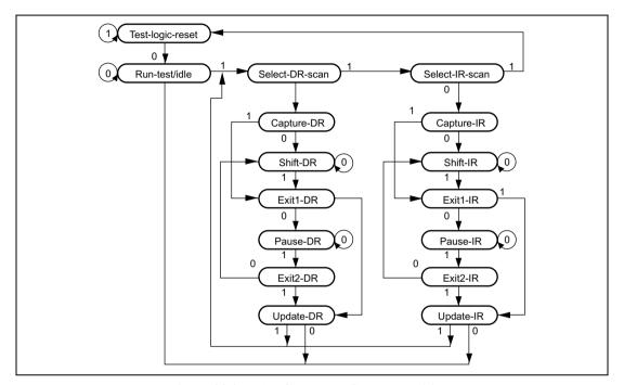
Figure 23.2 TAP Controller State Transitions
