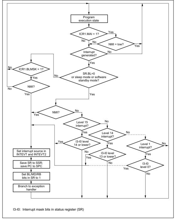
Figure 6.3 Interrupt Operation Flowchart
