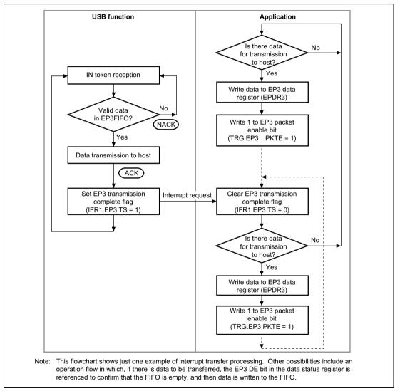
Figure 18.12 Operation of EP3 Interrupt-In Transfer
