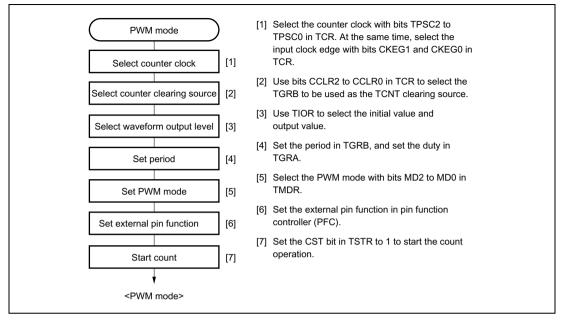
Figure 14.11 Example of PWM Mode Setting Procedure
