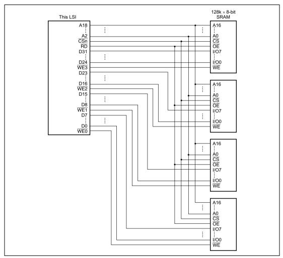
Figure 7.5 Example of 32-Bit Data-Width SRAM Connection
