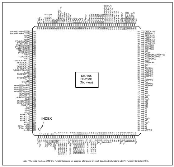
Figure 1.2 Pin Assignment (FP-208C)
