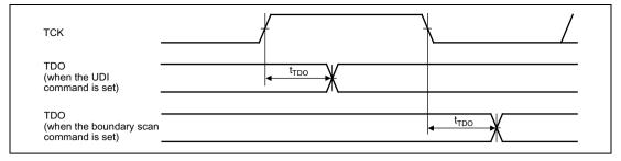
Figure 23.3 UDI Data Transfer Timing
