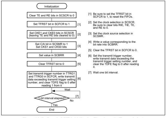
Figure 16.13 Sample SCIF Initialization Flowchart (1) (Transmission)
