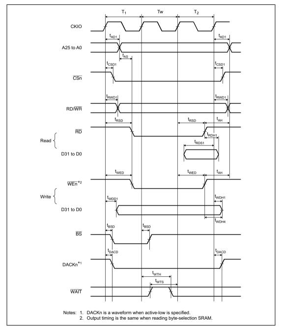
Figure 25.17 Basic Bus Cycle (One Software Wait)
