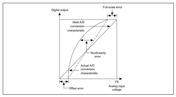
Figure 21.4 Definitions of A/D Conversion Accuracy
