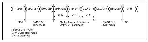
Figure 8.12 Bus State when Multiple Channels are Operating
