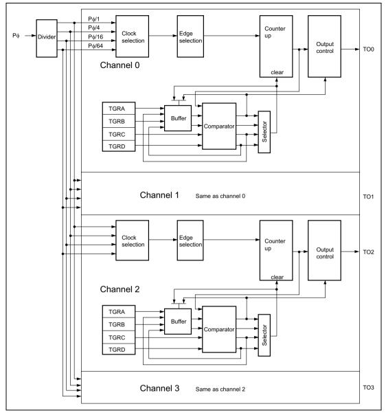
Figure 14.1 Block Diagram of TPU
