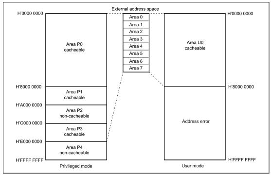
Figure 3.3 Virtual Address Space (MMUCR.AT = 0)
