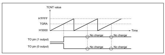
Figure 14.6 Example of 0 Output/1 Output Operation
