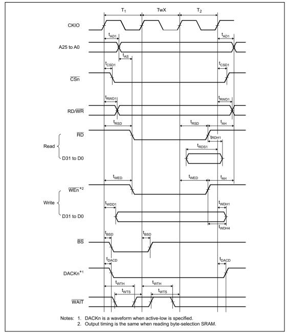
Figure 25.18 Basic Bus Cycle (One External Wait)
