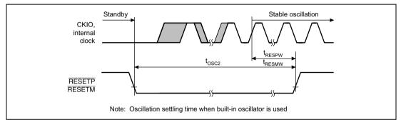
Figure 25.6 Oscillation Settling Time at Standby Return (Return by Reset)
