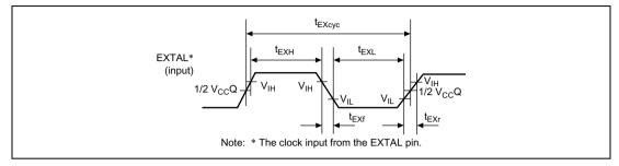
Figure 25.2 EXTAL Clock Input Timing
