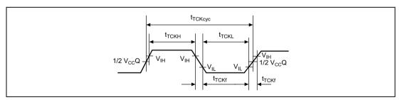
Figure 25.54 TCK Input Timing
