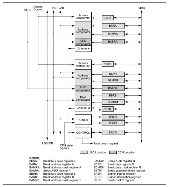
Figure 22.1 Block Diagram of User Break Controller
