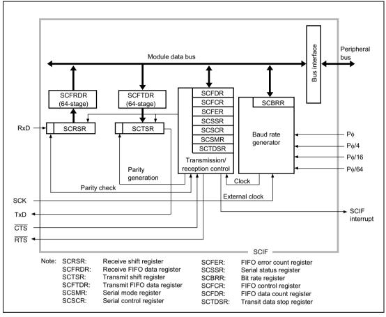
Figure 16.1 Block Diagram of SCIF
