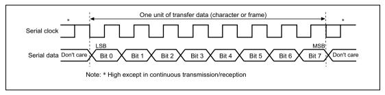
Figure 16.12 Data Format in Clock Synchronous Communication
