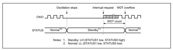
Figure 11.4 Canceling Software Standby by Interrupt STATUS Output
