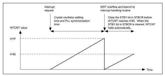
Figure 11.1 Canceling Standby Mode with STBY Bit in STBCR
