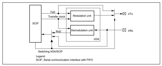
Figure 17.1 Block Diagram of IrDA
