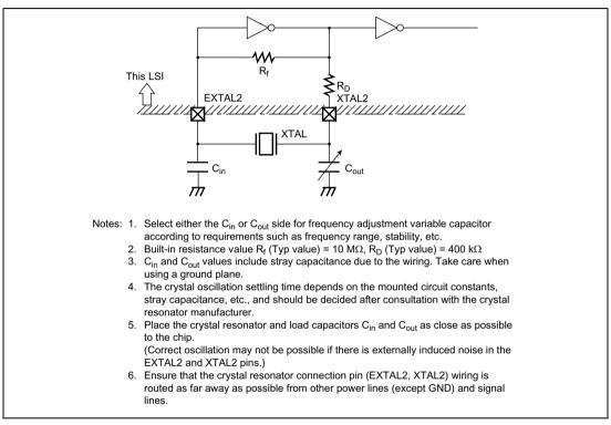
Figure 15.5 Example of Crystal Oscillator Circuit Connection
