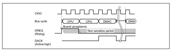
Figure 8.15 Example of DREQ Input Detection in Burst Mode Edge Detection
