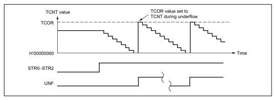
Figure 12.3 Auto-Reload Count Operation
