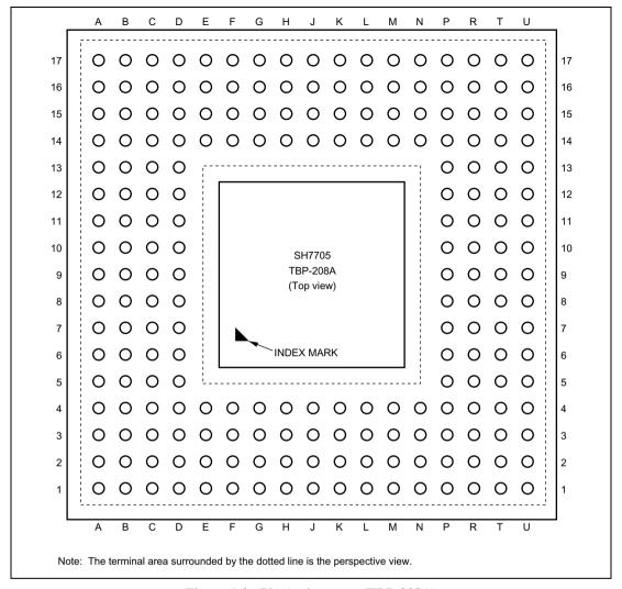
Figure 1.3 Pin Assignment (TBP-208A)
