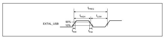
Figure 25.51 USB Clock Timing
