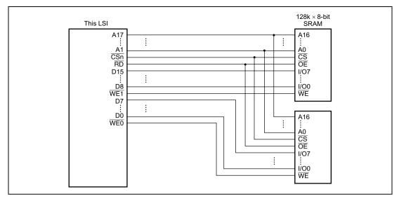
Figure 7.6 Example of 16-Bit Data-Width SRAM Connection
