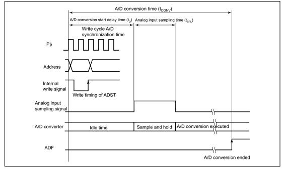
Figure 21.2 A/D Conversion Timing
