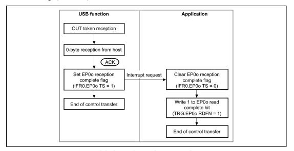
Figure 18.8 Status Stage (Control-In) Operation
