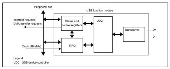
Figure 18.1 Block Diagram of USB
