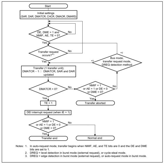
Figure 8.2 DMAC Transfer Flowchart
