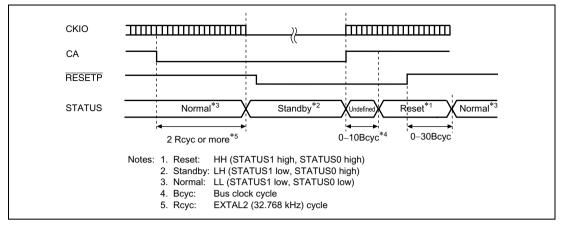
Figure 11.10 Hardware Standby Mode (When CA Goes Low in Normal Operation)
