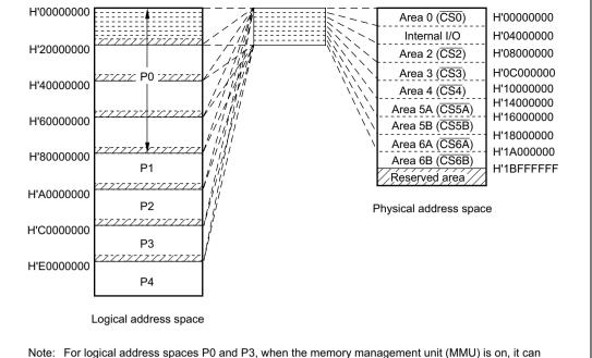
Note: For logical address spaces P0 and P3, when the memory management unit (MMU) is on, it can optionally generate a physical address for the logical address. This figure can be applied when MMU is off and when the MMU is on and each physical address for the logical address is equal except for higher three bits. When translating a logical address to a physical address, refer to table 7.2
