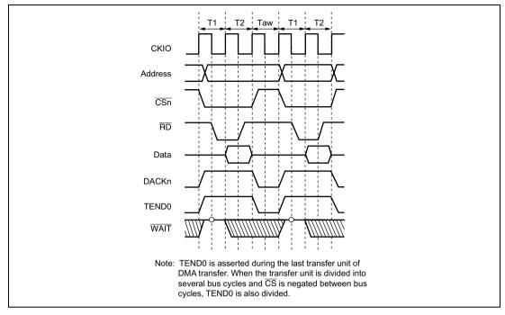
Figure 8.18 BSC Ordinary Memory Access (No Wait, Idle Cycle 1, Longword Access to 16-Bit Device)
