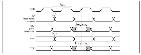
Figure 25.50 SCIF Input/Output Timing in Clock Synchronous Mode
