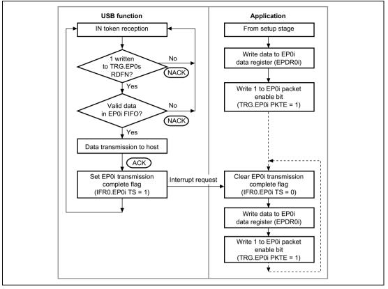
Figure 18.6 Data Stage (Control-In) Operation
