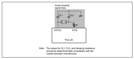
Figure 9.2 Points for Attention when Using Crystal Resonator
