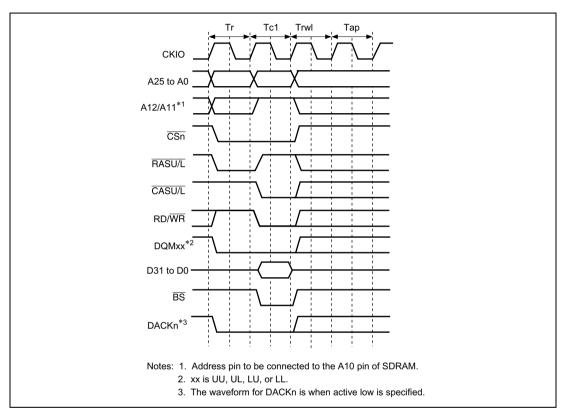
Figure 7.19 Basic Timing for Single Write (Auto Precharge)
