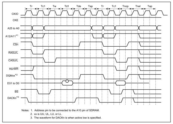
Figure 7.28 Low-Frequency Mode Access Timing
