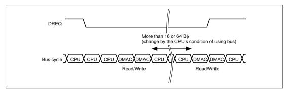
Figure 8.10 Example of DMA Transfer in Cycle Steal Intermittent Mode (Dual Address, DREQ Low Level Detection)
