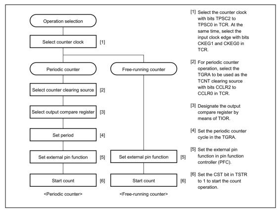
Figure 14.2 Example of Counter Operation Setting Procedure
