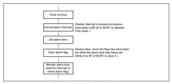
Figure 15.4 Using the Alarm Function
