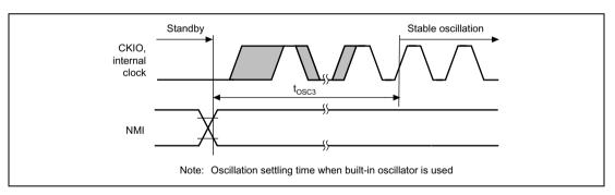
Figure 25.7 Oscillation Settling Time at Standby Return (Return by NMI)
