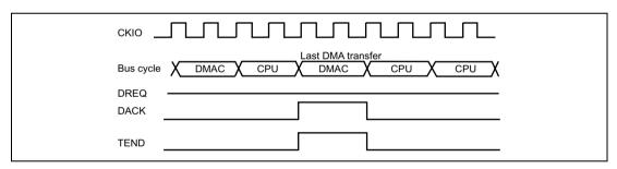
Figure 8.17 Example of DMA Transfer End Signal (in Cycle Steal Level Detection)
