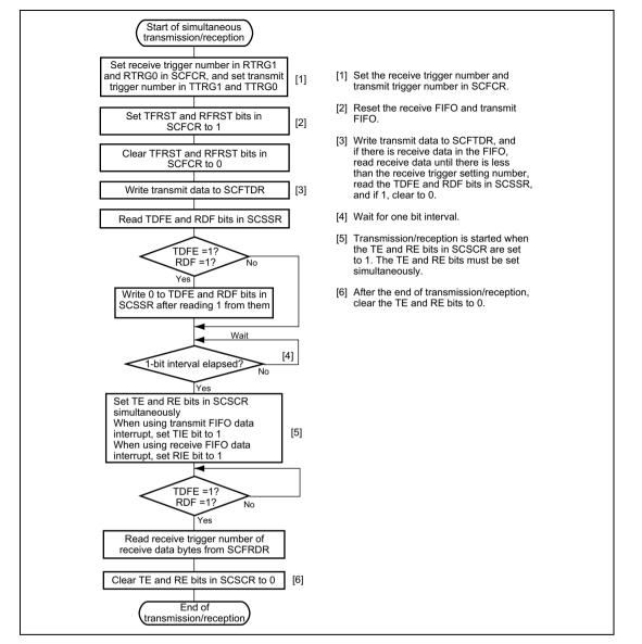
Figure 16.16 Sample Simultaneous Serial Transmission and Reception Flowchart (2) (Second and Subsequent Transfer)
