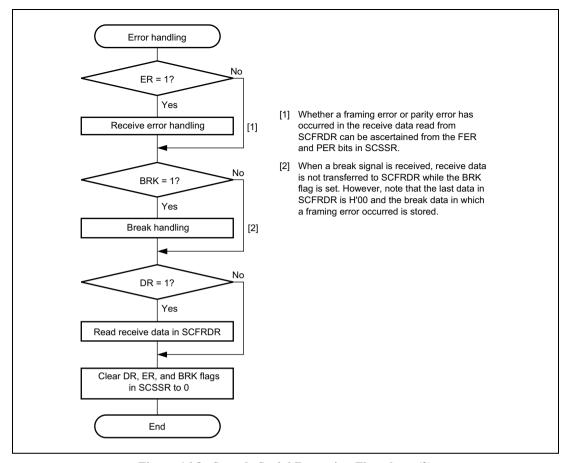
Figure 16.8 Sample Serial Reception Flowchart (2)
