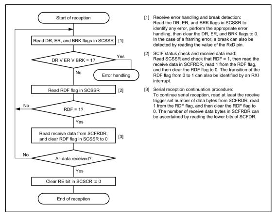
Figure 16.7 Sample Serial Reception Flowchart (1)
