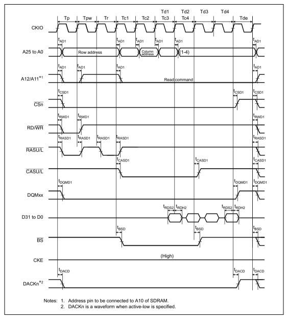
Figure 25.32 Synchronous DRAM Burst Read Bus Cycle (Single Read × 4)
