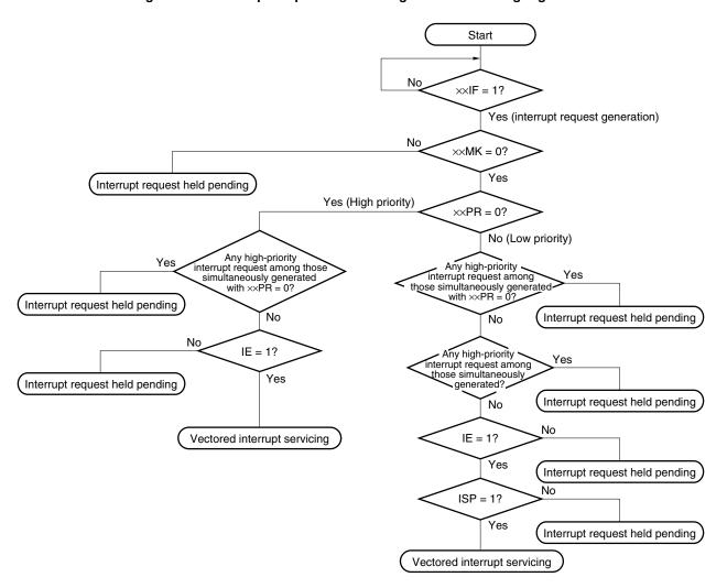
Figure 19-7. Interrupt Request Acknowledgement Processing Algorithm
