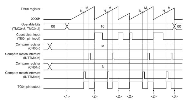
Figure 7-36. Example of Software Processing in Clear & Start Mode Entered by TI00n Pin Valid Edge Input
