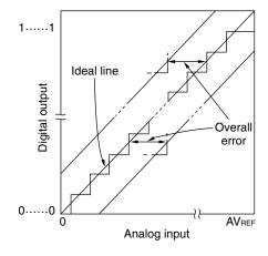
Figure 13-15. Quantization Error
