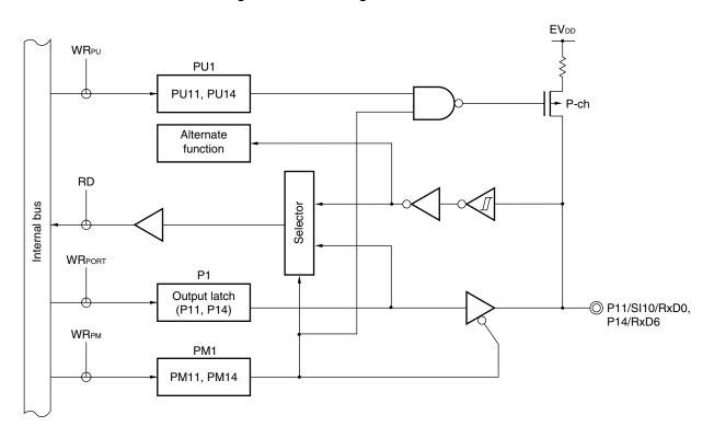
Figure 5-9. Block Diagram of P11 and P14
