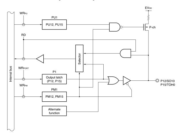
Figure 5-10. Block Diagram of P12 and P15
