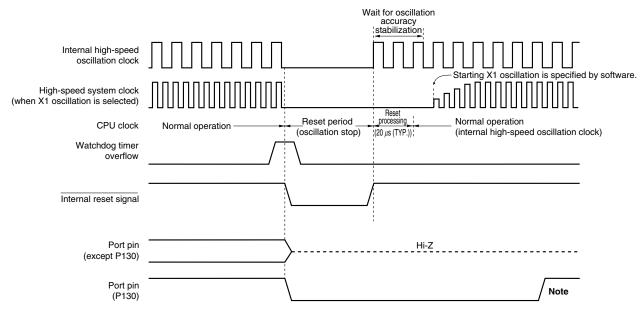
Note Set P130 to high-level output by software.
