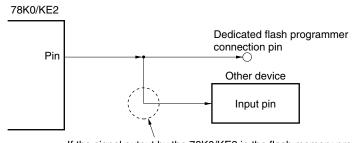
If the signal output by the 78K0/KE2 in the flash memory programming mode affects the other device, isolate the signal of the other device.
