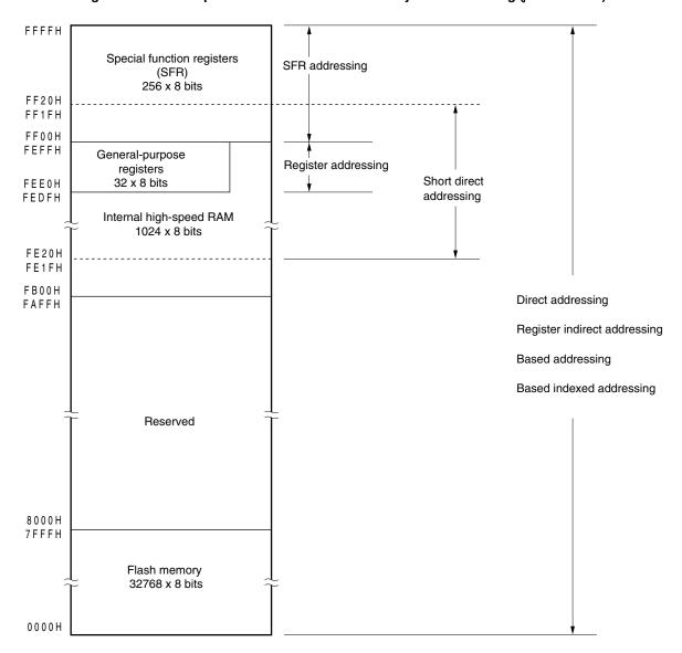
Figure 3-11. Correspondence Between Data Memory and Addressing (μPD78F0533)
