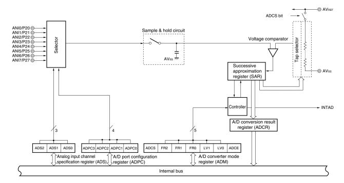
Figure 13-1. Block Diagram of A/D Converter
