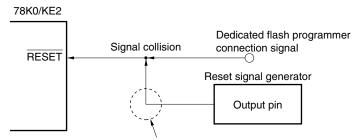
In the flash memory programming mode, the signal output by the reset signal generator collides with the signal output by the dedicated flash programmer. Therefore, isolate the signal of the reset signal generator.
