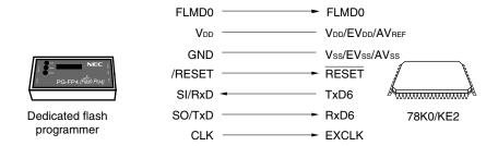
If FlashPro4 is used as the dedicated flash programmer, FlashPro4 generates the following signal for the 78K0/KE2. For details, refer to the FlashPro4 manual.
