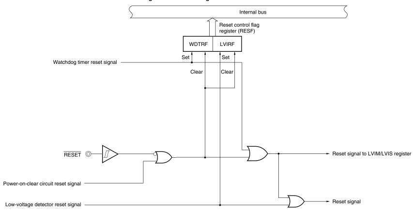
Figure 22-1. Block Diagram of Reset Function
