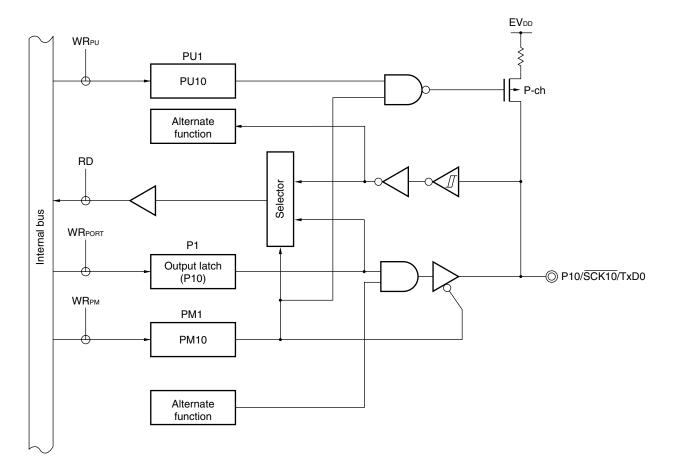
Figure 5-8. Block Diagram of P10
