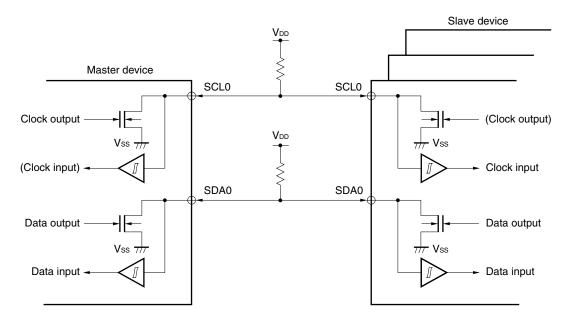
Figure 17-11. Pin Configuration Diagram
