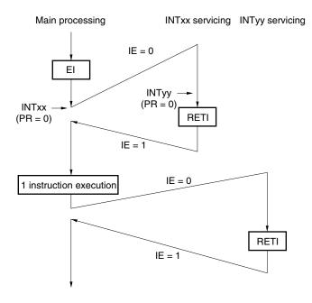
Interrupts are not enabled during servicing of interrupt INTxx (EI instruction is not issued), therefore, interrupt request INTyy is not acknowledged and multiple interrupt servicing does not take place. The INTyy interrupt request is held pending, and is acknowledged following execution of one main processing instruction.
