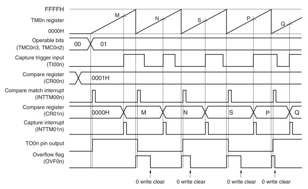
This is an application example where a compare register and a capture register are used at the same time in the free-running timer mode.
