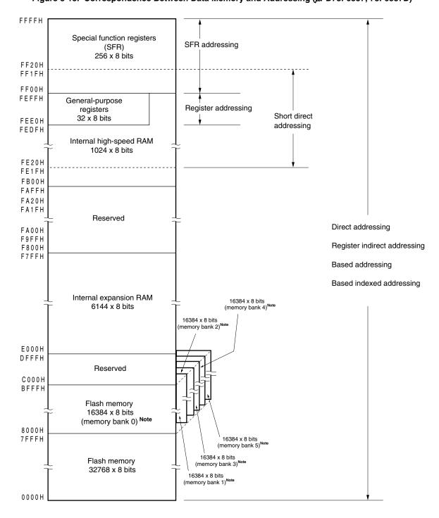
Figure 3-15. Correspondence Between Data Memory and Addressing (µPD78F0537, 78F0537D)
