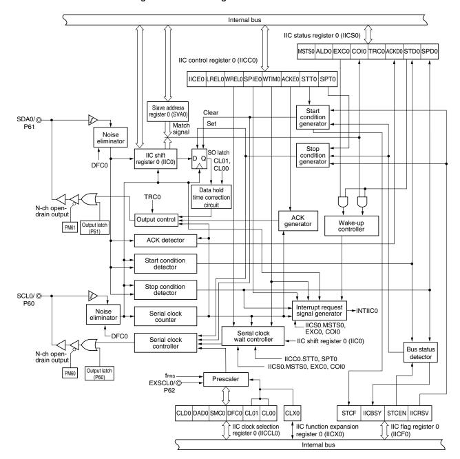
Figure 17-1. Block Diagram of Serial Interface IIC0
