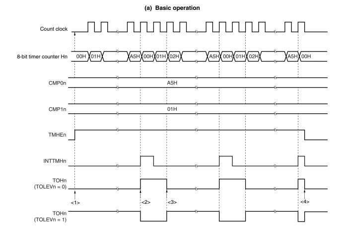
Figure 9-12. Operation Timing in PWM Output Mode (1/4)
