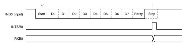
Figure 14-9. Reception Completion Interrupt Request Timing
