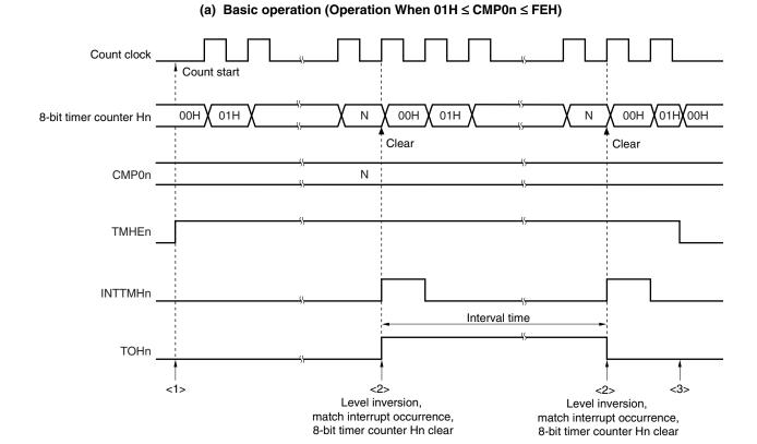
Figure 9-10. Timing of Interval Timer/Square-Wave Output Operation (1/2)
