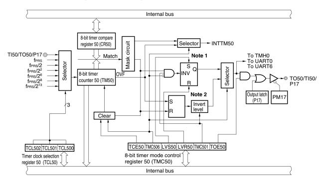
Figure 8-1. Block Diagram of 8-Bit Timer/Event Counter 50
