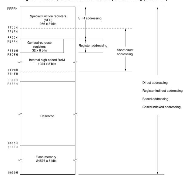
Figure 3-10. Correspondence Between Data Memory and Addressing (µPD78F0532)
