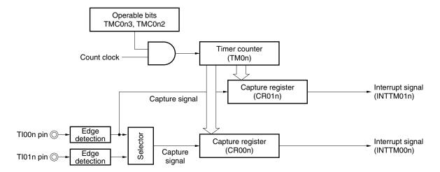
**Remarks 1.** If both CR00n and CR01n are used as capture registers in the free-running timer mode, the output level of the TO0n pin is not inverted.
