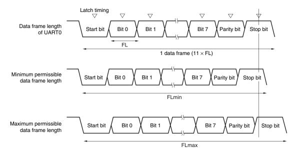
Figure 14-12. Permissible Baud Rate Range During Reception
