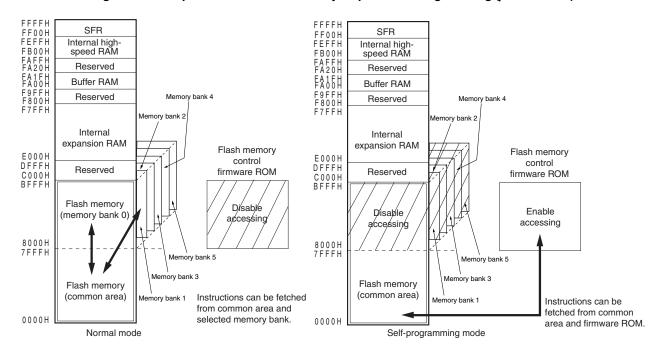
Figure 26-15. Operation Mode and Memory Map for Self-Programming (µPD78F0537)
