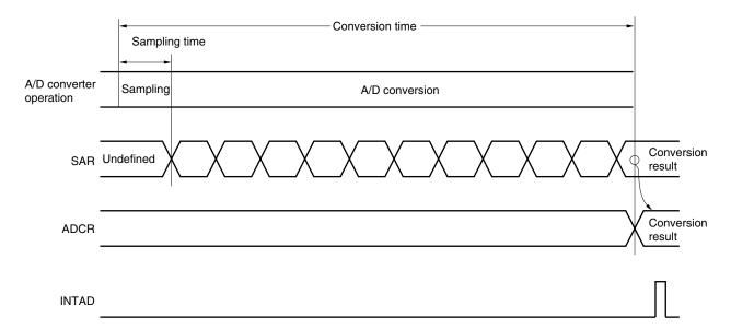
Figure 13-11. Basic Operation of A/D Converter
