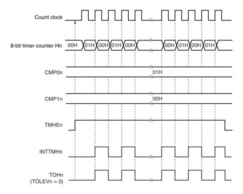
Figure 9-12. Operation Timing in PWM Output Mode (4/4)
