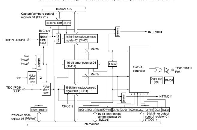
Figure 7-2. Block Diagram of 16-Bit Timer/Event Counter 01 (Available only in the  $\mu$ PD78F0534, 78F0535, 78F0536, 78F0537, and 78F0537D)
