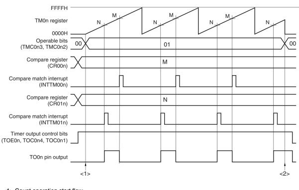
Figure 7-44. Example of Software Processing in Free-Running Timer Mode
