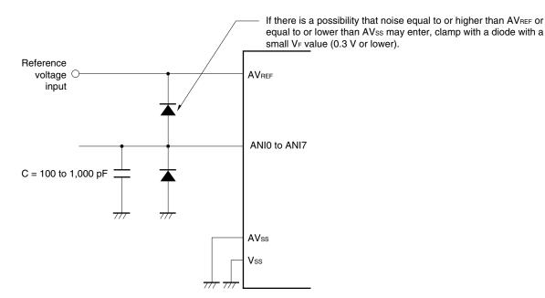
Figure 13-20. Analog Input Pin Connection
