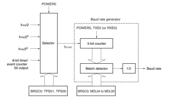
Figure 14-11. Configuration of Baud Rate Generator
