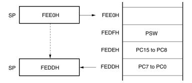
Figure 3-20. Data to Be Restored from Stack Memory
