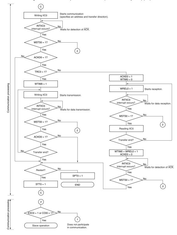
Figure 17-24. Master Operation Flowchart (Multi-Master System) (3/3)
