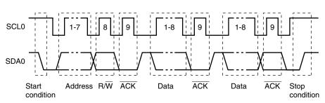
Figure 17-12. I<sup>2</sup>C Bus Serial Data Transfer Timing
