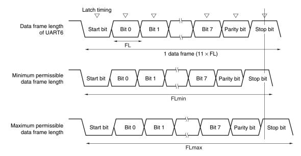
Figure 15-25. Permissible Baud Rate Range During Reception
