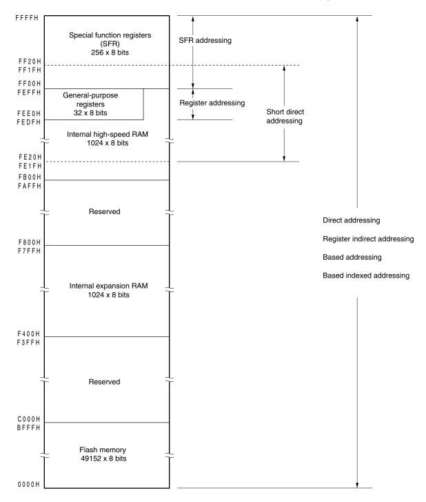
Figure 3-12. Correspondence Between Data Memory and Addressing (µPD78F0534)
