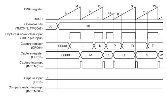
This is an application example where the pulse width of the signal input to the TI00n pin is measured.
