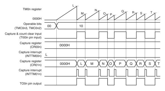
This is an application example where the count value is captured to CR01n, TM0n is cleared, and the TO0n pin output is inverted when the rising or falling edge of the Tl00n pin is detected.
