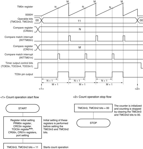
Figure 7-47. Example of Software Processing for PPG Output Operation
