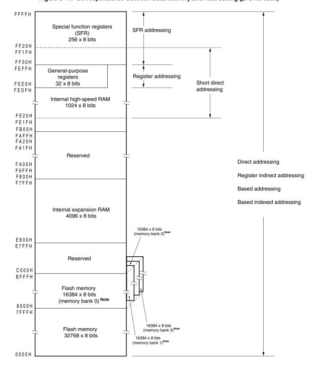
Figure 3-14. Correspondence Between Data Memory and Addressing (µPD78F0536)
