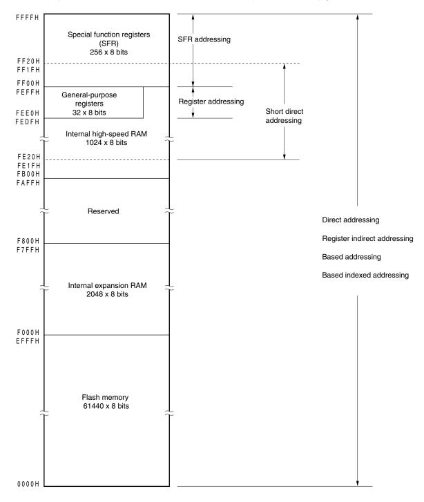
Figure 3-13. Correspondence Between Data Memory and Addressing (μPD78F0535)
