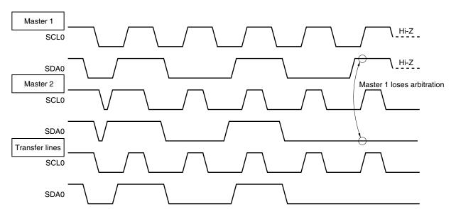
Figure 17-19. Arbitration Timing Example
