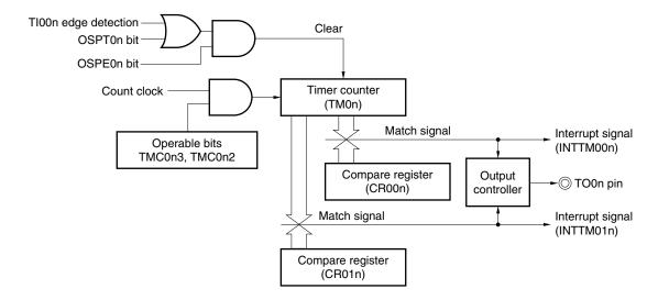
Figure 7-48. Block Diagram of One-Shot Pulse Output Operation
