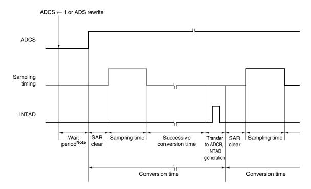
Figure 13-5. A/D Converter Sampling and A/D Conversion Timing
