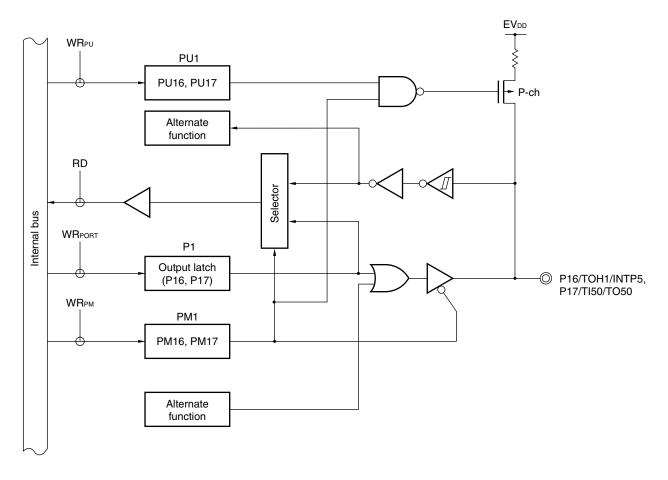
Figure 5-12. Block Diagram of P16 and P17
