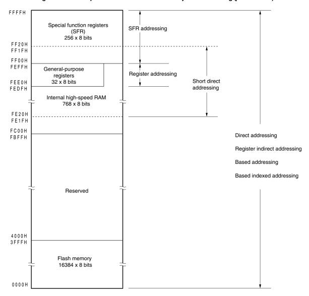
Figure 3-9. Correspondence Between Data Memory and Addressing (µPD78F0531)
