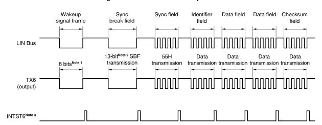
Figure 15-1. LIN Transmission Operation
