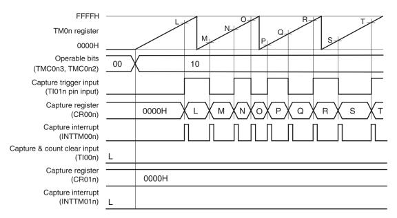
This is a timing example where an edge is not input to the TI00n pin, in an application where the count value is captured to CR00n when the rising or falling edge of the TI01n pin is detected.
