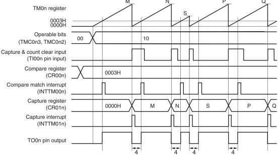
This is an application example where the width set to CR00n (4 clocks in this example) is to be output from the TO0n pin when the count value has been captured & cleared.
