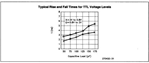
Figure 48. TTL Level Slew Rates for Output Buffers
