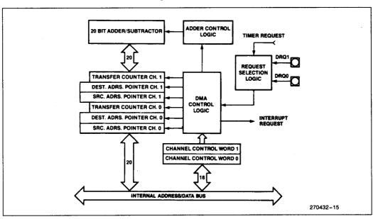
Figure 16. DMA Unit Block Diagram
