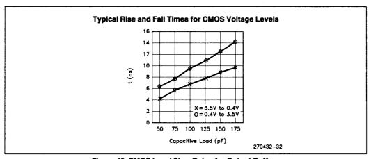
Figure 49. CMOS Level Slew Rates for Output Buffers
