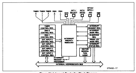
Figure 21. Interrupt Controller Block Diagram
