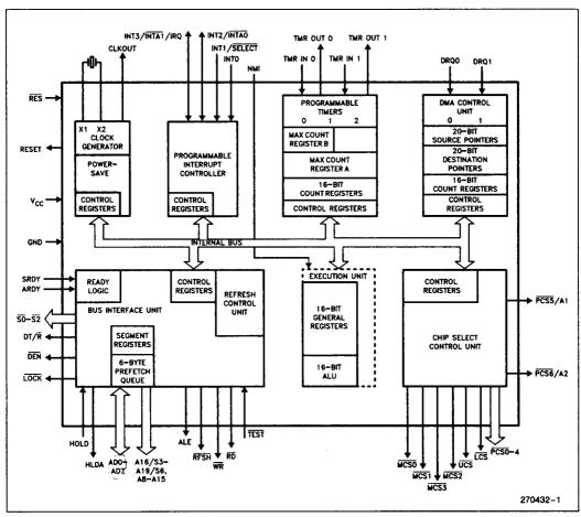
Figure 1. 80C188 Block Diagram
