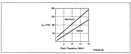
Figure 46. I<sub>CC</sub> vs Frequency
