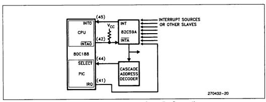
Figure 33. Slave Mode Interrupt Controller Connections
