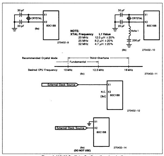
Figure 8. 80C188 Oscillator Configurations (see text)
