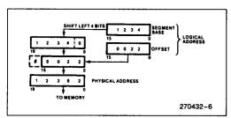
Figure 5. Two Component Address
