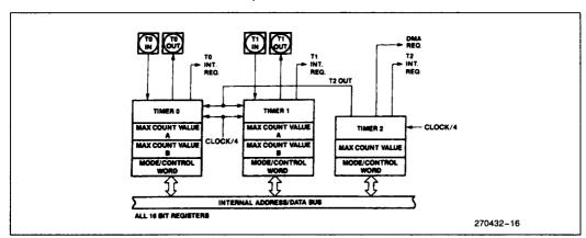
Figure 19. Timer Block Diagram
