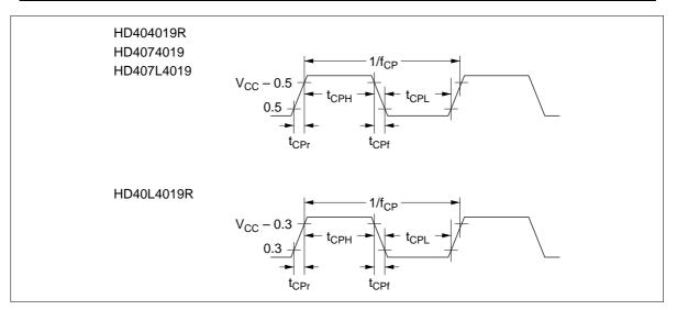
Figure 26 Oscillator Timing
