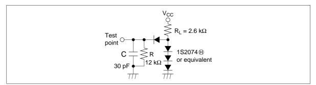
Figure 30 Timing Load Circuit
