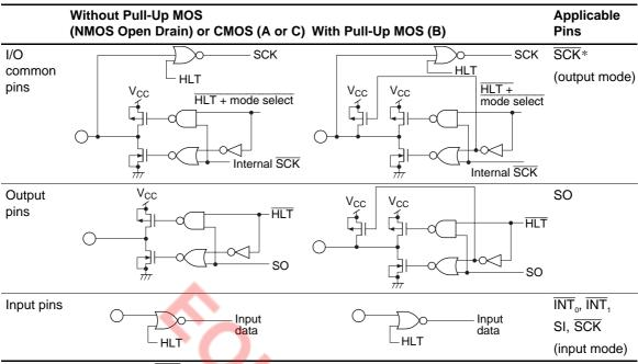
Notes: In the stop mode, HLT is 0, HLT is 1 and I/O pins are in high impedance. \* If the MCU is interrupted by the serial interface in the external clock input mode, the SCK terminal becomes input only.
