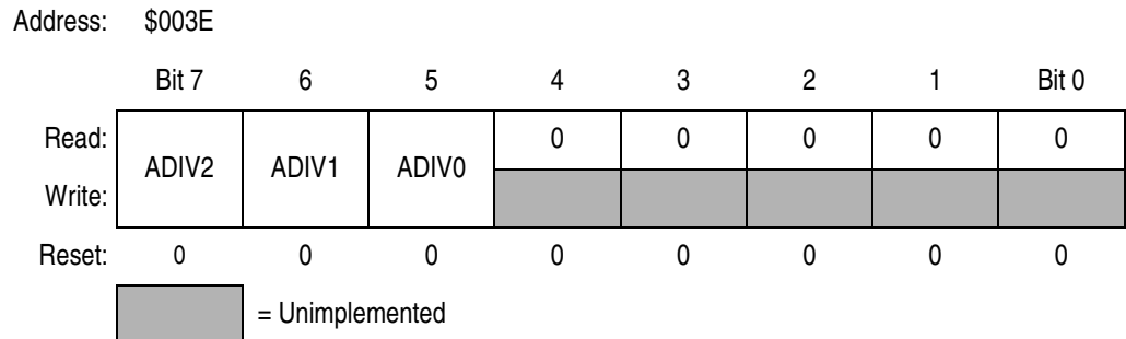
Figure 11-5. ADC Input Clock Register (ADICLK)
