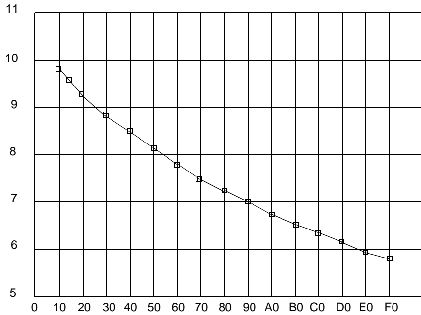
Figure 14. Typical Relaxation Oscillator Frequency vs. Trim Value @ 25°C
