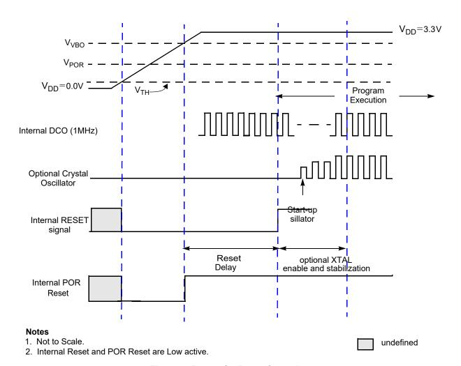
Figure 4. Power-On Reset Operations
