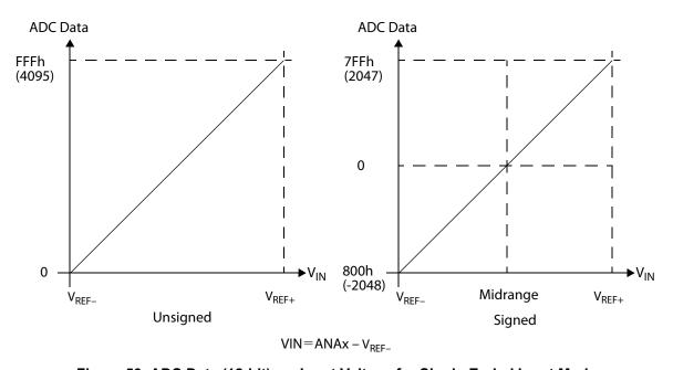
Figure 53. ADC Data (12-bit) vs. Input Voltage for Single-Ended Input Mode
