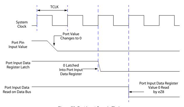
Figure 72. Port Input Sample Timing
