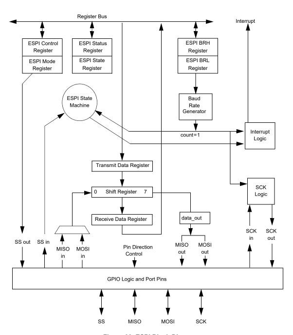
Figure 33. ESPI Block Diagram
