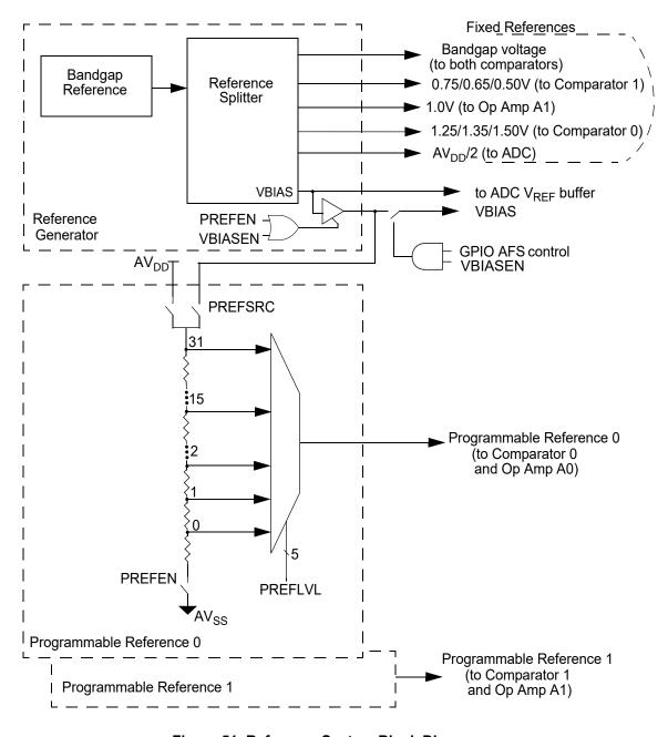
Figure 51. Reference System Block Diagram
