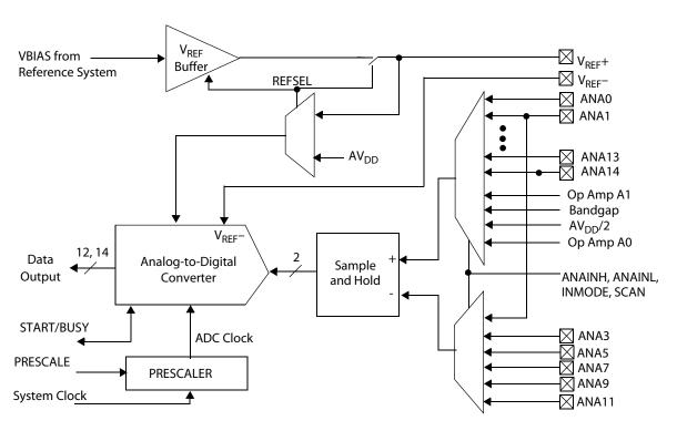
Figure 52. Analog-to-Digital Converter Block Diagram
