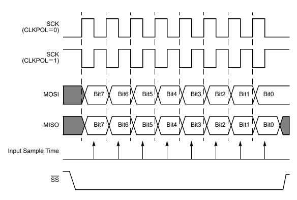
Figure 35. ESPI Timing when PHASE=1
