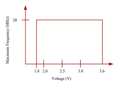
Figure 71. Maximum System Clock Frequency vs.  $\mathbf{V}_{\mathrm{DD}}$
