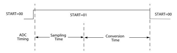
Figure 55. ADC Conversion Timing Diagram
