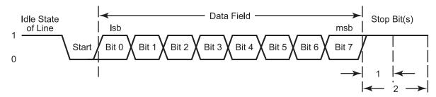
Figure 24. UART-LDD Asynchronous Data Format without Parity
