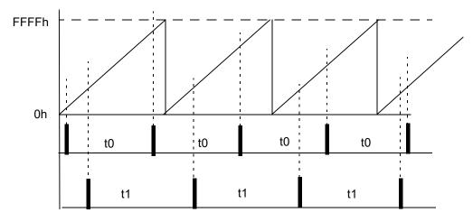
Figure 22. Count Max Mode with Channel Compare
