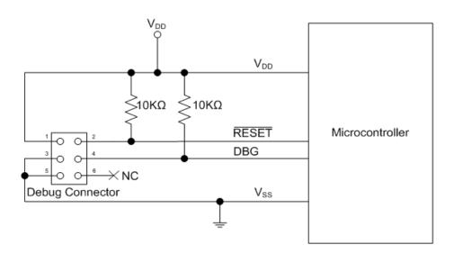
Figure 66. Target OCD Connector Interface
