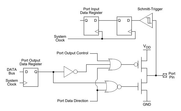
Figure 8. GPIO Port Pin Block Diagram
