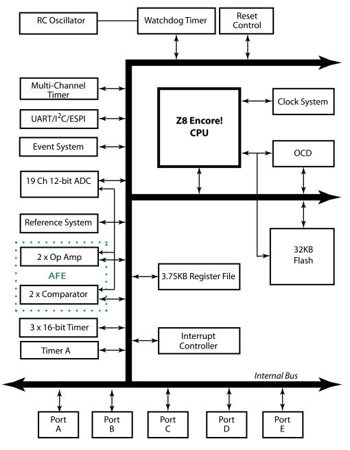
Figure 1. F3224 Series Block Diagram
