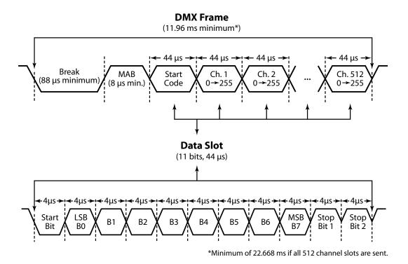
Figure 29. UART-LDD DMX Frame and Data Slot
