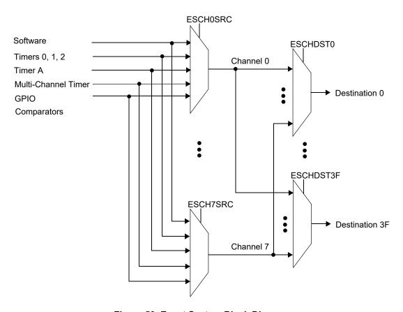
Figure 50. Event System Block Diagram
