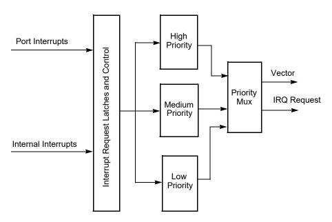
Figure 12. Interrupt Controller Block Diagram
