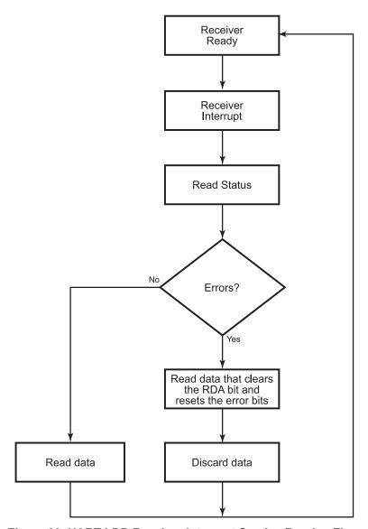
Figure 30. UART-LDD Receiver Interrupt Service Routine Flow
