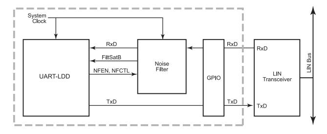
Figure 31. Noise Filter System Block Diagram
