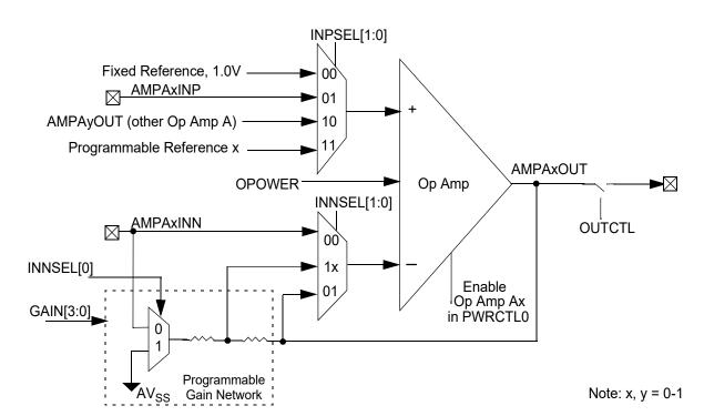
Figure 60. Op Amp A Block Diagram
