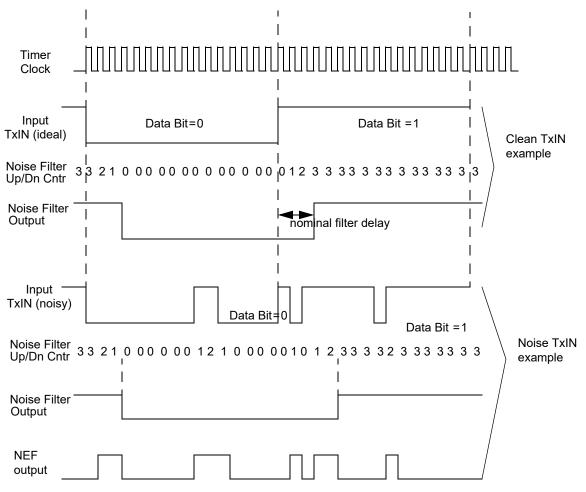
Figure 16. Noise Filter Operation
