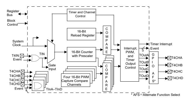
Figure 18. Multi-Channel Timer Block Diagram
