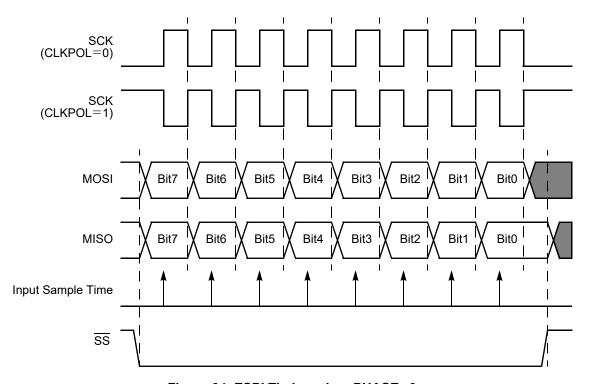
Figure 34. ESPI Timing when PHASE=0
