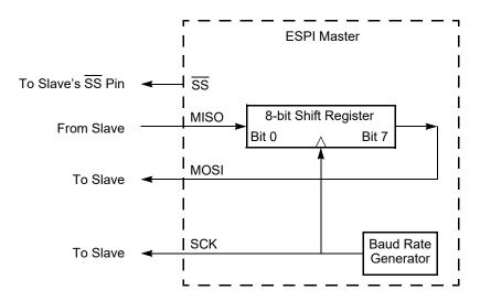
Figure 38. ESPI Configured as an SPI Master in a Single Master, Single Slave System
