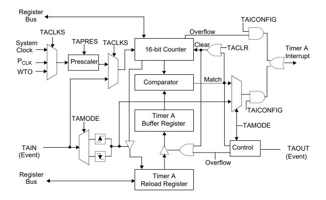
Figure 17. Timer A Block Diagram
