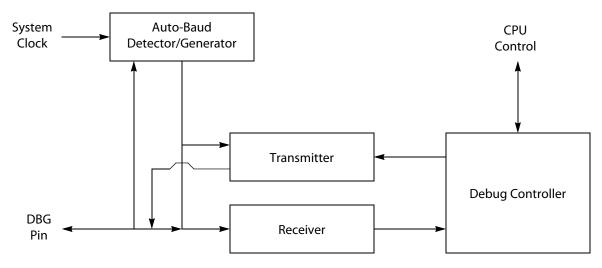
Figure 64. On-Chip Debugger Block Diagram
