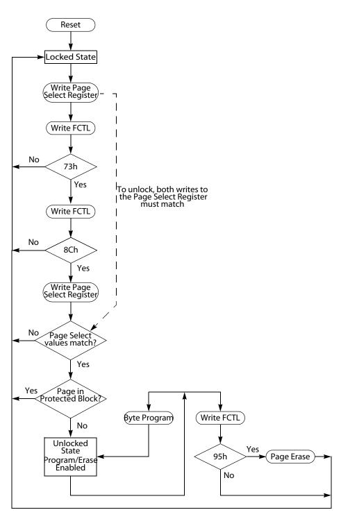
Figure 63. Flash Controller Operation Flowchart
