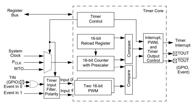
Figure 13. Timer Block Diagram
