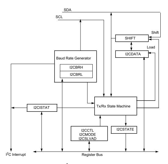
Figure 41. I<sup>2</sup>C Controller Block Diagram
