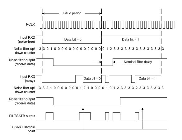
Figure 32. Noise Filter Operation
