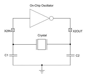
Figure 10. Recommended 32.768 kHz Crystal Oscillator Configuration
