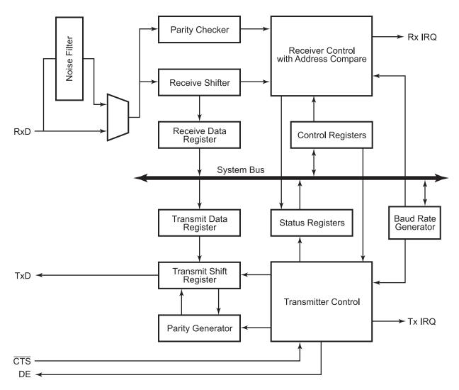
Figure 23. UART-LDD Block Diagram
