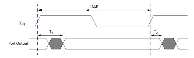
Figure 73. GPIO Port Output Timing
