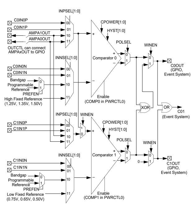
Figure 61. Comparators Block Diagram
