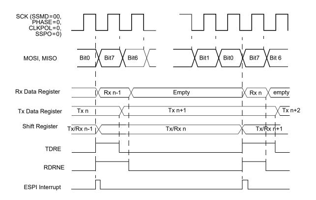
Figure 36. SPI Mode (SSMD=000)
