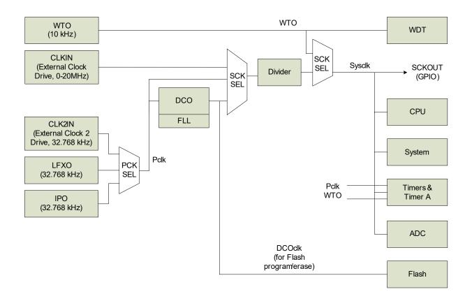
Figure 9. Clock System Block Diagram
