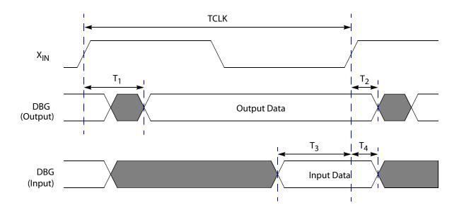
Figure 74. On-Chip Debugger Timing
