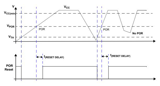
Figure 6. Power-On Reset Behavior
