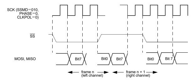
Figure 37. I<sup>2</sup>S Mode (SSMD=010), Multiple Frames
