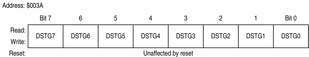
Figure 6-15. ICG DCO Stage Register (ICGDSR)
