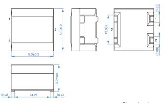
Dimensions in mm \* This product has 3 terminals. Pin 3 terminal is an dummy terminal, so open wiring is required.
