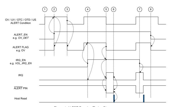
Figure 1. ALERT Function Timing Diagram
