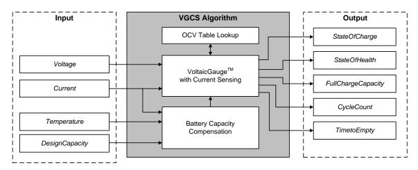
The RT9422 got battery voltage information then using OCV table and iterate calculation with current correction to calculate delta SOC, then using design capacity and battery capacity as a reference to optimize result and output final SOC result. VGCS also support high C-RATE charging technology.
