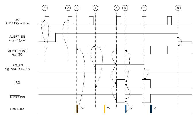
Figure 2. SC ALERT Function Timing Diagram
