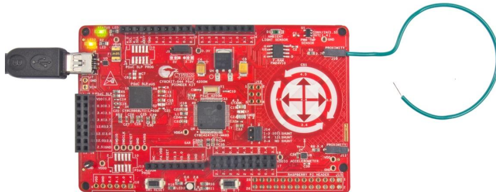
Figure 4-5. Proximity Sensor Connection on PSoC 4 M-Series Pioneer Kit
