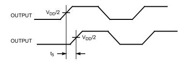
Figure 5. Input to Output Propagation Delay
