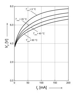
**Opt. Power / Forward Voltage** <sup>7), 8)</sup> B2:  $V_F = f(I_F)$ ;  $T_{case} = 25^{\circ}C$
