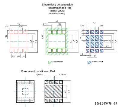
Do not use exposed copper MCPCB technology for automotive applications. For superior solder joint connectivity results we recommend soldering under standard nitrogen atmosphere. Package not suitable for any kind of wet cleaning or ultrasonic cleaning.
