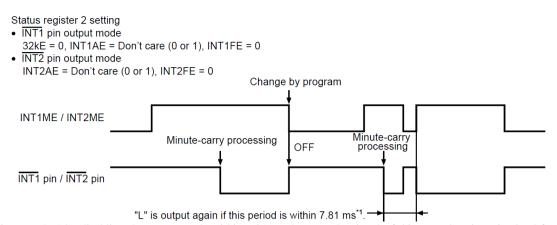
\*1. Pin output is set to "H" by disabling the output mode within 7.81 ms, because the signal of this procedure is maintained for 7.81 ms. Note that pin output is set to "L" by setting enable the output mode again.
