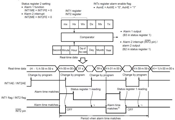
\*1. If users clear INT2AE once; "L" is not output from the INT2 pin by setting INT2AE enable again, within a period when the alarm time matches real-time data.
