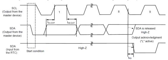
**Output Timing of Acknowledgment Signal**
