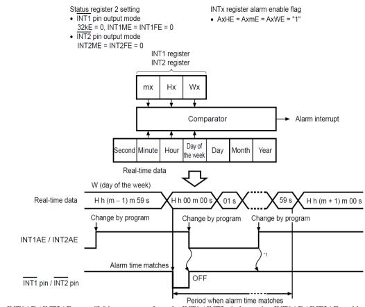
\*1. If users clear INT1AE / INT2AE once; "L" is not output from the INT1 / INT2 pin by setting INT1AE / INT2AE enable again, within a period when the alarm time matches real-time data.
