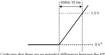
\*1. 0 V indicates that there are no potential differences between the VDD pin and VSS pin. How to Raise the Power Supply Voltage
