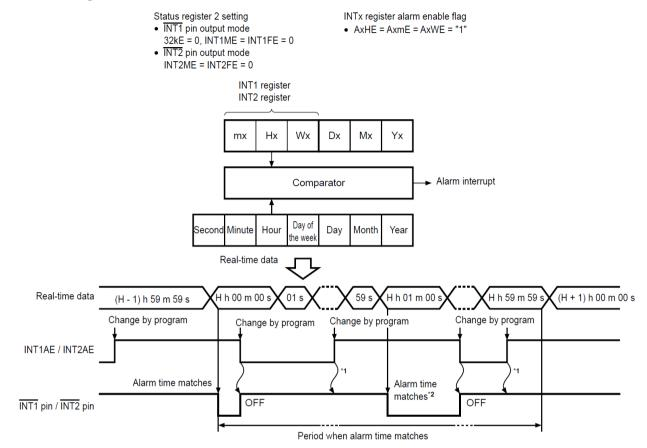
\*1. If users clear INT1AE / INT2AE once; "L" is not output from the INT1 / INT2 pin by setting INT1AE / INT2AE enable again, within a period when the alarm time matches real-time data.
