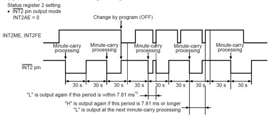
**\*1.** Setting the output mode disable makes the pin output "H", while the output from the INT2 pin is in "L". Note that pin output is set to "L" by setting enable the output mode again.
