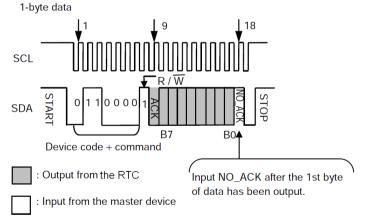
Example of Data Reading 1 (1-Byte Data Register)
