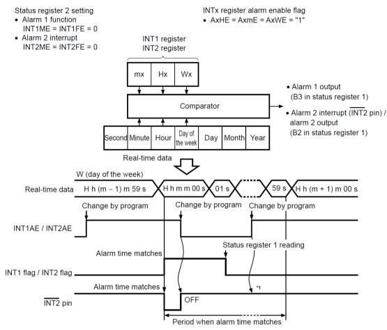
\*1. If users clear INT2AE once; "L" is not output from the INT2 pin by setting INT2AE enable again, within a period when the alarm time matches real-time data.
