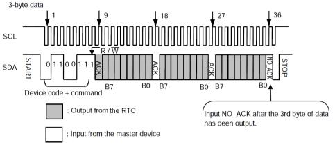
Example of Data Reading 2 (3-Byte Data Register)
