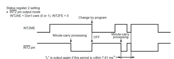
\*1. Pin output is set to "H" by disabling the output mode within 7.81 ms, because the signal of this procedure is maintained for 7.81 ms. Note that pin output is set to "L" by setting enable the output mode again.
