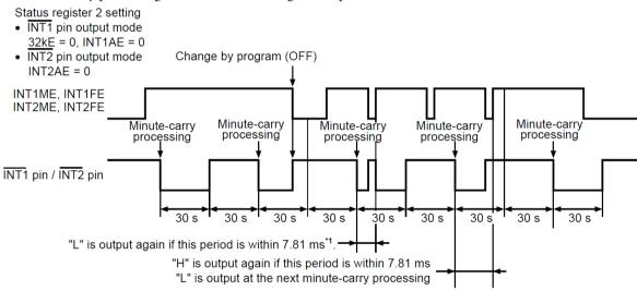
\*1. Setting the output mode disable makes the pin output "H", while the outputs from the INT1 / INT2 pin is in "L". Note that pin output is set to "L" by setting enable the output mode again.
