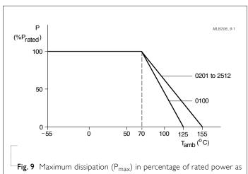
Fig. 9 Maximum dissipation (P<sub>max</sub>) in percentage of rated power as a function of the operating ambient temperature (T<sub>amb</sub>)
