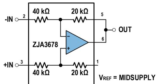
$$V_{OUT} = \frac{1}{2} (V_{IN+} - V_{IN-}) + V_{REF}$$
