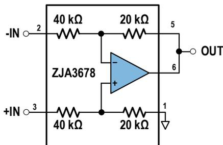
$$V_{OUT} = \frac{1}{2} (V_{IN+} - V_{IN-})$$
