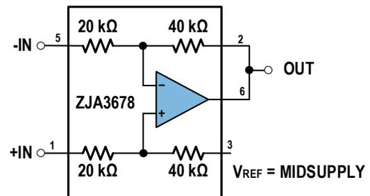
$$V_{OUT} = 2 (V_{IN+} - V_{IN-}) + V_{REF}$$
