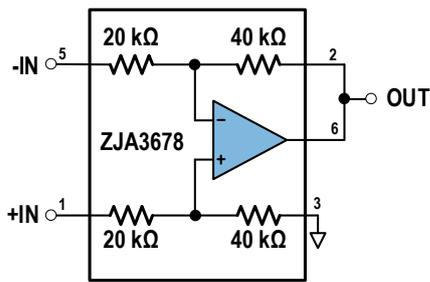
$$V_{OUT} = 2 (V_{IN+} - V_{IN-})$$
