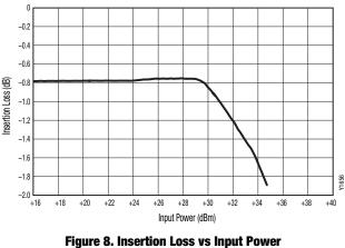
gure 8. Insertion Loss vs input Pow @ 3.6 GHz, V1 = 5 V
