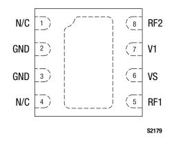
Figure 2. SKY13347-360LF Pinout (Top View)
