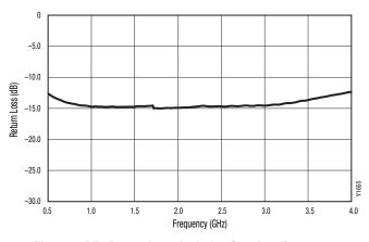
Figure 6. RF2 Return Loss (Isolation State) vs Frequency
