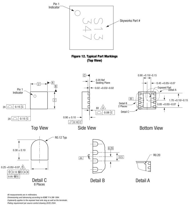
Dimension applies to metalized terminal and is measured between 0.15 mm and 0.30 mm from terminal tip.
