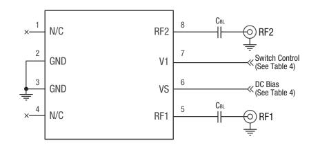
Note: CBL = 47 pF for >500 MHz operation; 220 pF for operation down to 50 MHz. Higher values recommended for lower frequency operation. Exposed paddle must be grounded.
