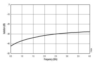
**Figure 5. Isolation vs Frequency**
