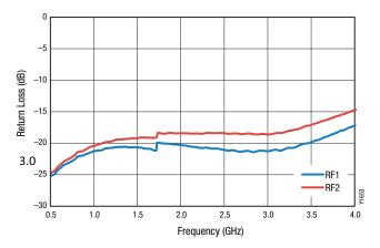
Figure 4.Return Loss (Insertion Loss State) vs Frequency
