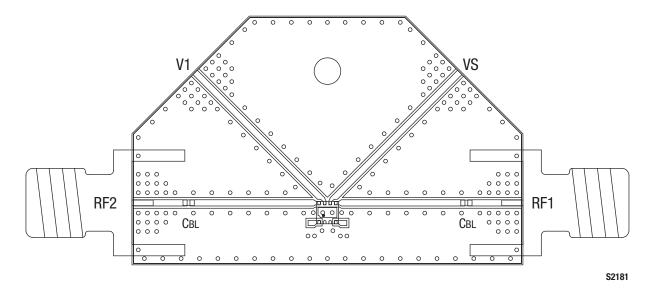
Figure 10. SKY13347-360LF Evaluation Board Assembly Diagram
