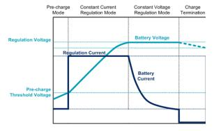
Figure 24: Pre-Charge and Charge Voltage/Current
