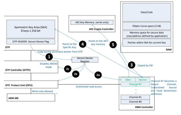
Figure 10: Symmetric Keys manipulation
