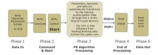
Figure 57: ECC programming flow
