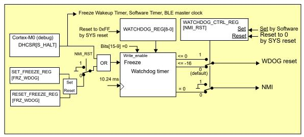
Figure 109: Watchdog Timer block diagram
