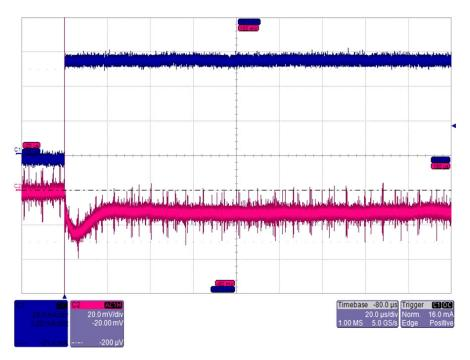
Figure 20: LDO\_IO loadstep 0 to 60mA (Cload=10uF)
