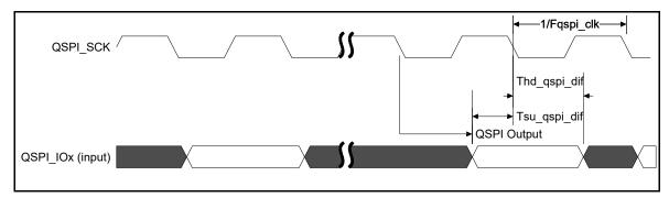
Figure 48: QSPI Input Timing
