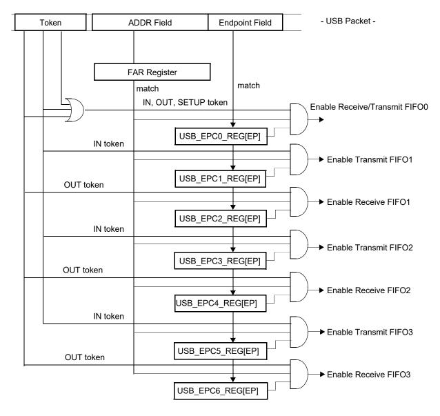
Figure 113: USB Function Address/Endpoint Decoding
