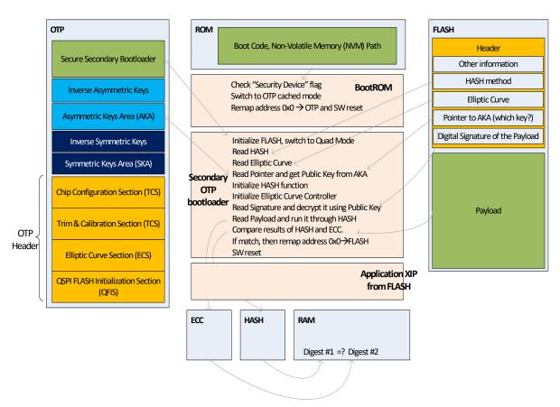
Figure 11: CPU steps for a Secure Boot process
