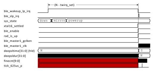
Figure 125: Exit BLE Deep Sleep Mode at predetermined time (zoom out)
