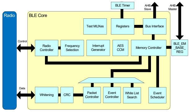
Figure 121: BLE Core Block Diagram
