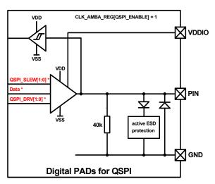
Figure 120: Latching of QSPI pad signals
