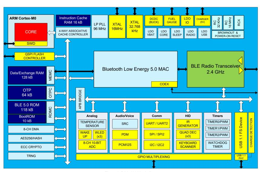
Figure 1: DA14683 block diagram
