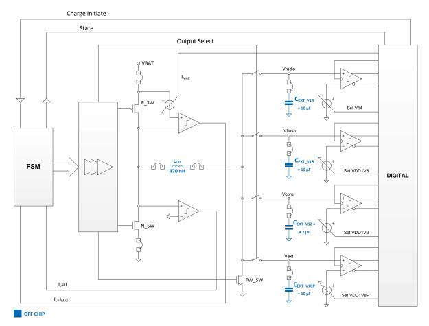
Figure 13: SIMO DCDC Converter block diagram
