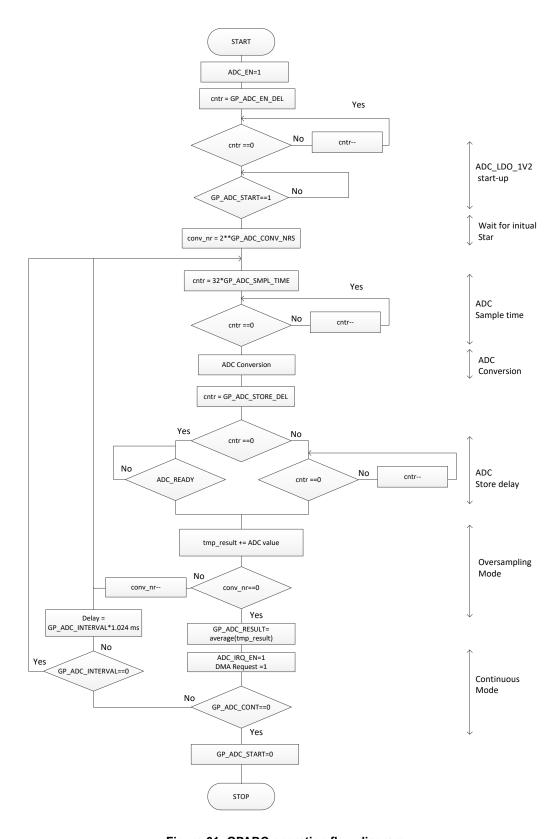
Figure 61: GPADC operation flow diagram
