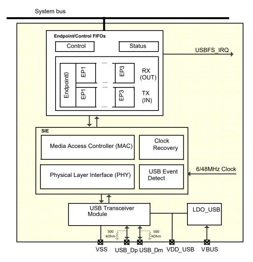
Figure 110: USB Node block diagram
