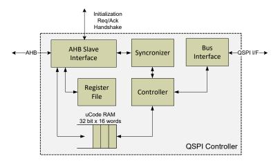
Figure 46: Quad SPI Controller architecture
