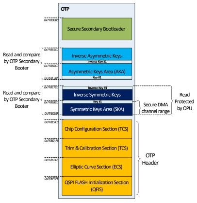
Figure 9: OTP layout with security features enabled
