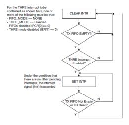
Figure 78: Flowchart of Interrupt generation when not in Programmable THRE Interrupt Mode
