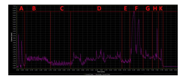
Figure 129: BLE Connection power profile
