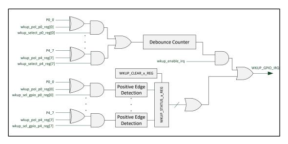
Figure 59: Wakeup Timer block diagram
