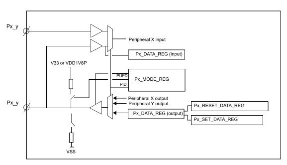
Figure 118: Port P0, P1, P2, P3 and P4 with Programmable Pin Assignment
