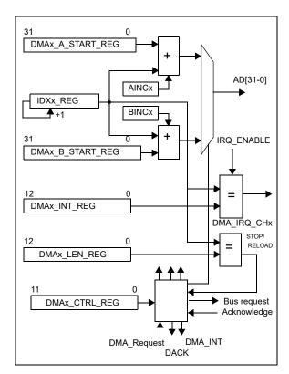
Figure 51: DMA channel diagram
