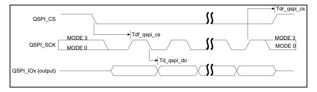
Figure 49: QSPI output Timing
