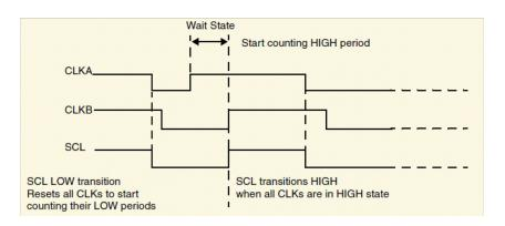
Figure 95: Multiple Master Clock synchronization.
