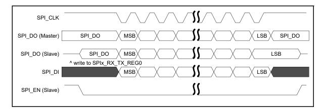
Figure 83: SPI Master/slave, mode 3: SPI\_POL=1 and SPI\_PHA=1
