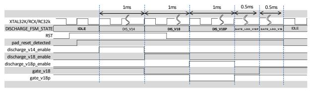
Figure 32: Discharging rails FSM timing
