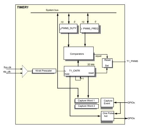
Figure 106: Timer 1 block diagram
