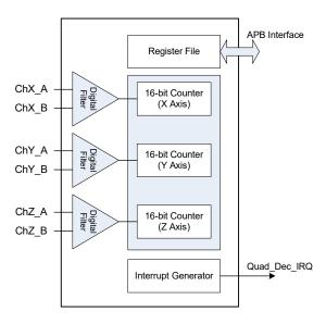
Figure 98: Block diagram of the Quadrature Decoder
