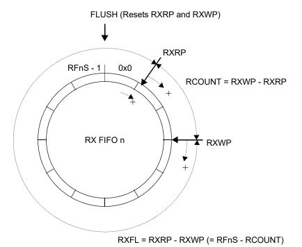
Figure 116: Rx FIFO operation
