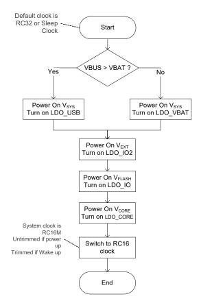
Figure 4: Power Up / Wake Up FSM
