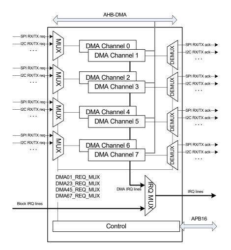
Figure 50: DMA controller block diagram
