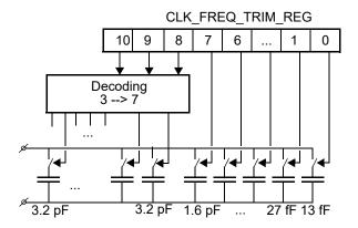
Figure 36: Frequency trimming
