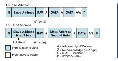
Figure 91: Master-Transmitter Protocol
