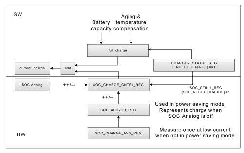
Figure 28: Fuel Gauge operation
