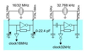
Figure 35: Crystal oscillator circuits
