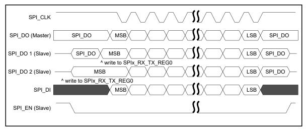
Figure 82: SPI Master/Slave, mode 2: SPI\_POL=1 and SPI\_PHA=0
