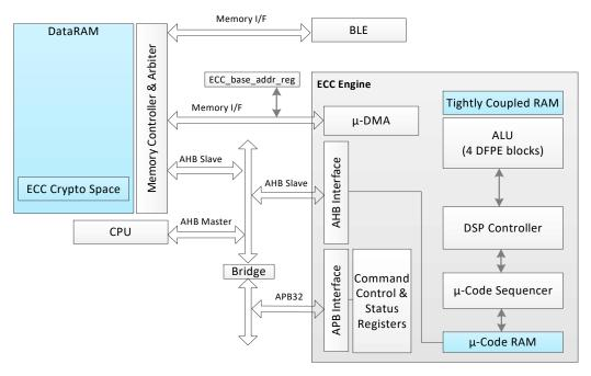
Figure 56: ECC Engine Block Diagram
