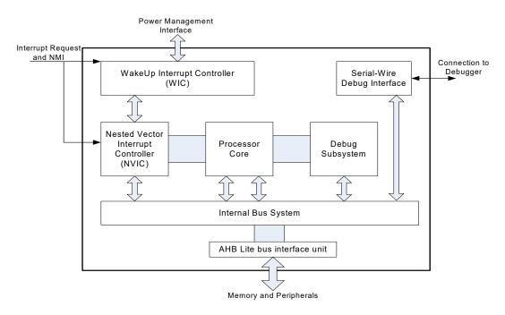
Figure 38: Arm Cortex-M0 Block Diagram
