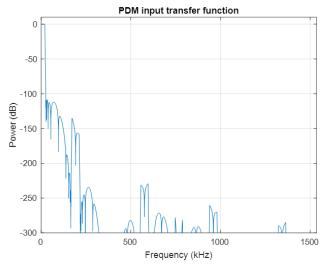
Figure 65: SRC PDM input transfer function
