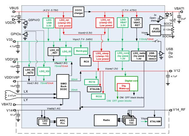
Figure 12: Power management unit block diagram
