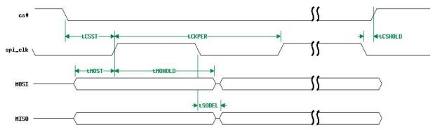
Figure 84: SPI slave mode timing (CPOL=0, CPHA=0)
