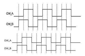
Figure 100: Moving backwards on axis X
