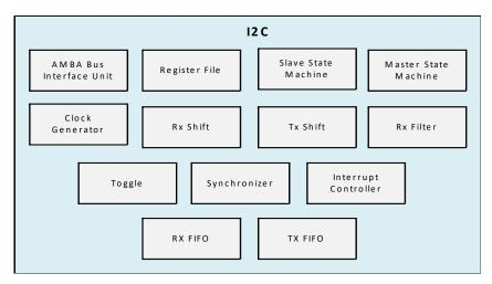
Figure 85: I2C Block diagram
