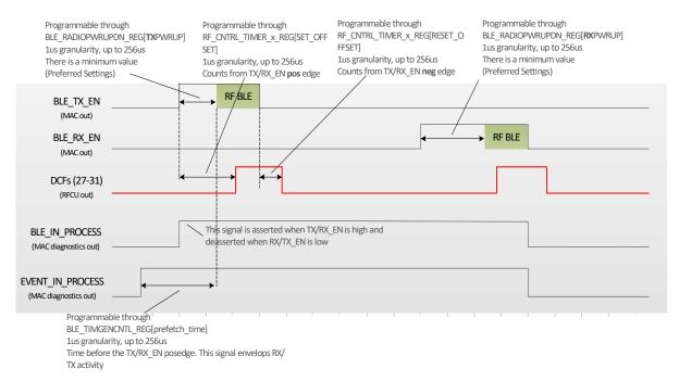
Figure 133: DCF signals programming
