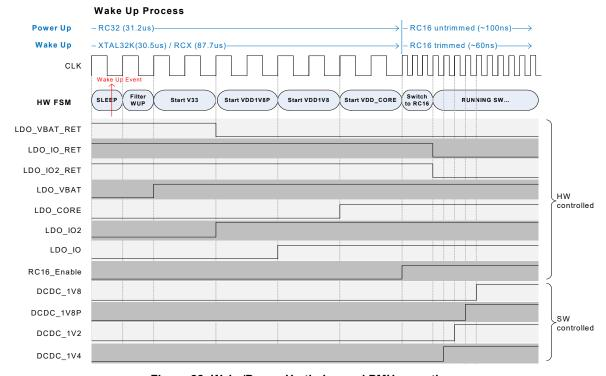
Figure 22: Wake/Power-Up timing and PMU operations
