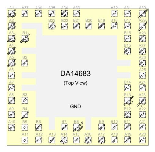
Figure 2: AQFN60 pin assignment
