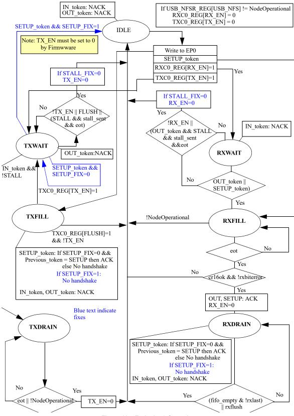
Figure 114: Endpoint 0 Operation
