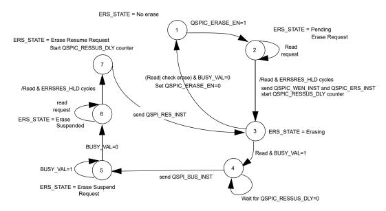
Figure 47: Erase Suspend/Resume in Auto mode
