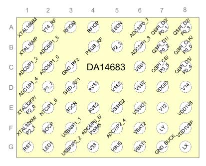
Figure 3: WLCSP53 ball assignment
