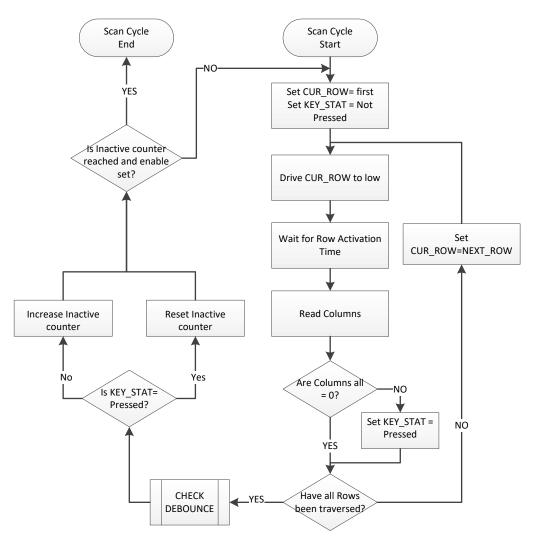
Figure 103: Scan cycle state machine
