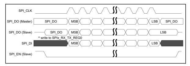
Figure 81: SPI Master/Slave, mode 1: SPI\_POL=0 and SPI\_PHA=1
