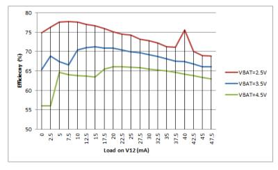
Figure 15: 1.2V rail DCDC efficiency vs load
