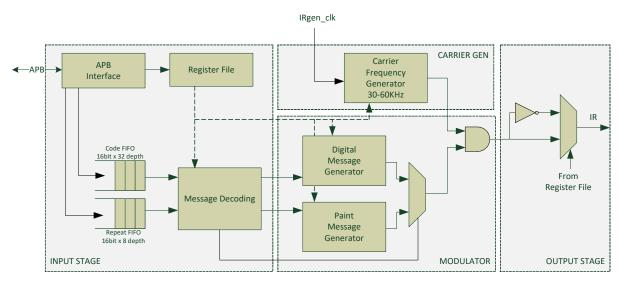
Figure 96: InfraRed Generator Block Diagram
