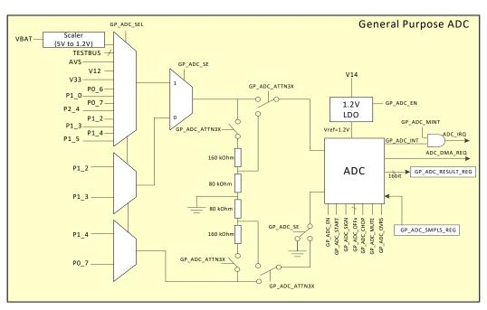
Figure 60: Block diagram of the General Purpose ADC
