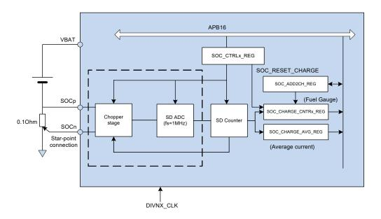
Figure 27: State of charge (SOC) circuit block diagram
