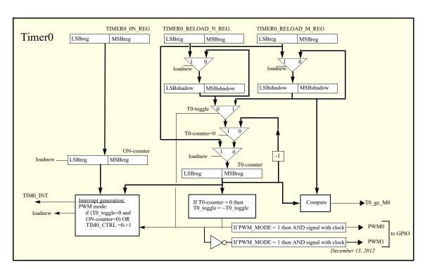
Figure 104: Timer0 block diagram
