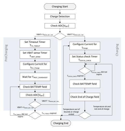
Figure 25: Pre-Charge and Charge SW FSM
