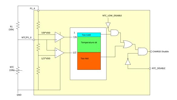
Figure 26: Charger auto shut-off circuit
