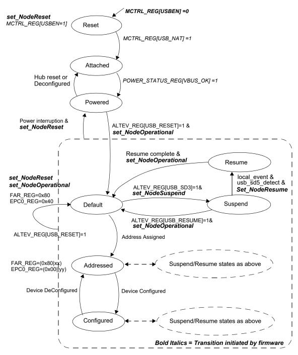
Figure 112: Node Functional State Diagram
