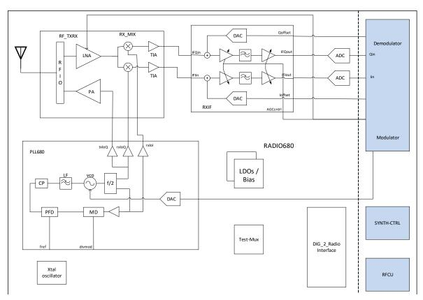
Figure 132: Radio Block Diagram
