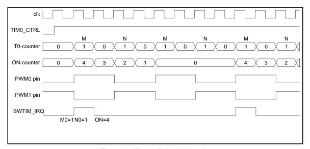
Figure 105: Timer 0 Pulse PWM mode
