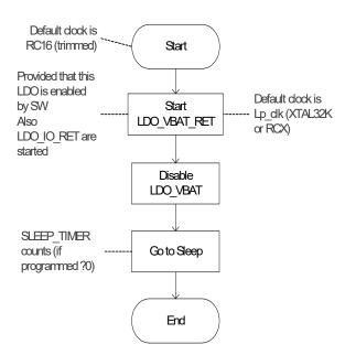
Figure 5: Go to Sleep FSM flow diagram
