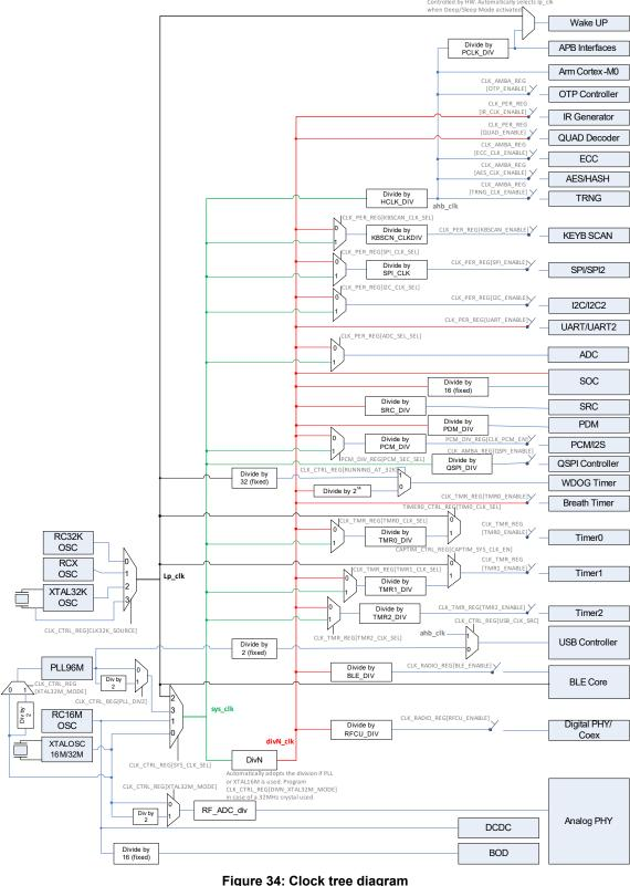
Figure 34: Clock tree diagram
