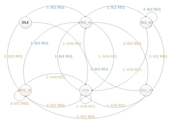
Figure 43: Memory controller's arbitration scheme
