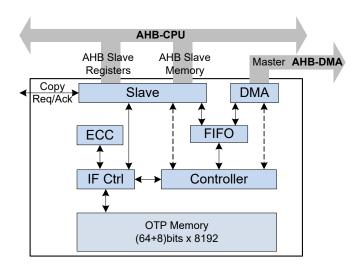
Figure 44: OTP Controller block diagram
