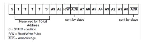
Figure 90: 10-bit Address Format
