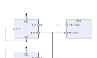
Figure 63: PDM with dual mic interface
