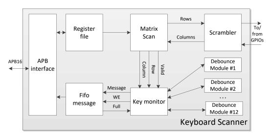
Figure 101: Keyboard Scanner block diagram
