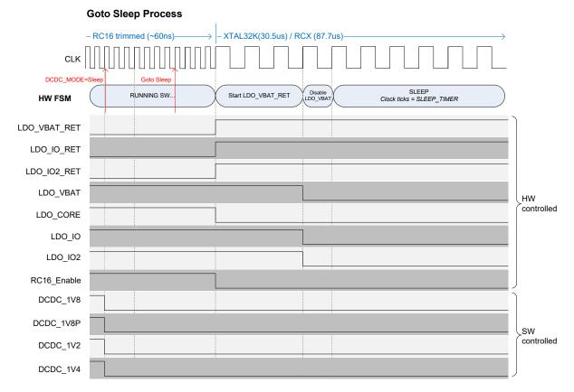
Figure 23: Goto Sleep timing and PMU operations
