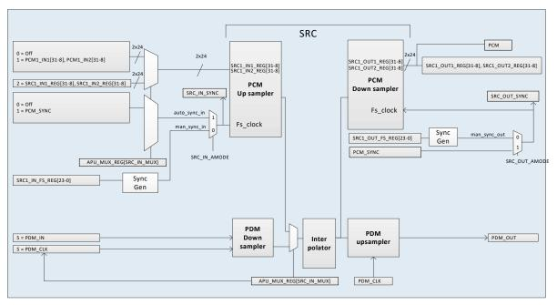
Figure 62: Sample rate Converter block diagram
