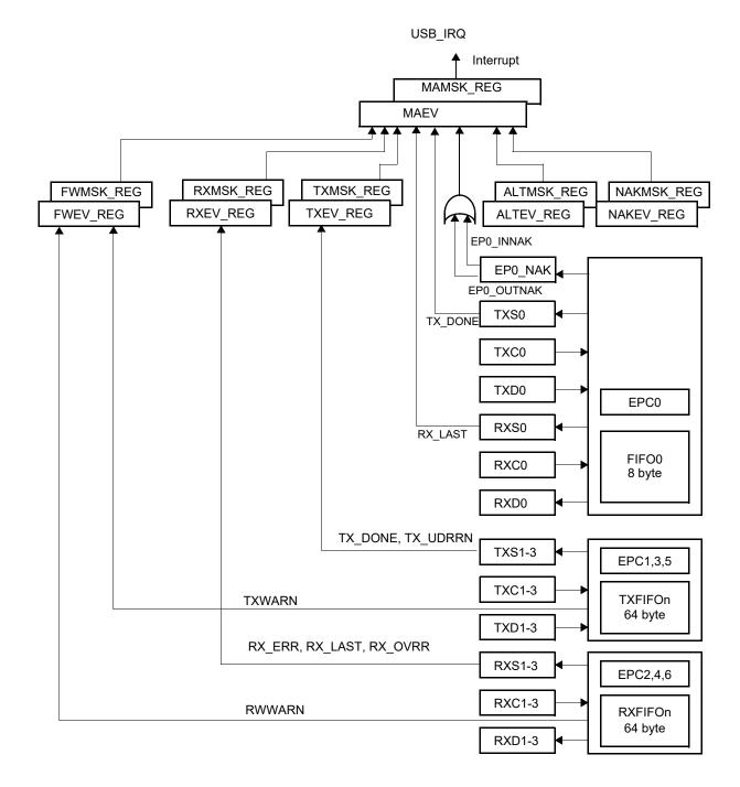
Figure 117: Interrupt Register hierarchy
