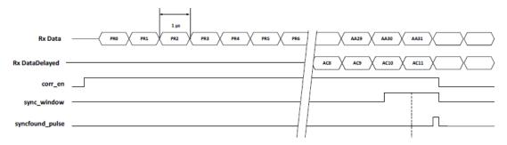
Figure 127: Diagnostics signals timing during correlation
