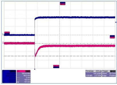
Figure 17: LDO\_VBAT loadstep 0 to 100mA (Cload=4.7uF, Vout=3.3V)
