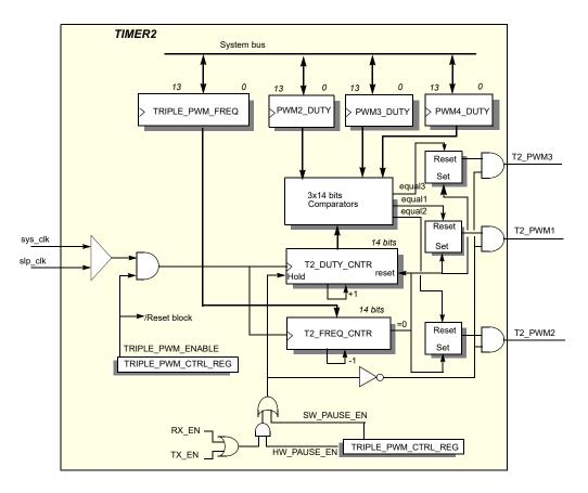
Figure 107: PWM Timer 2 block diagram
