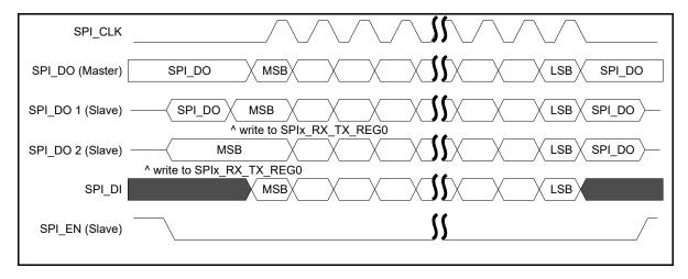
Figure 80: SPI Master/slave, mode 0: SPI\_POL=0 and SPI\_PHA=0
