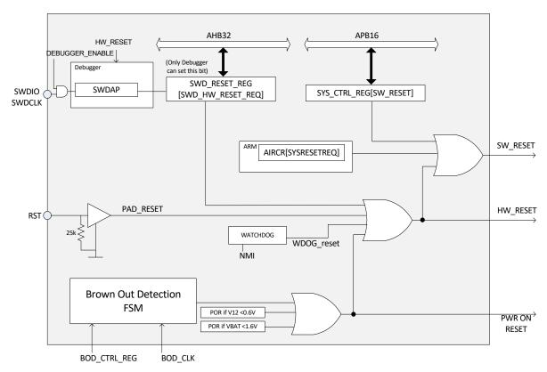
Figure 30: Reset and Brown-Out block diagram
