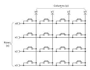
Figure 102: 4x4 Keyboard Matrix example
