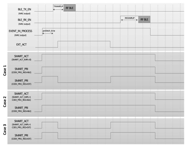
Figure 131: Coexistence signalling cases
