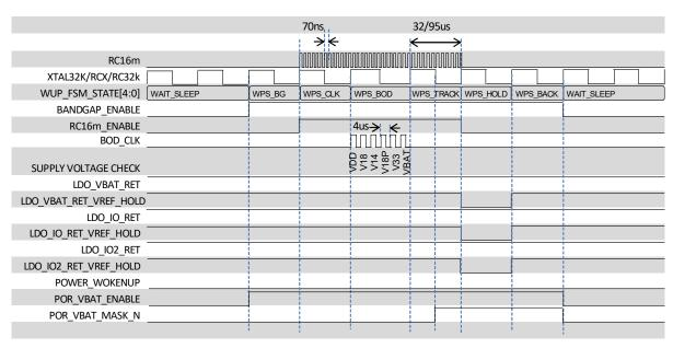
Figure 33: SLEEP TIMER based wake up timing for BOD
