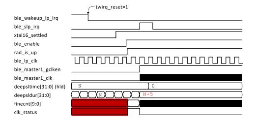
Figure 124: Exit BLE Deep Sleep Mode later than the predetermined time (zoom in)
