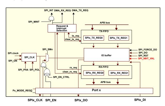
Figure 79: SPI block diagram
