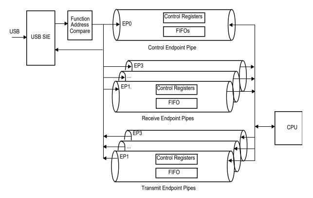
Figure 111: Endpoint Operation
