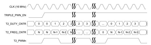
Figure 108: Timer 2 PWM timing diagram
