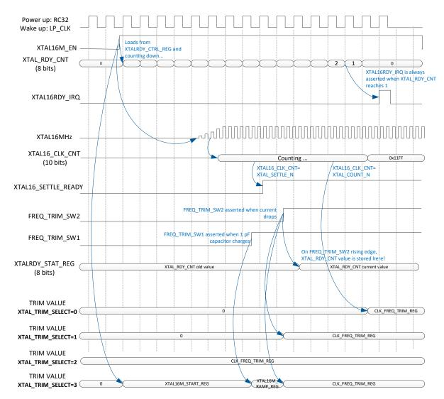
Figure 37: Automated mechanism for XTAL16M trim and settling
