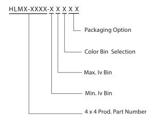
To order Subminiature Lamps packaged with these standard options, include the appropriate option code along with the device catalog part number.
