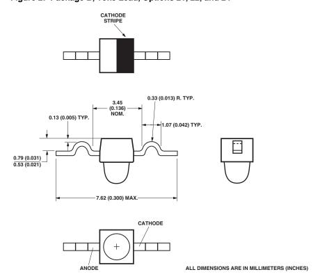
Figure 3: Package C, Z-Bend Lead, Option 31, 32, and 34
