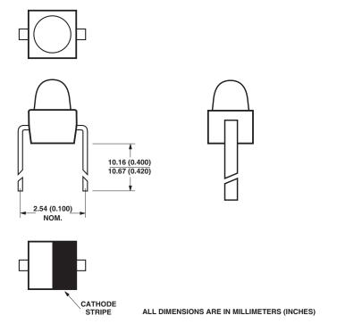
Figure 5: Package E, Right-Angle Bend Option 1S
