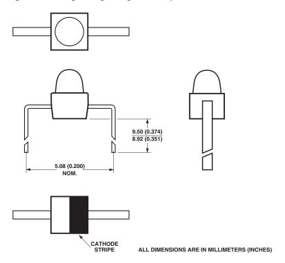
Figure 7: Package G, Right-Angle Bend Option 2S
