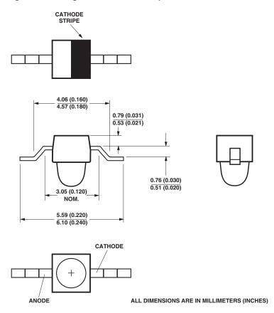
Figure 4: Package D, Right-Angle Bend, Option 1L
