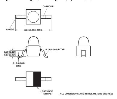
Figure 2: Package B, Yoke Lead, Options 21, 22, and 24
