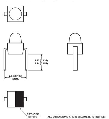
Figure 6: Package F, Right-Angle Bend Option 2L
