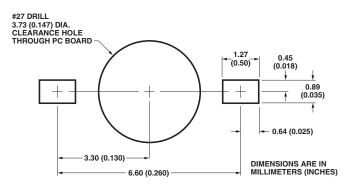
Figure 16: Recommended Soldering Pad Pattern for Z-Bend Leads 31, 32, and 34
