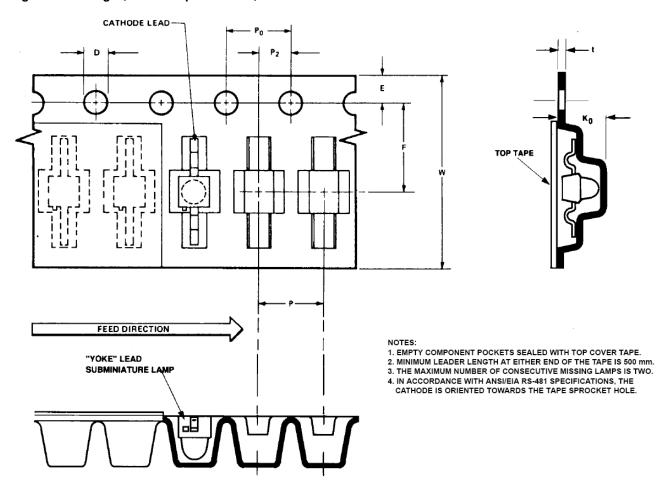
Figure 10: Package J, 12-mm Tape-and-Reel, Z-Bend Lead
