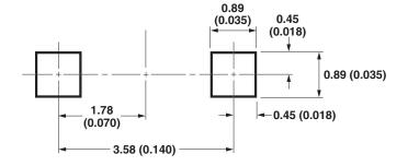
Figure 15: Recommended Soldering Pad Pattern for Yoke Leads 21, 22, and 24
