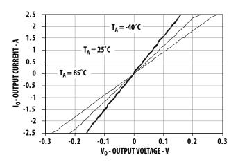
Figure 11: Typical R<sub>(ON)</sub> (DC Connection) vs. Temperature
