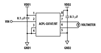
Figure 10: Input Offset vs. Supply Voltage
