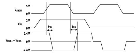
Figure 27: Propagation Delay Diagram
