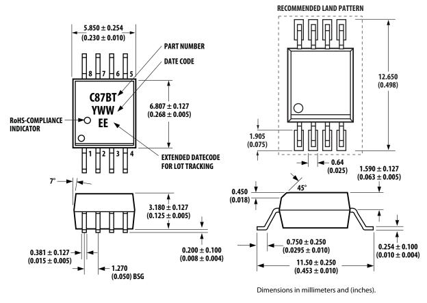
Lead coplanarity = 0.1 mm (0.004 inches). Floating lead protrusion = 0.25mm (10mils) max.
