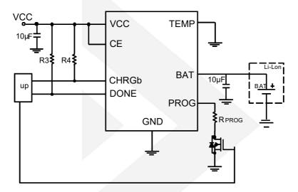
Figure 5. Manual Shutdown Mode Application Circuit
