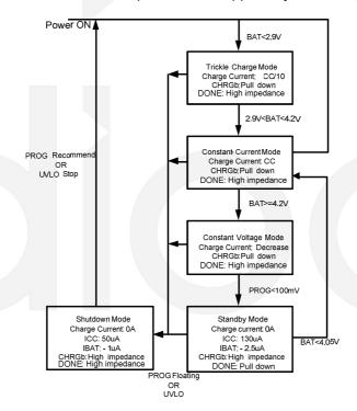
Figure 4. State Diagram of a Typical Charge Cycle
