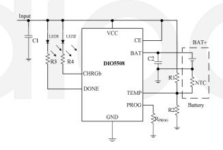
**Figure 1 Typical Application Circuit**
