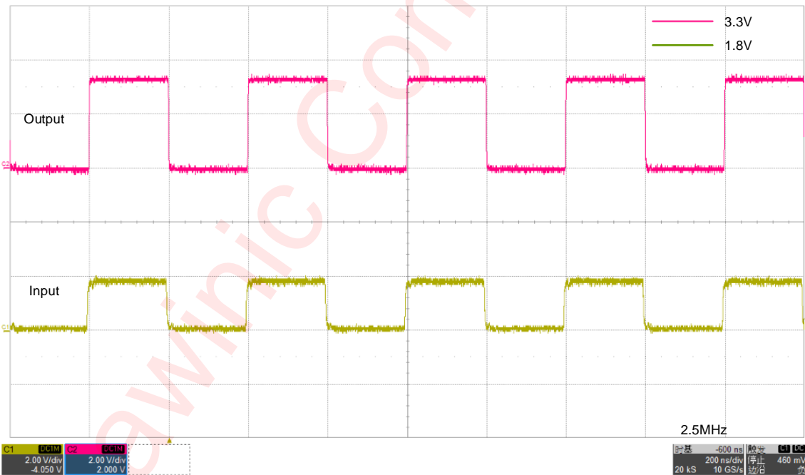
2.5-MHz 1.8V-3.3V Signal Level-Translation @ C_L=30p
