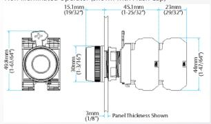
Illuminated Full Voltage and Multi-Voltage Dual Push Button Operators (shown with 1 Flush Cap and 1 Extended Cap)
