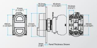
2-Position Push-Twist Release Maintained Non-Illuminated Operator (shown with 40mm [1-9/16"] Mushroom Cap)
