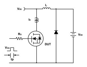
Figure C. Unclamped Inductive Switching Circuit & Waveforms
