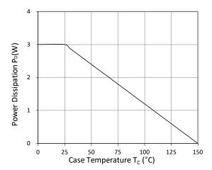
Figure 9. Power Dissipation
