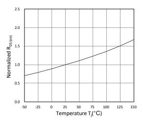
Figure 6. Normalized  $R_{DS(on)}$  vs. Temperature
