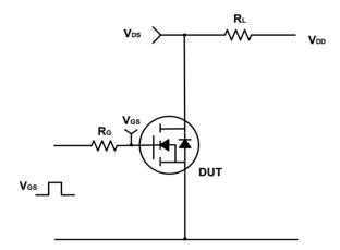
Figure B. Switching Test Circuit & Waveforms
