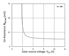
Figure 4.  $R_{DS(ON)}$  vs.  $V_{GS}$
