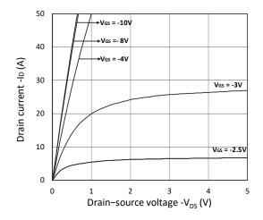
Figure 1. Output Characteristics
