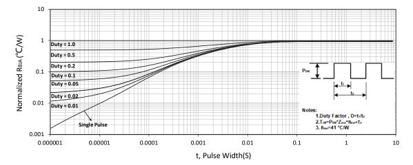
Figure 11. Normalized Maximum Transient Thermal Impedance
