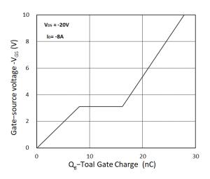
Figure 8. Gate Charge Characteristics
