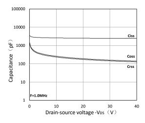
Figure 7. Capacitance Characteristics
