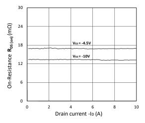
Figure 5.  $R_{DS(ON)}$  vs.  $I_D$
