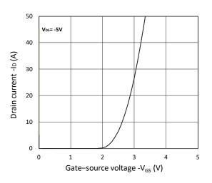
Figure 2. Transfer Characteristics
