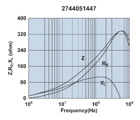
Impedance, reactance, and resistance vs. frequency.
