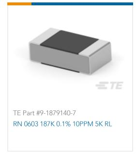
200K  $\Omega$ , Thin Film, Precision Resistor, .1 %, 2 Termination, 0603, Taped & Reeled, .063 W,  $\pm 10$  ppm/°C, Solder, Height .018 in [.45 mm], Holsworthy RN73
