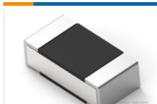
TE Part #1-2176308-8 RP 1E 0.1W 200K 0.1% 25PPM 5K RL
