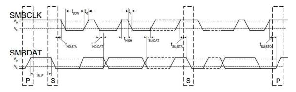
Figure 6-9. SMBus Slave Time Diagram
