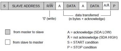
Figure 7-1 Write transfer format
