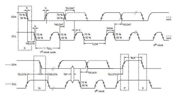
Figure 7-4 Definition of timing on the I2C bus
