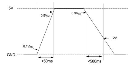
Figure 5-2 Power On/Off Sequence in 5V only mode
