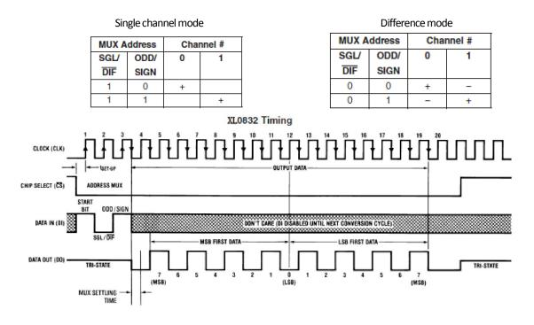
When 2-bit data is set to 1 or 0, only the CH0 is converted in single channel.
