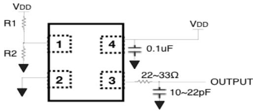
Non-modulated clock output when R1=NC and, R2=0 ohm
