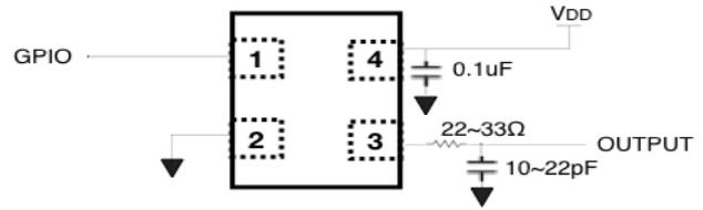
Non-modulated clock output when GPIO=Low
