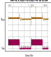
Short-Circuit Response V<sub>IN</sub>=24V,V<sub>OUT</sub>=5V,I<sub>OUT</sub>=0A to Short
