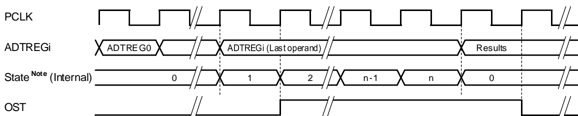
Figure 27-39. Timing Diagram of Sequence Operation (ACTCLREG.STM = 0 case)
