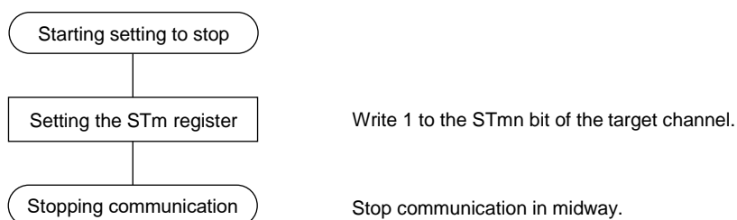
Figure 15-37. Procedure for Stopping Master Reception
