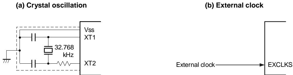
Figure 5-22. Example of External Circuit of XT1 Oscillator
