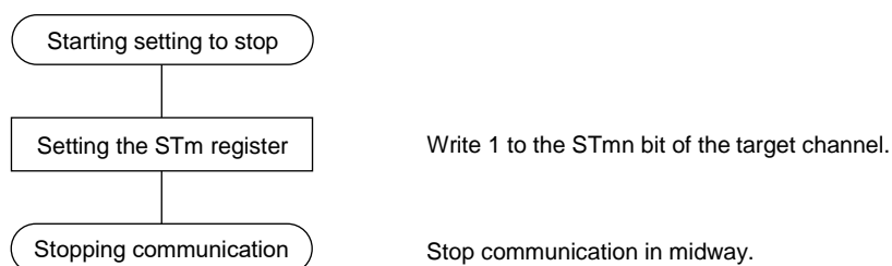
Figure 15-37. Procedure for Stopping Master Reception
