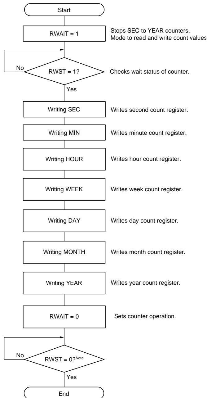
Figure 9-24. Procedure for Writing Real-time Clock
