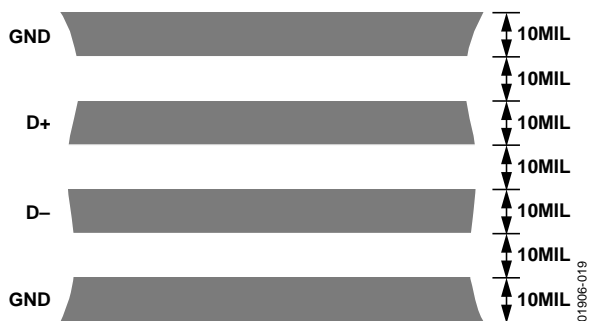
Figure 19. Arrangement of Signal Tracks
