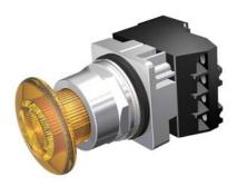
30mm Command/52, Chrome Finish Heavy Duty, Watertight/Oiltight Complete Metal Unit Illuminated Push-Pull Operator Full Voltage, 24V AC/DC Incandescent Lamp Mushroom Head Cap Small 1 3/4" (44.5 mm) Plastic, Amber 2 Position Maintained, Pull-to-Release with 1 N.O. - 1 N.C. Heavy Duty Contacts, A600/P600 UL Listed, CSA Certified NEMA 1,3,3R,4,4X,12,13 & Automotive Standards
