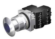
30mm Command/52, Chrome Finish Heavy Duty, Watertight/Oiltight Complete Metal Unit Illuminated Push-Pull Operator Transformer type, 480V AC LED Lamp Mushroom Head Cap Small 1 3/4" (44.5 mm) Metal, Chrome with Blue Lens 3 Position Pull-Momentary/Push-Maintained 1 N.C.+1 N.C. Extra Late Break Heavy Duty Contacts, A600/P600 UL Listed, CSA Certified NEMA 1,3,3R,4,4X,12,13 & Automotive Standards
