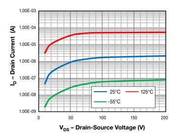
Figure 2. Typical Drain-Source Leakage Current vs. Ambient Temperature
