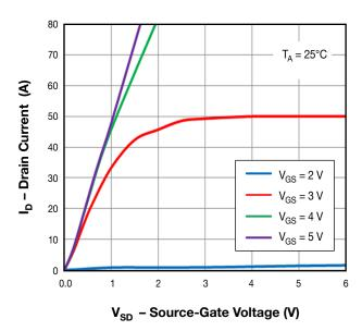
Figure 4. Typical Gate-Drain Transfer Characteristic
