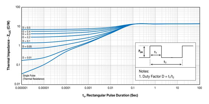
Figure 13. Transient Thermal Impedance, Junction to Case
