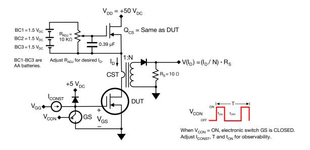
Figure 14. Charge Test Circuit
