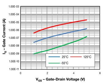
Figure 3. Gate-Source Leakage Current vs. Ambient Temperature
