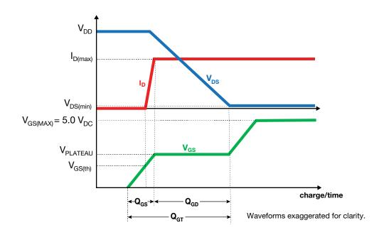
Figure 15. Typical Gate Charge Test Waveform
