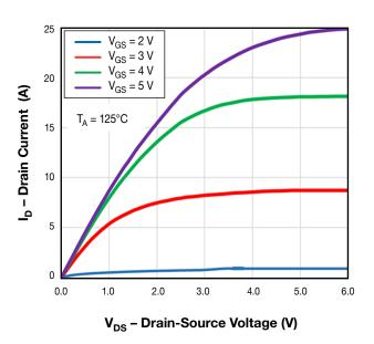
Figure 5. Typical Output Characteristics
