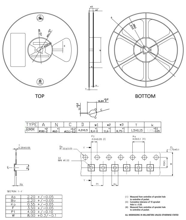
Figure 8: 8TR2211 Tape and Reel Dimension
