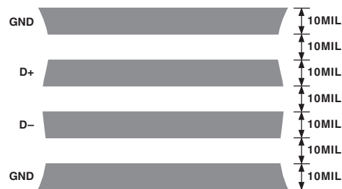
Figure 4. Arrangement of Signal Tracks
